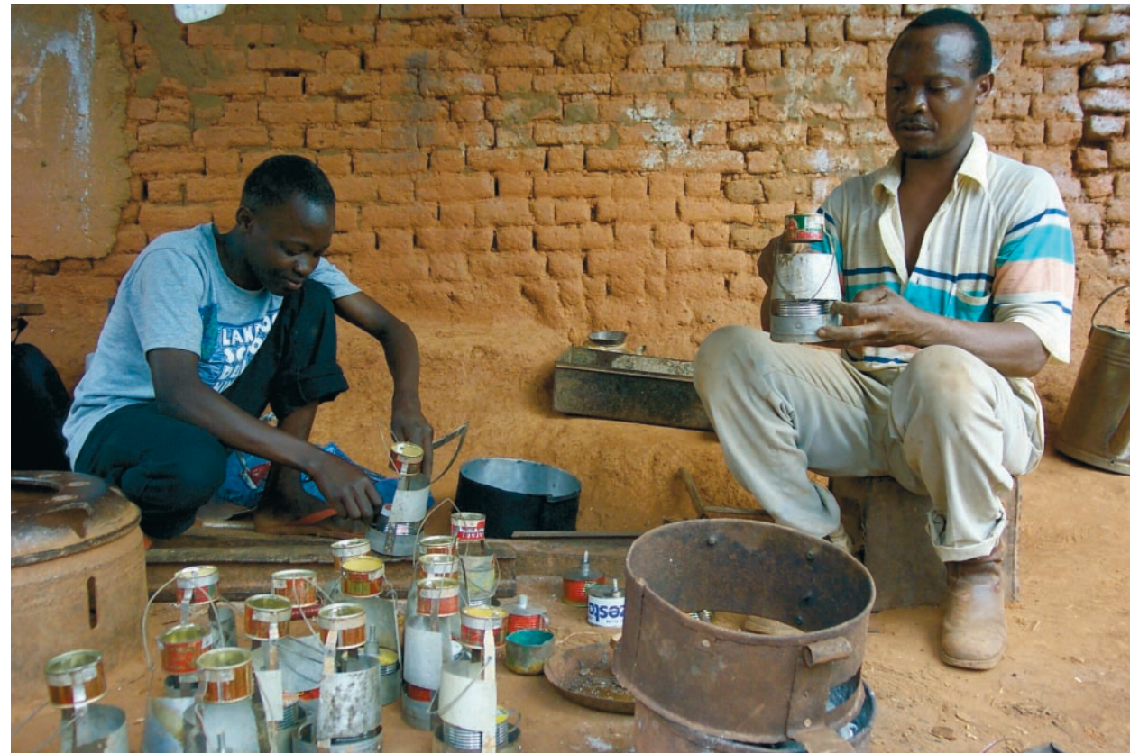
Local koroboi -maker assembling the repellent lamp from recycled tin cans and bits of wire. Photo: Hans Jemet
