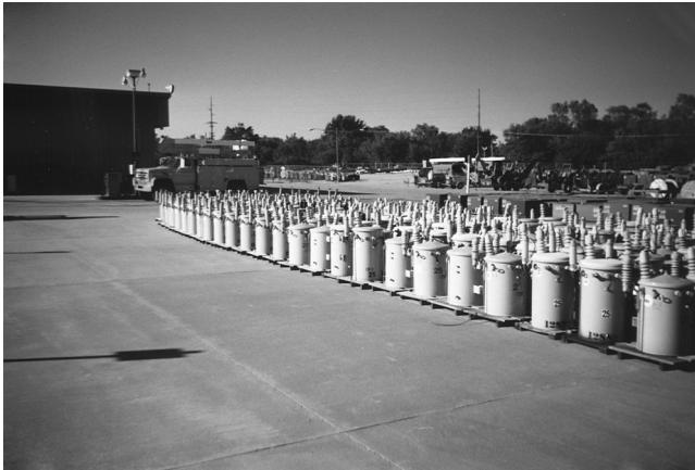
FIGURE 15.1 Electric utility distribution storage yard. Forklift trucks are used to load transformers on line trucks. Storage area is covered with concrete to provide accessibility and protect transformers.
