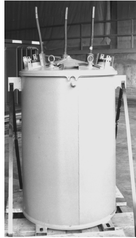
FIGURE 15.6 Submersible distribution transformer strapped to a pallet for shipment. Cables are for low-voltage connections. High-voltage connections are made with elbow cable connectors to bushing inserts installed in wells shown on top of the transformer. (Courtesy ABB Power T&D Company Inc.)
