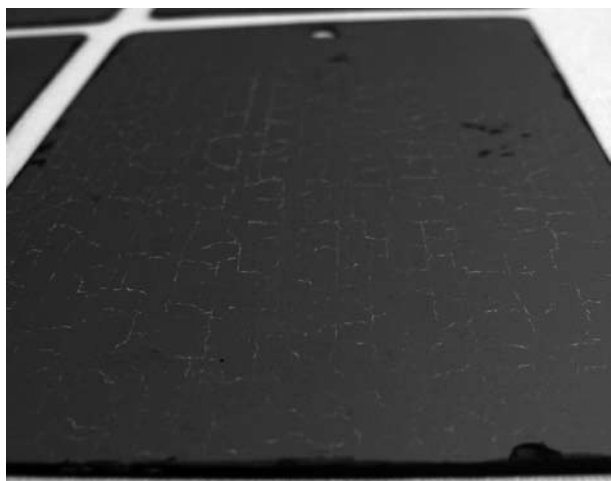
Figure 4: Tromm III wax crazed and cracked on drying revealing the metal substrate
