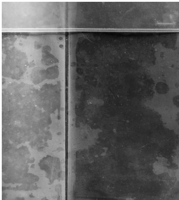
Figure 3: Plasticised PVC photograph pocket from 1980s showing liquid plasticiser which has migrated from the PVC polymer and will contaminate any enclosed materials
