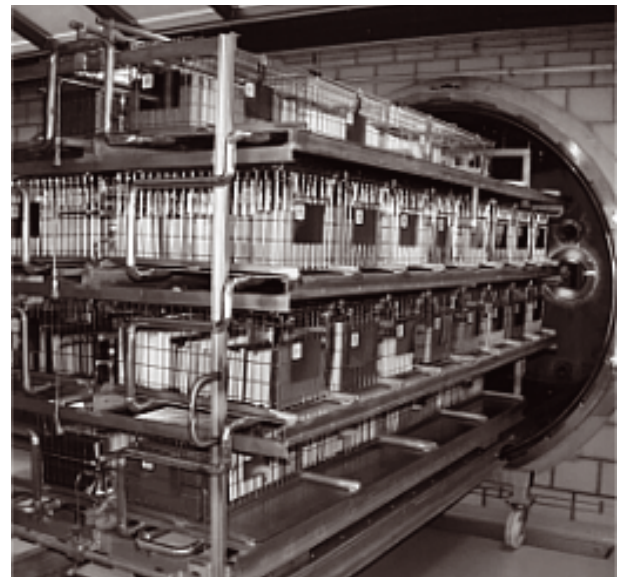
Fig. 7. In the PaperSave mass deacidification treatment there is no agitation but the batch is going into a deacidification chamber with a solution of magnesium titanium alkoxide and hexamethyldisiloxane.
