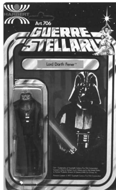
Figure 4: Star Wars figures are made from plasticised PVC and are highly collectible. Darth Vader has remained in his original packaging with the result that the migrating plasticiser has hydrolysed in the acid environment. White crystals of phthalic anhydride are visible on his once-black head
