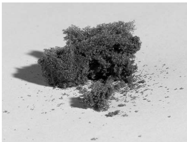
Figure 5: Photo-oxidation of polyurethane ether foam frequently results in loss of structure and crumbling
