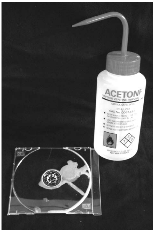
Figure 7: Environmental Stress Cracking (ESC) can be induced by cleaning a rigid plastic such as with a low boiling point solvent. The polystyrene jewel case shown here has been treated with acetone
