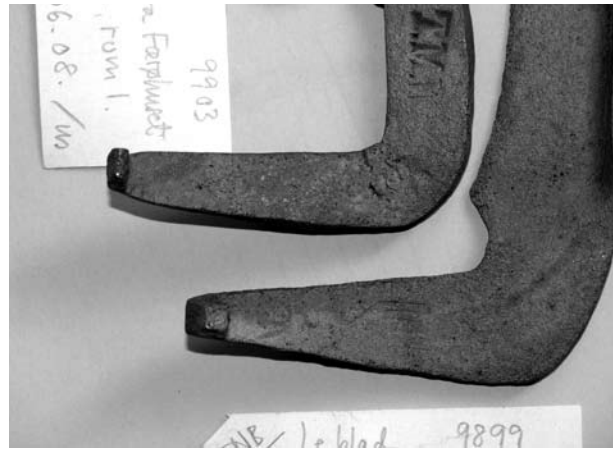
Fig. 3 Details as fabrication marks on the iron should be well documented before coating with several layers of paint. Two end parts of scythe blades are shown. Good documentation and/or sampling is also need if objects have to be stripped of remains of original paint layers.
