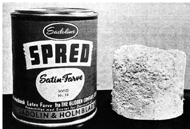
Figure 1. The content of solid binder, in this jar of styrene-butadiene paint from the 1950s, is shown next to the jar. It is obvious why the binder determines most of the paint's characteristics.
