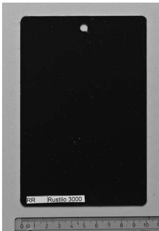
Figure 2: Rustillo 3000 is an anticorrosive coating which formed a black, opaque film on drying
