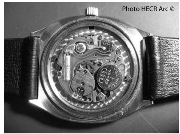
Figure 2. Girard-Perregaux quartz movement (1978 or 1979). Only the battery support and the printed circuit are made of plastic.
