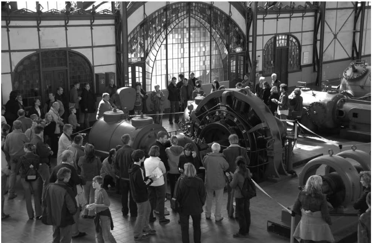
Fig 11: 1902 air compressor; “retro-fitted” by museum restorers and retired craftsmen, during a demonstration run for visitors (N. Tempel, LWL-Industriemuseum, Dortmund, 2007)
