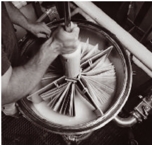
Fig. 6. The Bookkeeper mass deacidification treatment takes place in cylinders with a dispersion of perfluorocarbon and magnesium oxide.
