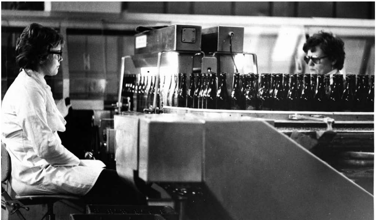
"Clearing ladies, approx. 1970. Detecting deformations in the glass was extremely demanding and the ladies staring at the bottles needed more brakes than their colleagues"
