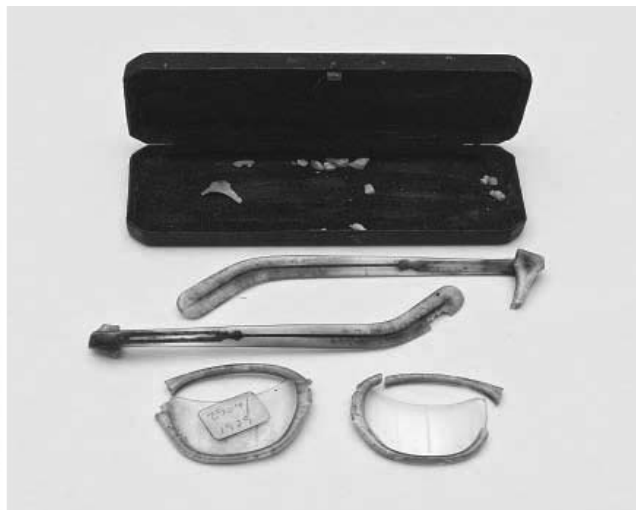
Figure 1: The frames of these cellulose nitrate spectacles made in the 1960s, began to show degradation by crazing and by the plastic's ability to corrode copper ear wires and screws in the frame in the 1980s (left of image). By 1995, degradation had progressed so dramatically that the spectacles could no longer function and were hardly recognizable as a cohesive object (right of image). They were therefore deaccessioned by the National Museum of Denmark
