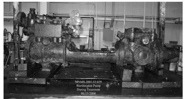
Figure 2: Starboard Worthington pump during deconcretion. Note the patent date of April 3, 1849 on the side of the cast iron cradle.
