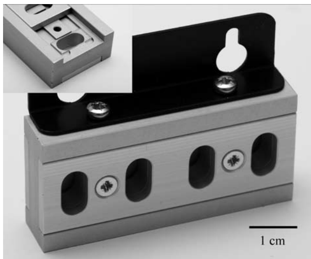
Figure 1: The EWO dosimeter holder with the PPO polymer covered glass sensor chip (inset).
