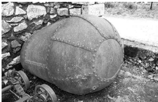
Figure 1. Cornish boiler in the East Pool and Agar Mine (Paul Bonington)
