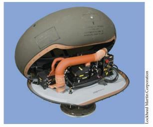
Clockwise from above: An MQ-1C Gray Eagle unmanned aircraft system (UAS) transmits images and sensor data for up to 24 hours at altitudes up to 25,000 feet; a Longbow UTA allows the crew of an AH-64D Apache to control a UAS while both are in flight; an AH-64 Apache departs Bagram Airfield, Afghanistan.
