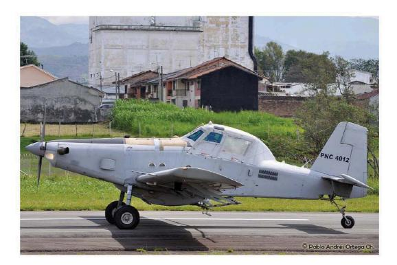
Figure 2.8. Photograph of AT-802 Spray Plane<sup>225</sup>
