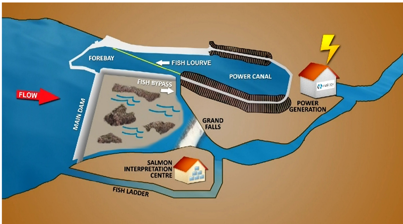
Figure 2.6 Overview of the Grand Falls Generating Station and Associated Fish Conveyance Systems
