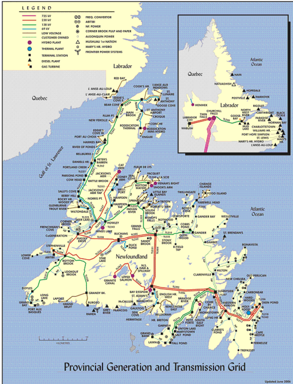
Figure 1.3 Existing Newfoundland and Labrador Generation and Transmission System
