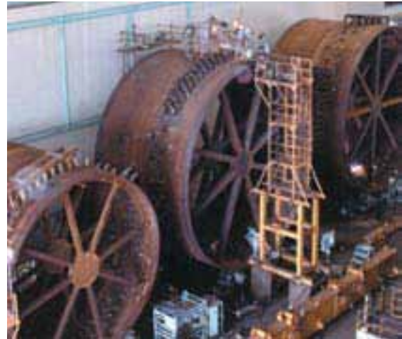
SAS reactors being fabricated in Japan
