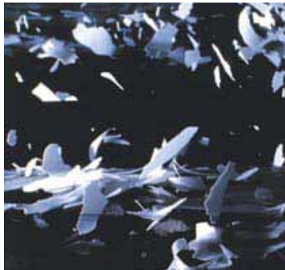
Fischer-Tropsch hard wax flakes from the low-temperature reactor at Sasolburg
