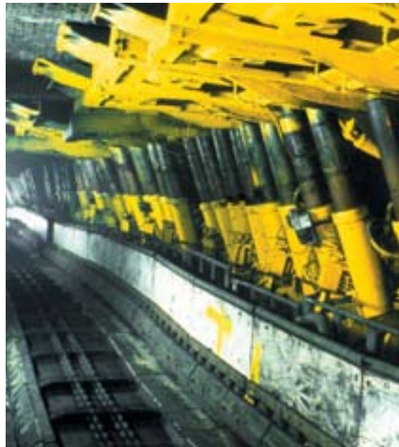
Sasol experimented with long-wall mining methods from 1967 to 1980. Shown here are hydraulic shield supports in a long-wall section
