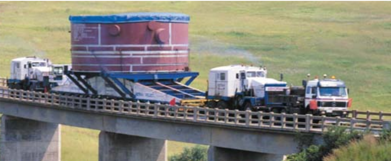
A large section of a new SAS reactor being transported from Richards Bay, on South Africa's east coast, to the Sasol Synfuels site at Secunda. This was part of the largest superload to be conveyed on South African roads
