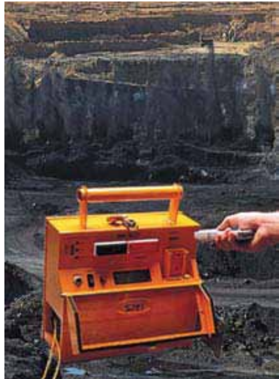
A Sasol Mining Initiators-developed electronic initiation system
