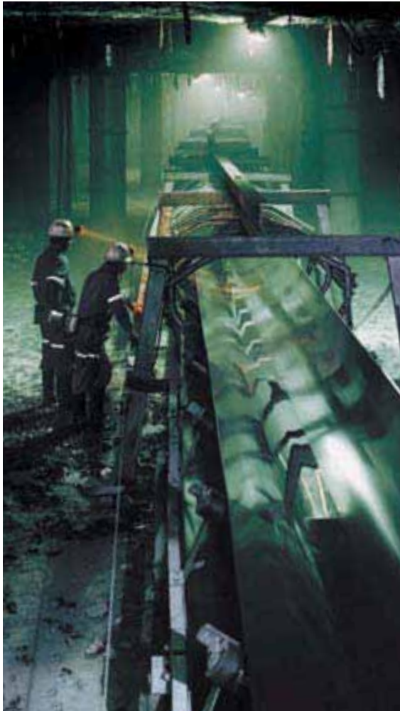
Another world first – a curved underground conveyor at the Middelbult Colliery at Secunda
