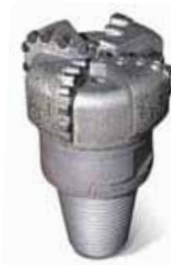
Drill bit used for directional drilling
