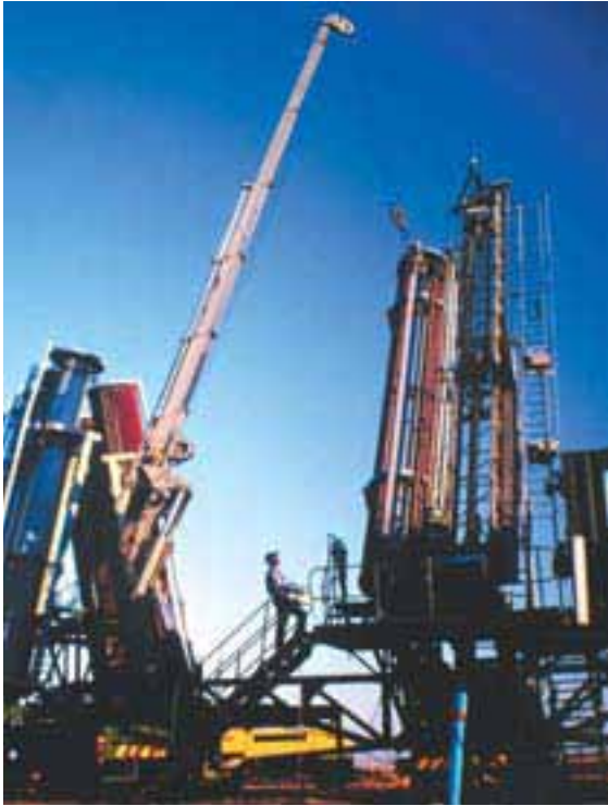
Directional drilling allows for the intensive exploration of 1 000 hectares from a single point in six months
