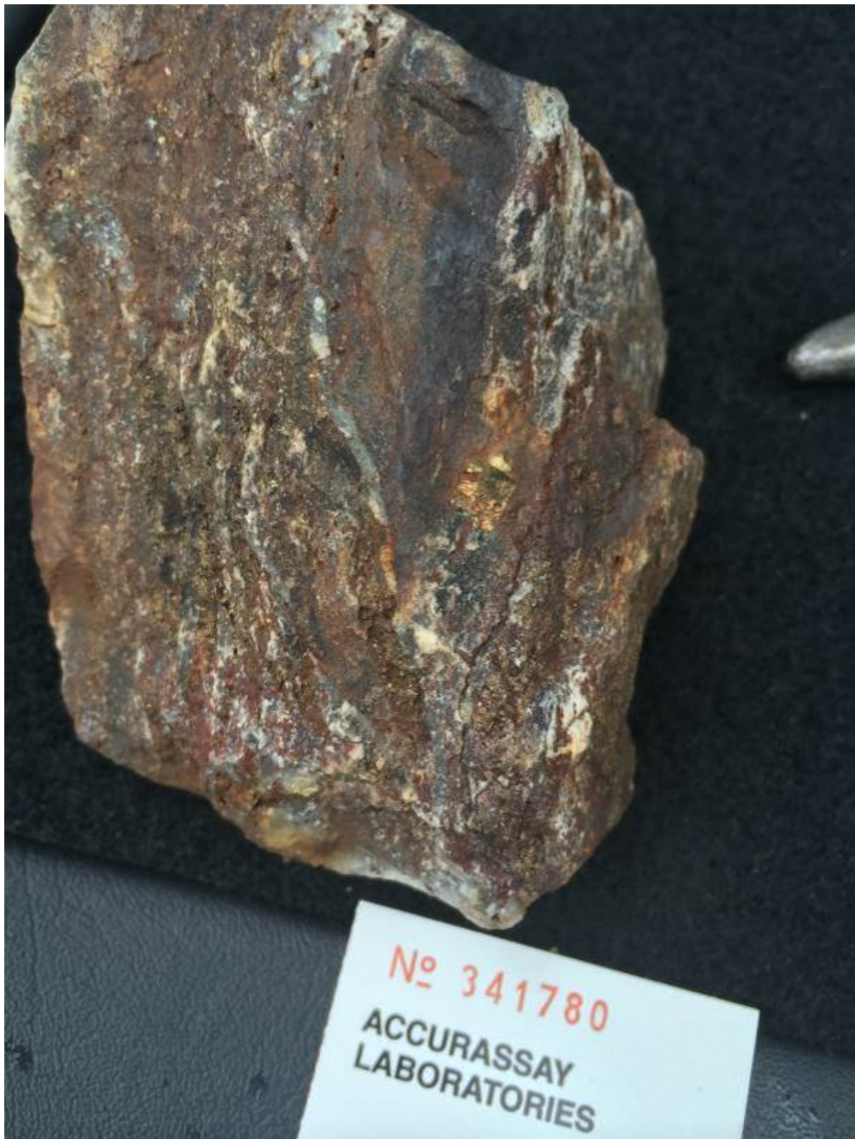
Figure 11: Emerald Lake Prospect: Sheared and silicified ironstone with pyrite after magnetite (replacement) and euhedral pyrite crystals in quartz veining. This sample assayed 3.32 g/t (check assay 2.9 g/t).
