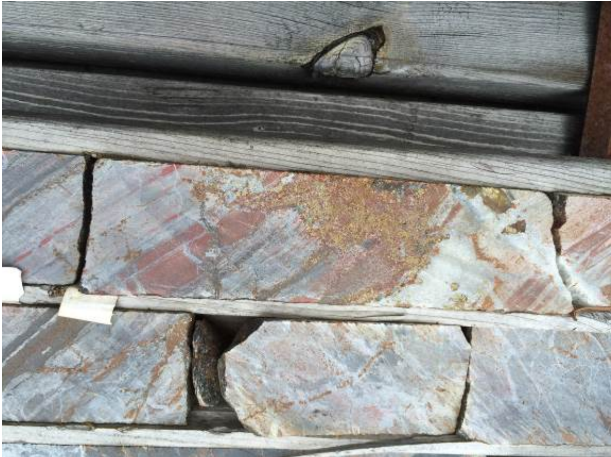
Figure 15: Core from Emerald Lake (Golden Rose) property showing ferroan carbonate – pyrite veining and pyrite replacement of ironstone bands in a dominantly brittle environment.
