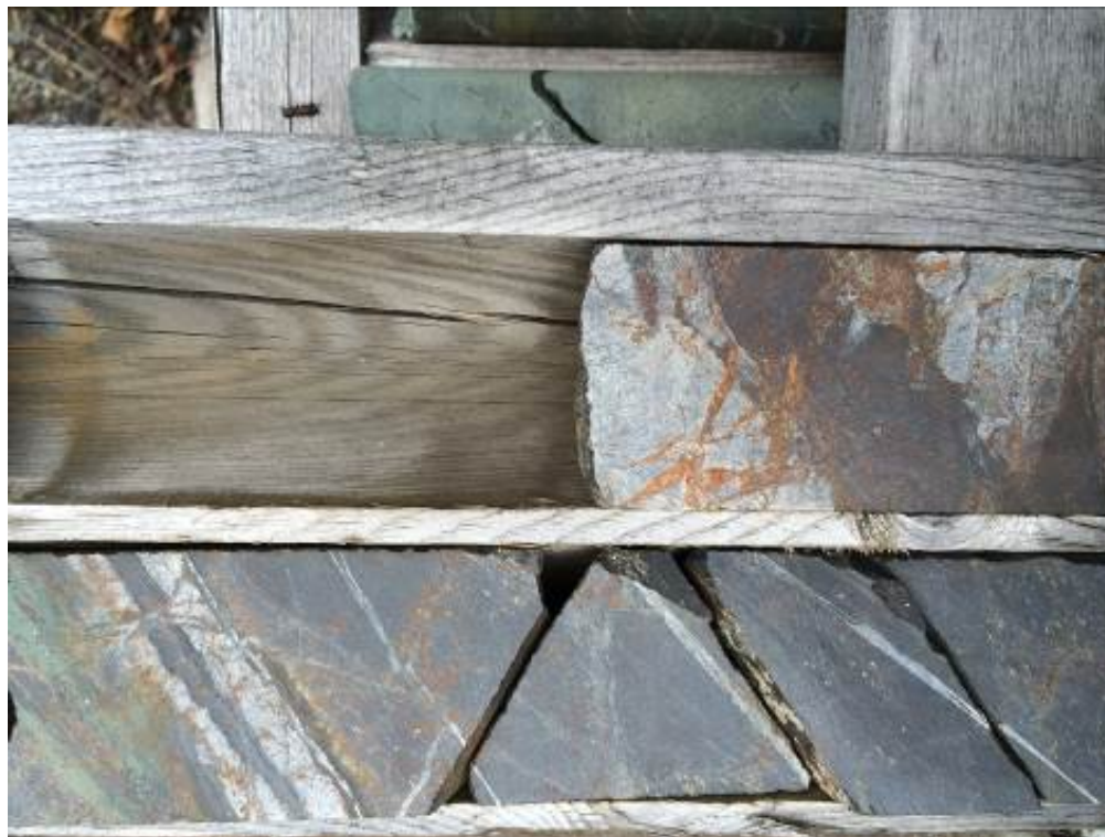
Figure 17: Cut Core from Emerald Lake with brittle crosscutting quartz and ferroan carbonate veining in BIF.
