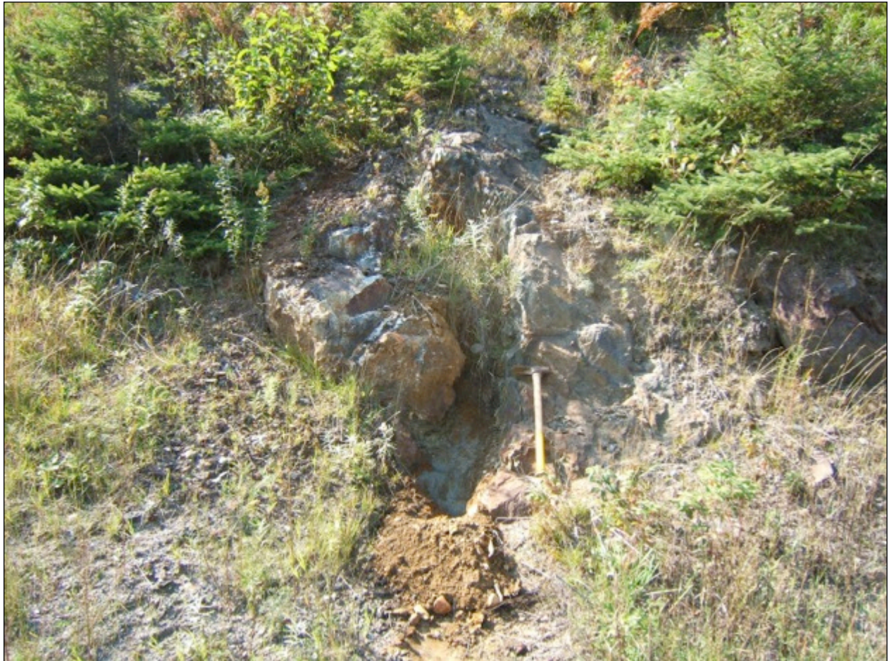
Figure 20: South Band Iron Formation in Highway Roadcut showing a quartz – tourmaline vein from which MNDM sampling documented gold values of 3,29 grams per tonne (Grabowski 2005). This is part of a zone of quartz stockworks adjoining the outcrop documented in Figure 19.
