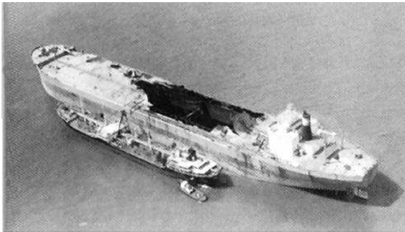
Figure 2.5: Kong Haakon deck after tank cleaning explosion. Obvious similarity to Mactra. Source: Auke Visser, supertankers.topcities.com
