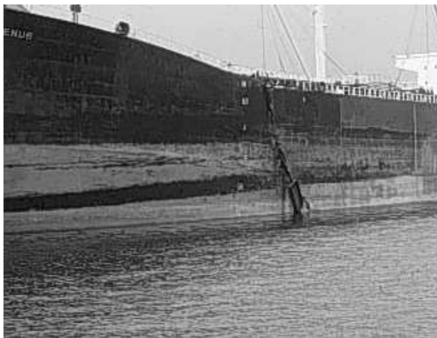
Figure 3.3: Alvenus buckled after grounding. Source: R. Hann.
