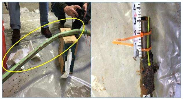
Figure 11 - Damaged Service line
