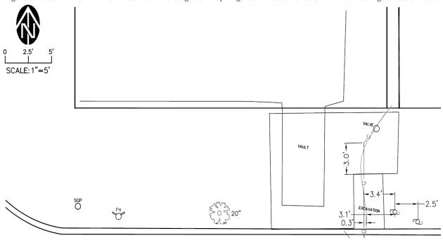
Figure 10 – NW Natural's site survey of vault, excavation area, valve, and service line.
