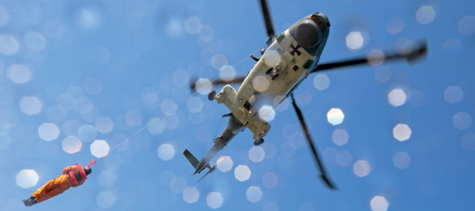
Winching a person with the SEA LYNX shipboard helicopter (Bundeswehr/Bienert)
