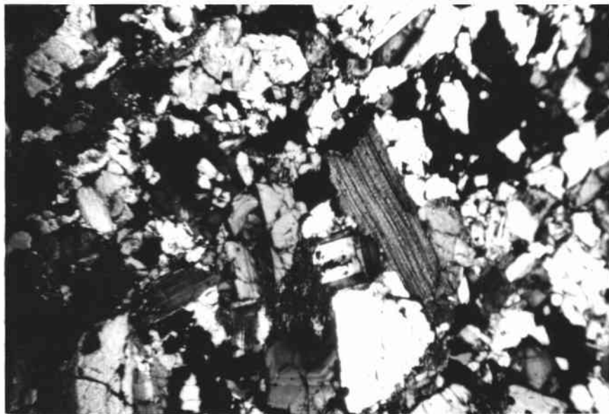
Figure 11. Photomicrograph of unmelted coarse-grained granitic fragment. - Note phenocryst of biotite with ragged and embayed edges but showing no evidence of replacement. Granophyric texture is minor.
