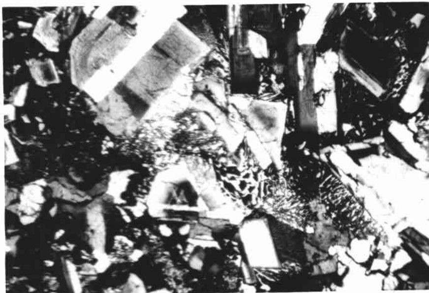
Figure 13. Photomicrograph of slightly melted coarse-grained granitic fragment. Note development of glass in the granophyric intergrowths.
