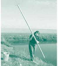
Figure 2. Sampling earthen basin with sampling probe.
