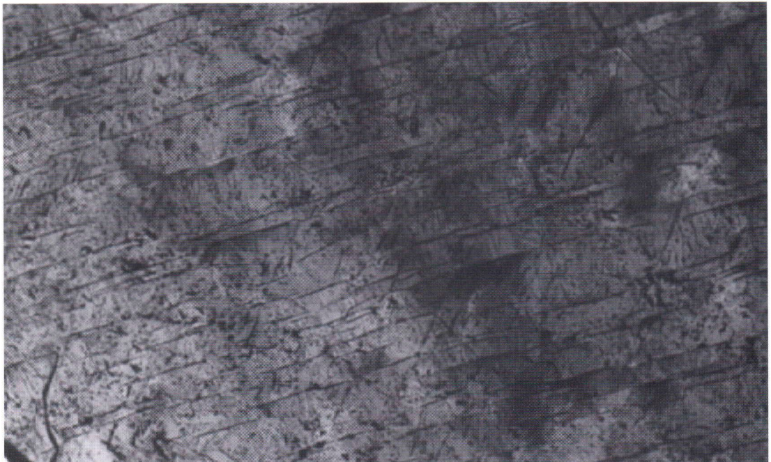
Fig.17. Quartz clast with PDFs (mostly planar fractures) parallel to (0001). DH 385, depth 141.35 m. Crossed polars. The horizontal edge of the figure is 0.69 mm.
