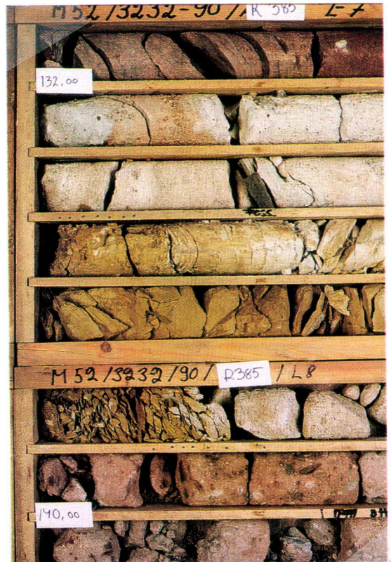
Fig. 11. Reddish conglomeratic sandstone, light grey quartz-sandstone, yellow kaolinitic clay, and red siltstone in DH 385, depth 141.5 -132.5 m. (Photo by J. Väättäinen).
