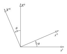
FIGURE 4.2: Minkowski space can be considered an ordinary Euclidean space where a Lorentz transformation from  $(x^1, X^0 = ict)$  to  $(x'^1, X'^0 = ict')$  corresponds to an ordinary rotation through an angle  $\theta$ . This rotation leaves the Euclidean distance  $(x^1)^2 + (X^0)^2 = x^2 - c^2t^2$  invariant.
