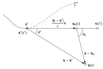
FIGURE 8.7: Signals which are observed at the field point  $\mathbf{x}$  at time t were generated at the source point  $\mathbf{x}'(t')$ . After time t' the particle, which moves with nonuniform velocity, has followed a yet unknown trajectory. Extrapolating tangentially the trajectory from  $\mathbf{x}'(t')$ , based on the velocity  $\mathbf{v}(t')$ , defines the *virtual* simultaneous coordinate  $\mathbf{x}_0(t)$ .
