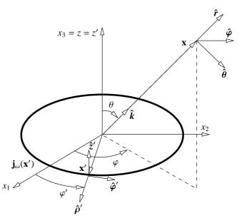
FIGURE 8.3: For the loop antenna the spherical coordinate system  $(r, \theta, \varphi)$  describes the field point  $\mathbf{x}$  (the radiation field) and the cylindrical coordinate system  $(\rho', \varphi', z')$  describes the source point  $\mathbf{x}'$  (the antenna current).
