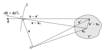
FIGURE 7.1: Relation between the surface normal and the  $\mathbf{k}$  vector for radiation generated at source points  $\mathbf{x}'$  near the point  $\mathbf{x}_0$  in the source volume V. At distances much larger than the extent of V, the unit vector  $\hat{\mathbf{n}}$ , normal to the surface S which has its centre at  $\mathbf{x}_0$ , and the unit vector  $\hat{\mathbf{k}}$  of the radiation  $\mathbf{k}$  vector from  $\mathbf{x}'$  are nearly coincident.
