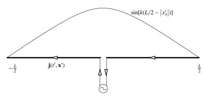
FIGURE 8.1: A linear antenna used for transmission. The current in the feeder and the antenna wire is set up by the EMF of the generator (the transmitter). At the ends of the wire, the current is reflected back with a 180° phase shift to produce a antenna current in the form of a standing wave.
