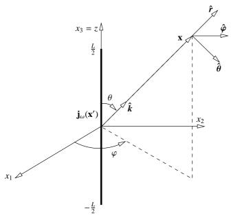
FIGURE 8.2: We choose a spherical polar coordinate system  $(r = |\mathbf{x}|, \theta, \varphi)$  and orient it so that the linear antenna axis (and thus the antenna current density  $\mathbf{j}_{\omega}$ ) is along the polar axis with the feed point at the origin.
