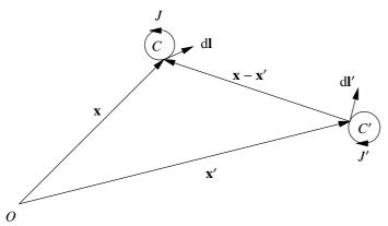
FIGURE 1.3: Ampère's law describes how a small loop C, carrying a static electric current I through its tangential line element dl located at  $\mathbf{x}$ , experiences a magnetostatic force from a small loop C', carrying a static electric current I' through the tangential line element dl' located at  $\mathbf{x}'$ . The loops can have arbitrary shapes as long as they are simple and closed.
