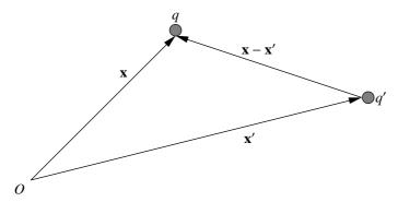
FIGURE 1.1: Coulomb's law describes how a static electric charge q, located at a point  $\mathbf{x}$  relative to the origin O, experiences an electrostatic force from a static electric charge q' located at  $\mathbf{x}'$ .
