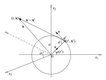
FIGURE 8.10: Coordinate system for the radiation from a charged particle at  $\mathbf{x}'(t')$  in circular motion with velocity  $\mathbf{v}(t')$  along the tangent and constant acceleration  $\dot{\mathbf{v}}(t')$  toward the origin. The  $x_1x_2$  axes are chosen so that the relative field point vector  $\mathbf{x} - \mathbf{x}'$  makes an angle  $\alpha$  with the  $x_3$  axis which is normal to the plane of the orbital motion. The radius of the orbit is  $\alpha$ .
