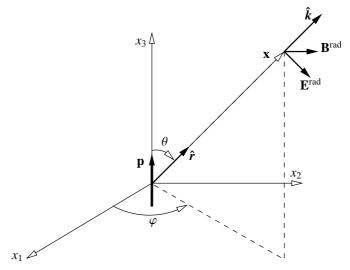
FIGURE 8.5: If a spherical polar coordinate system  $(r, \theta, \varphi)$  is chosen such that the electric dipole moment  $\mathbf{p}$  (and thus its Fourier transform  $\mathbf{p}_{\omega}$ ) is located at the origin and directed along the polar axis, the calculations are simplified.
