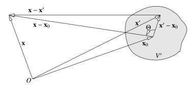
FIGURE 8.4: Geometry of a typical multipole radiation problem where the field point  $\mathbf{x}$  is located some distance away from the finite source volume V' centred around  $\mathbf{x}_0$ . If  $k |\mathbf{x}' - \mathbf{x}_0| \ll 1 \ll k |\mathbf{x} - \mathbf{x}_0|$ , then the radiation at  $\mathbf{x}$  is well approximated by a few terms in the multipole expansion.
