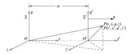
FIGURE 4.1: Two inertial systems  $\Sigma$  and  $\Sigma'$  in relative motion with velocity  $\mathbf{v}$  along the x=x' axis. At time t=t'=0 the origin O' of  $\Sigma'$  coincided with the origin O of  $\Sigma$ . At time t, the inertial system  $\Sigma'$  has been translated a distance vt along the x axis in  $\Sigma$ . An event represented by P(t, x, y, z) in  $\Sigma$  is represented by P(t', x', y', z') in  $\Sigma'$ .
