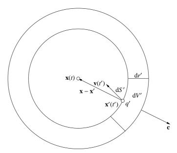
FIGURE 8.6: Signals which are observed at the field point  $\mathbf{x}$  at time t were generated at source points  $\mathbf{x}'(t')$  on a sphere, centred on  $\mathbf{x}$  and expanding, as time increases, with the velocity  $\mathbf{c}$  outward from the centre. The source charge element moves with an arbitrary velocity  $\mathbf{v}$  and gives rise to a source 'leakage' out of the source volume  $\mathrm{d}V' = \mathrm{d}^3x'$ .
