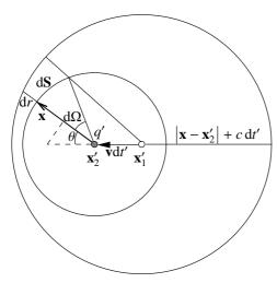
FIGURE 8.9: Location of radiation between two spheres as the charge moves with velocity  $\mathbf{v}$  from  $\mathbf{x}_1'$  to  $\mathbf{x}_2'$  during the time interval (t', t' + dt'). The observation point (field point) is at the fixed location  $\mathbf{x}$ .
