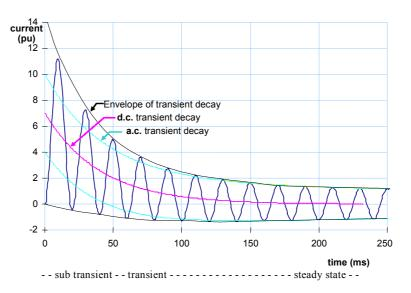
Figure 2.8 – Transient decay of current in synchronous generator
