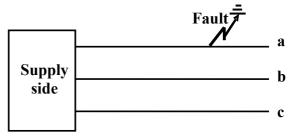
Figure 2.15 - L-G fault on phase **a**
