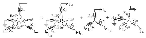
Figure 2.24 - Sequence component networks of generator
