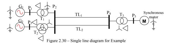
The Positive sequence network is drawn similar to the single line diagram with the generator and the synchronous motor being replaced by their internal emf and impedance. This is shown in figure 2.31a.
