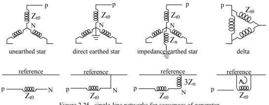
Figure 2.25 –single-line networks for sequences of generator
