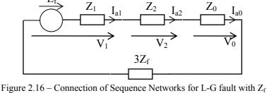
$V_{a0} + V_{a1} + V_{a2} = 3I_{a0}.Z_{f}$
