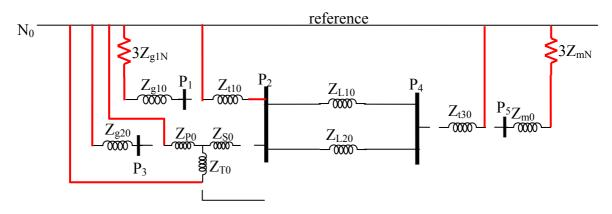
Figure 2.31c –Zero sequence diagram for Example
