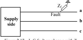
Figure 2.17 – L-G fault on phase  $\mathbf{a}$  with  $Z_{f}$
