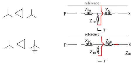
Figure 2.28a - single-line networks for sequences of three-winding transformers
