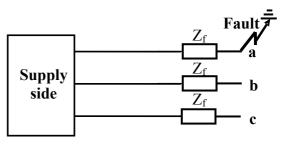
Figure 2.18 - L-G fault with  $Z_f$
