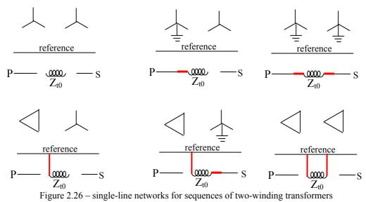
Considering the transformer as a whole, it can be seen that the single-line diagrams indicate the correct flow of the zero-sequence current from primary to secondary.
