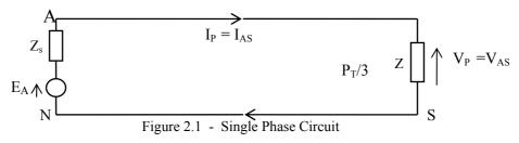
Figure 2.1 shows one single phase "AN" of the three phase circuit "ABC N". Since the system is balanced, there is no current in the neutral, and there is no potential drop across the neutral wire. Thus the star point "S" of the system would be at the same potential as the neutral point "N". Also, the line current is the same as the phase current, the line voltage is  $\sqrt{3}$  times the phase voltage, and the total power is 3 times the power in a single phase.
