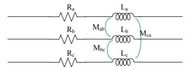
Figure 2.13 – 3 phase transmission line
