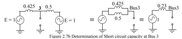
Thus, the equivalent input impedance is given by to give  $Z_{in}$  as 0.23 pu at bus 3, so that the short circuit capacity at busbar 3 is given as
