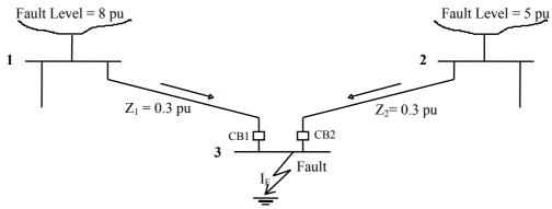
Figure 2.6 – Circuit for Fault Level Calculation
