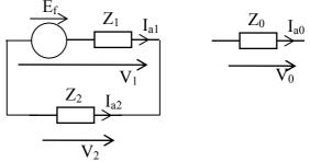
Figure 2.21 - Connection of Sequence Networks for L-L fault
