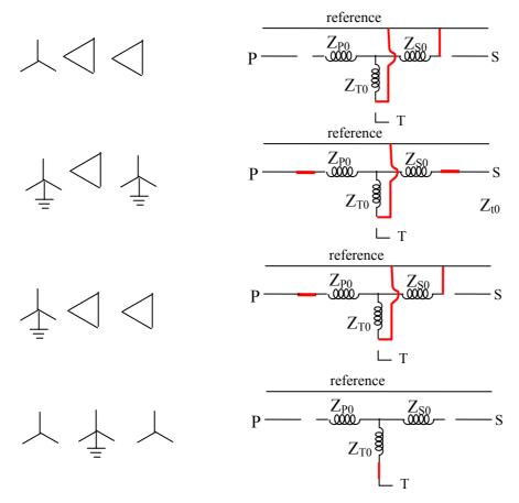
Figure 2.28b - single-line networks for sequences of three-winding transformers
