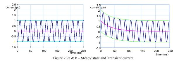
Figure 2.9a and 2.9b show the steady state current waveform, and the transient waveform of a simple R-L circuit, to show the decay in the d.c. component. In addition to this, in the synchronous machine, the magnitude of the a.c. current peak also changes with time as shown in figure 2.9c, with the unidirection component of the transient waveform removed.
