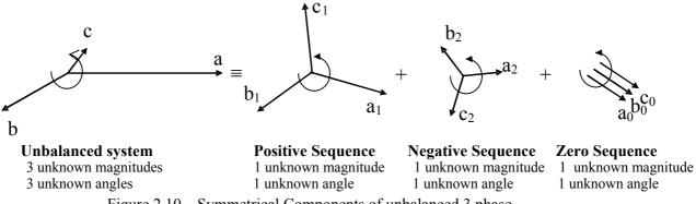
Figure 2.10 – Symmetrical Components of unbalanced 3 phase
