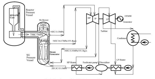
Fig. 2. Flow diagram of the HTR-PM steam turbine cycle.
