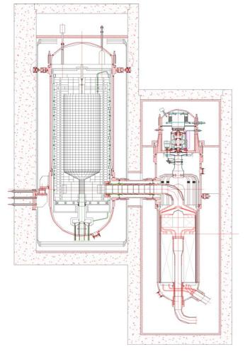
Fig. 1. Primary system of the HTR-PM.
