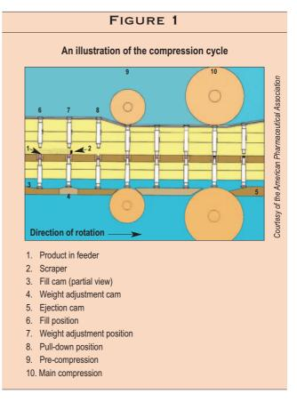
Head pressure. This factor is related to the amount of product in the overhead feed system or hopper. The more product present, the greater the head pressure, and vice versa. When the pressure varies, so does the weight of the tablets.
