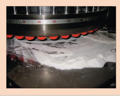
slowly as possible while maintaining proper tablet weight. Running the feeder too fast can also cause the product to segregate. See Figure 2.
