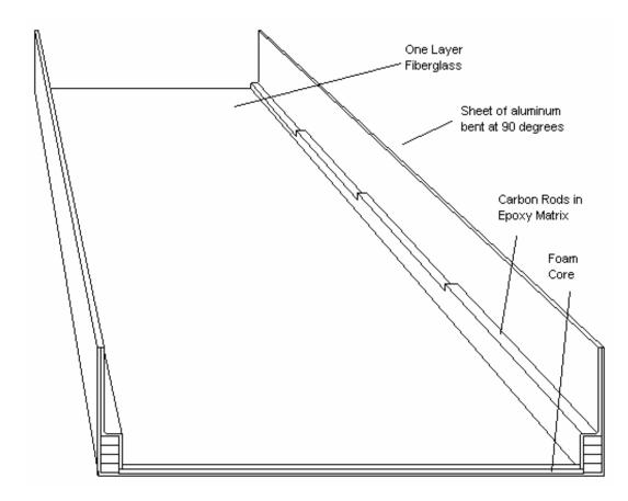
Figure 1: Spar construction
