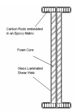
**Figure 2: Completed Spar**
