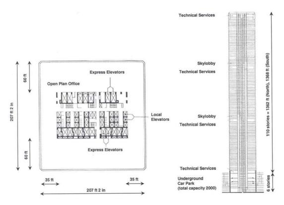
Figure 1 Typical floor layout and elevation in Twin Towers
