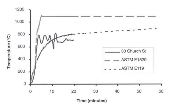
Figure 3 Time-Temperature curves from two standard tests and temperature measurements (DeCicco, et al., 1972) in the Hudson Terminal Building
