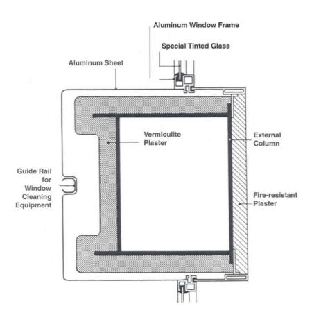
Figure 2 Fire Protection for typical Exterior Columns in Twin Towers
