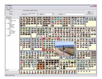
Figure 1 A prototype interface for semi-automatic image annotation based on PhotoMesa[2]. Photos are laid out within a zoomable space grouped by event that is detected by hierarchical event clustering. Users can drag labels on image groups to make bulk annotation.
