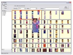
Figure 3 Identified people who are cropped from photos are laid out on the screen ready to be annotated. Torsos are detected by using face detection. Similar torsos which have short visual distances with each other are clustered together.
