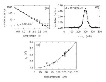
FIG. 11. Measurement of the cyclotron damping rate at 146.70 GHz, near the upper sideband of  $TE_{136}$ . The cyclotron damping rate as a function of axial amplitude (c) extrapolates to the desired lifetime. Each point in (c) consists of a damping rate measured from a fit to a histogram of cyclotron jump lengths (a) as well as an axial amplitude measured from a driven cyclotron line (b).
