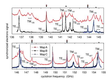
FIG. 10. (Color) Modes of the trap cavity as observed with synchronized electrons in three separate sweeps. The calibration frequencies are indicated with symbols above the plots. The striking difference between maps B and C and map A is discussed in the text.
