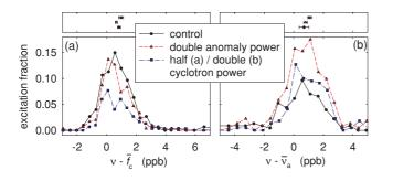
FIG. 14. (Color online) The lower plots show cyclotron (a) and anomaly (b) data taken in search of cyclotron and anomaly power shifts. The upper plots compare the weighted means of these lines.
