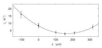
FIG. 13. Measurement of the offset between the electrostatic and mode centers. Here, z refers to the position relative to the electrostatic center, and the minimum in the cyclotron damping rate corresponds to the mode center.
