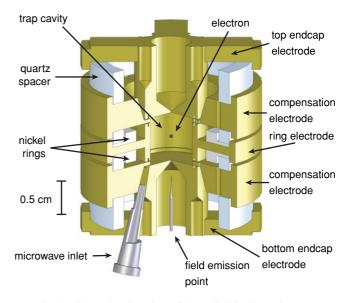
FIG. 4. (Color) Section view of the cylindrical Penning trap cavity used to confine a single electron and inhibit spontaneous emission. The electrodes facing the electron are cylindrically symmetric except for the compensation electrodes, each of which are split vertically in half. Microwaves with a 2 mm wavelength enter the trap through the squeezed tube that is the microwave inlet.
