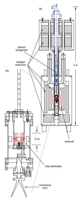
FIG. 5. (Color) An overview of the apparatus (a), including a 10-times enlarged view (b) of the vacuum enclosure for the Penning trap electrodes. The solenoid and electrodes are in red. The dilution refrigerator is in blue. Cryogen spaces are hatched.
