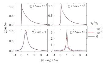
FIG. 9. (Color online) The theoretical Brownian-motion lineshape for various  $\gamma_z/\Delta\omega$  and  $\gamma_c/\gamma_z$ . Our cyclotron line has  $\gamma_z/\Delta\omega \approx 10^{-2}$ . Our anomaly line has  $\gamma_z/\Delta\omega \approx 10$ . For our  $\gamma_z$ ,  $\gamma_c/\gamma_z = 10^{-1}$ –  $10^{-2}$  correspond to lifetimes of 1.6 s–16 s. The infinite-lifetime limit is  $\gamma_c/\gamma_z = 0$ .
