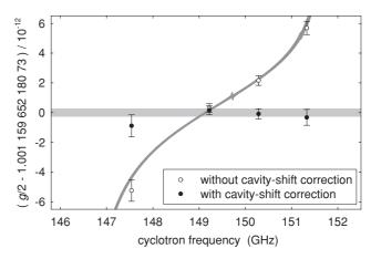
FIG. 15. Four measurements of g/2 without (open) and with (filled) cavity-shift corrections. The light gray uncertainty band shows the average of the corrected data. The dark-gray band indicates the expected location of the uncorrected data given our result in Eq. (65) and including only the cavity-shift uncertainty.
