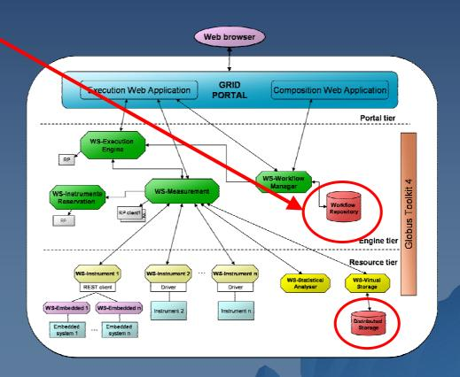
The WS-Instrument services are in charge of communicating with the real devices.
