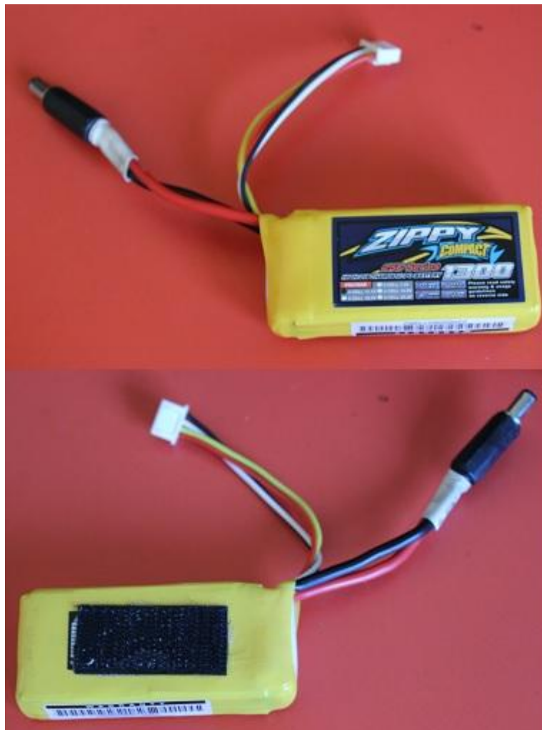
Figure 3.15: 1300 mAh and 11.1 V LIPO battery.
