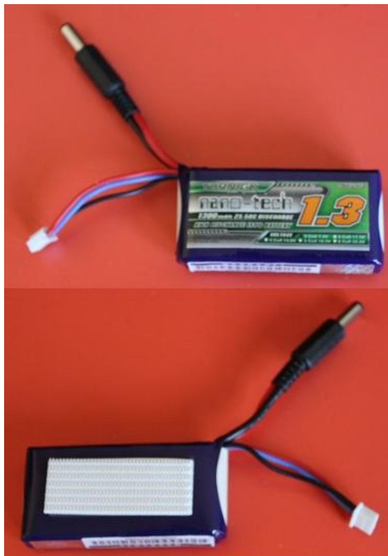
Figure 3.16: 1300 mAh and 7.4 V LIPO battery.
