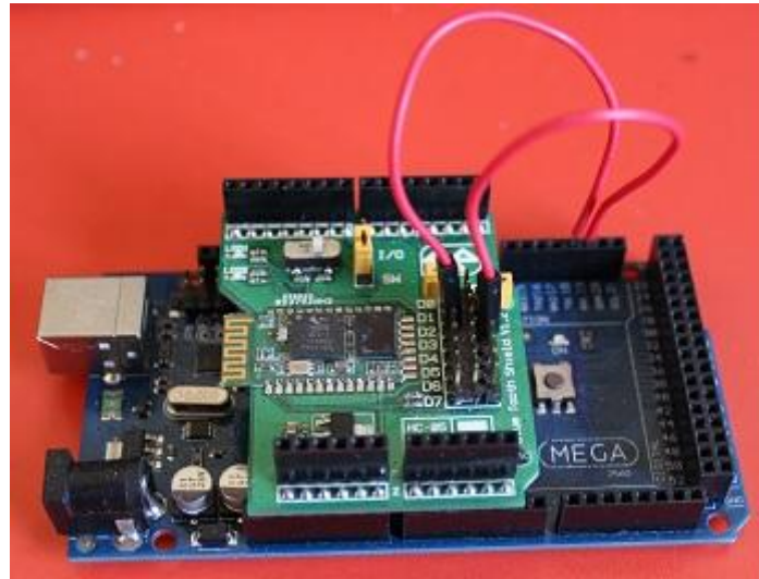
Figure 5.8: Master Bluetooth Shield with Arduino MEGA board.
