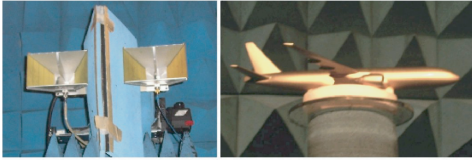
Figure 1: Horn radar antennas (transmitting and receiving) (left), and model mounted on a rotating pedestal (right), inside the anechoic chamber.
