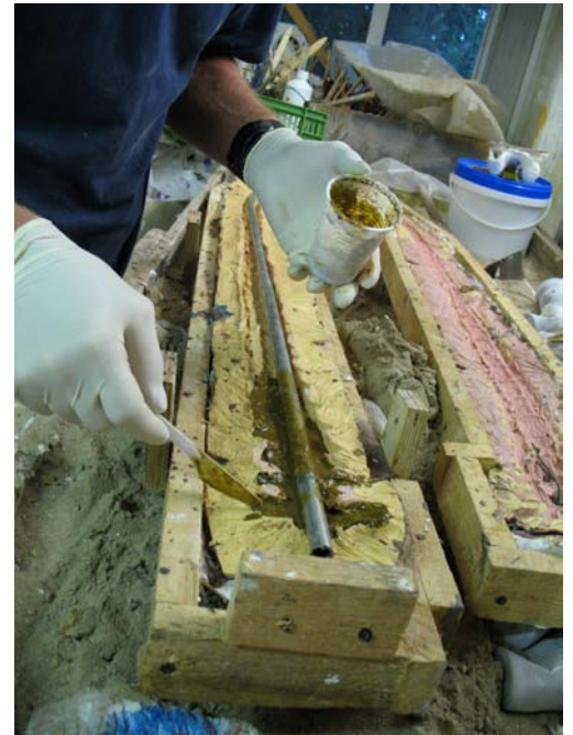
Fig. 13 – Casting: A – using a pouch as a pastry bag containing polyester resin; notice the piece of steel wire inside the mould, providing a rigid structure to the cast. B – applying polyester resin; this layer serves as the base colour for the subsequent painting (photos by Pedro Viegas).
