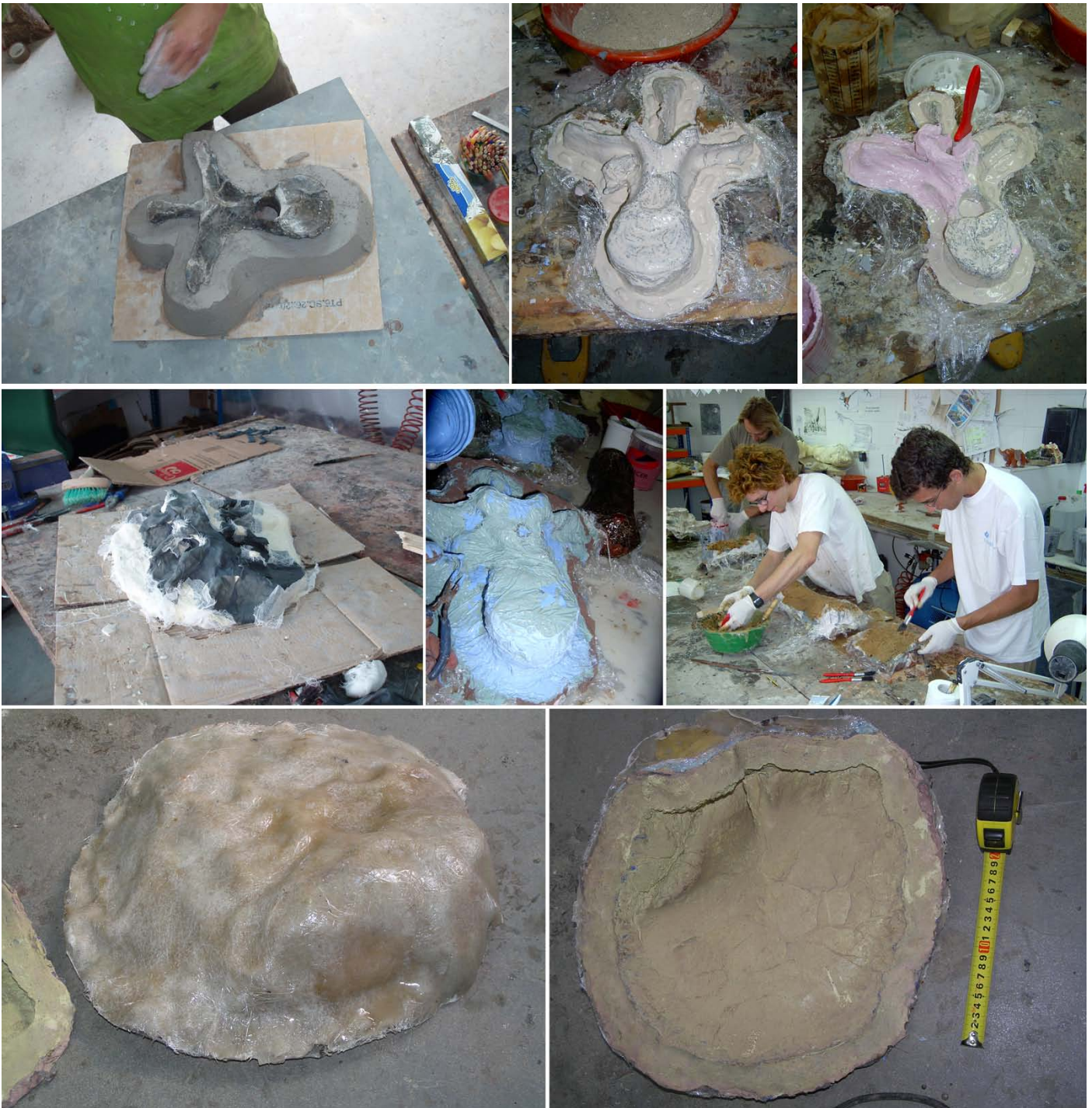
Fig. 11 – General procedure for moulding: A – defining thoughtfully where the mould should be divided, clay is used to separate the two parts of the mould; B – application of the first thin layer; C – in the second layer thixotropic additive is added, giving a yoghurt viscosity to the silicone; D – ladies stockings can be applied directly on the mould or pieces of cotton cloths can be embedded with silicone with a spatula before proceeding to its application on the previous layer of the mould; E – aspects of the mould with all the silicone layers applied; F – plastic film should be applied before making the supporting mould; G – aspect of the supporting mould once dried; H – on the other side, the final aspect of the silicone rubber.
