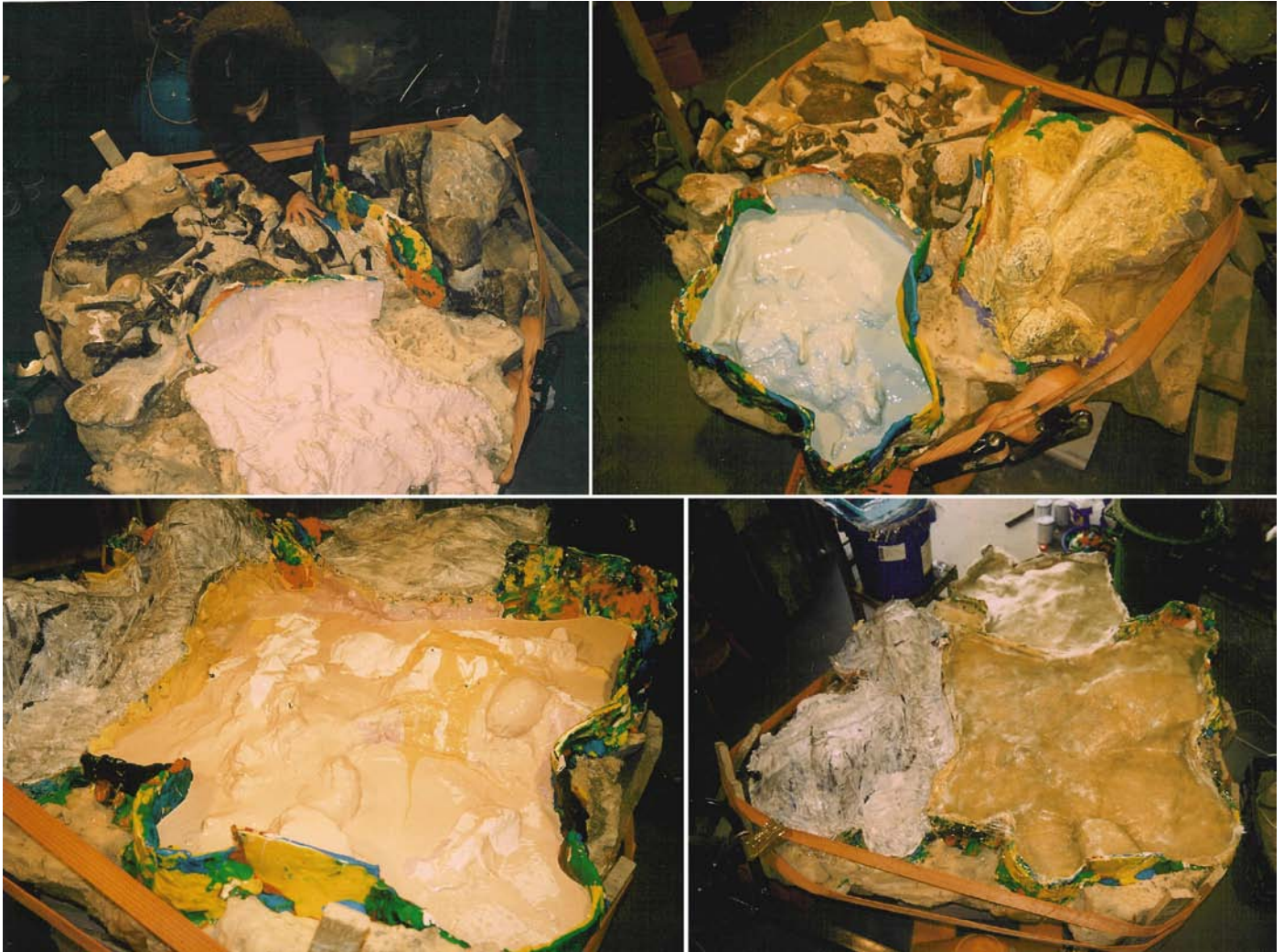
Fig. 10 – Moulding the main block: A – raising modelling clay retaining walls; B – aspect of the block after applying the first layer of silicone; C – aspect of the mould once the second and third layers of silicone were applied; D – polyester resin supporting mould.
