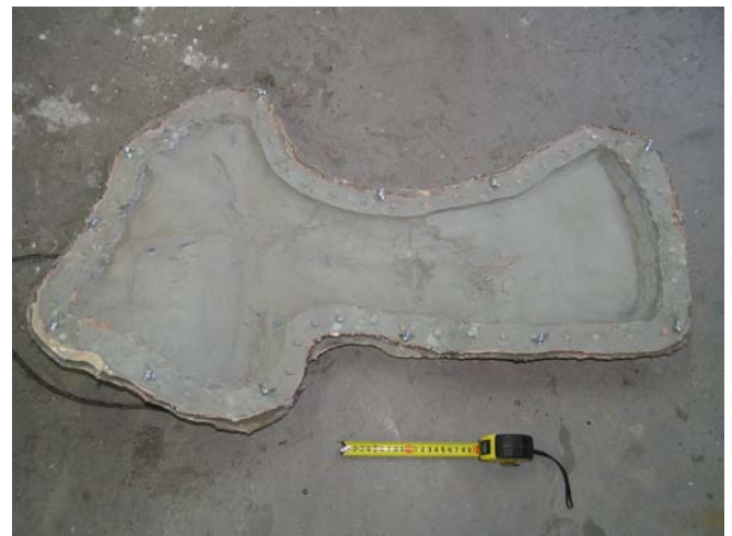
Fig. 12 – Storing moulds: screws attach the silicone mould to the rigid polyester resin supporting mould.
