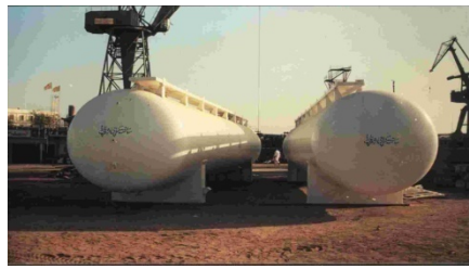
LPG Storage Tanks
