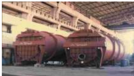
Fire Tube Boilers
