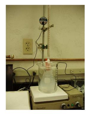
*Figure 2.* The set-up used to measure the volume expansion upon injection at  $37^{\circ}$ C.
