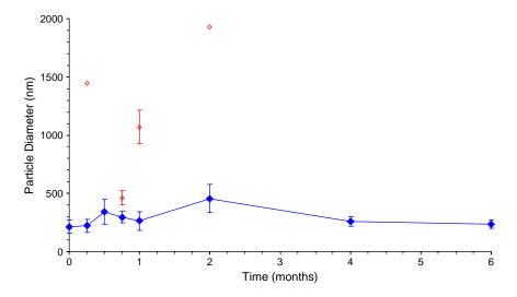
*Figure 3.* The particle-size distribution of DDFPe for 6 months at  $23^{\circ}C \pm 2^{\circ}C$ . The error bars represent one standard deviation of the triplicate measurements. The open diamonds represent measurements of less than 2% of the particle distribution at that timepoint.
