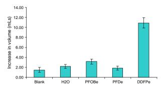
*Figure 5.* Volume increase upon heating 5 mL injections of the 3 PFC emulsions, the blank formulation, and water to  $37^{\circ}$ C.
