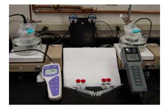
*Figure 1.* The set-up used for measuring oxygen absorption. The vials on the left contain one of the PFC emulsions and the vials on the right contain the blank formulation.
