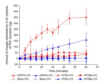
*Figure 4.* The amount of oxygen absorbed by 5 mL injections of DDFPe (triangles), PFDe (diamonds), PFOBe (squares), and the formulation blank (open circles) at 21C (blue) and 37C (red) over the course of 60 minutes.
