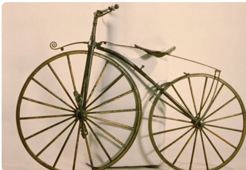
FIGURE 2 Velocipede by Pierre Michaux et Cie of Paris, France circa 1869. In the wake of the draisine, the next major development in bicycle design was the velocipede, which was developed in France and achieved its greatest popularity in the late 1860s. The velocipede marks the beginning of a continuous line of developments leading to the modern bicycle. Its most significant improvement over the draisine was the addition of cranks and pedals to the front wheel. Different types of (not very effective) braking mechanisms were used, depending on the manufacturer. In the case of the velocipede shown, the small spoon brake on the rear wheel is connected to the handlebar and is engaged by a simple twisting motion. The wheels are wooden wagon wheels with steel tires. (Reproduced with permission of the Canada Science and Technology Museum, Ottawa, Canada.)
