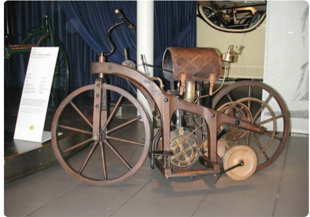
FIGURE 5 Daimler petrol-powered motorcycle. Gottlieb Daimler, who later teamed up with Karl Benz to form the Daimler-Benz Corporation, is credited with building the first motorcycle in 1885. (Reproduced with permission of DaimlerChrysler AG, Stuttgart, Germany.)
