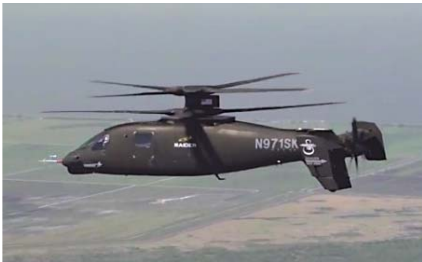
Above: Sikorsky recently resumed flight testing of the S-97 Raider compound helicopter, with a series of high speed flights away from the Palm Beach airport boundary.
