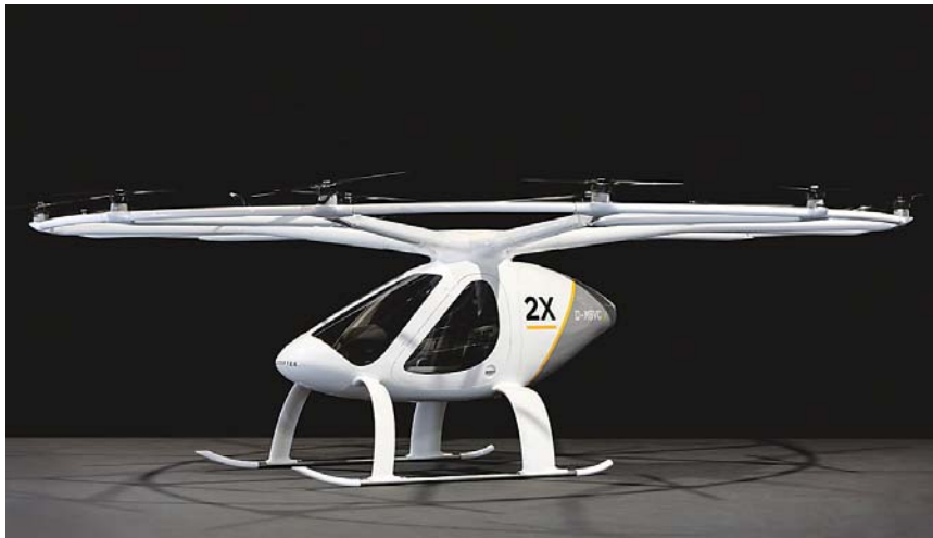
Above: e-volo has launched a two-seat Model 2X version of its electric-powered Volocopter.
