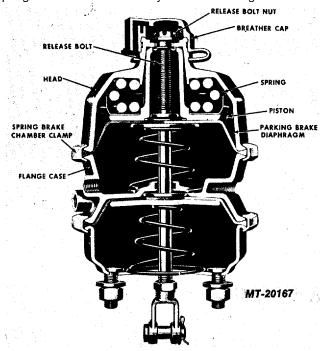
Cross Section of MGM Spring Brake Assembly
