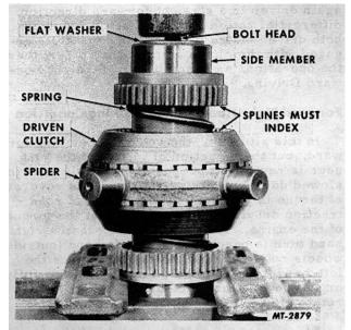
Fig. 44 Release of Spring Pressure
