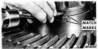
Fig. 12 Marking Differential Case Halves
