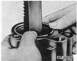
Fig. 31 Install End Plate Retaining Ring
