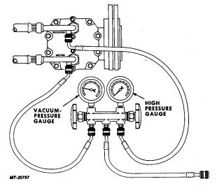
Fig. 35 Manifold and Garage Set Connected to Compressor Service Port
