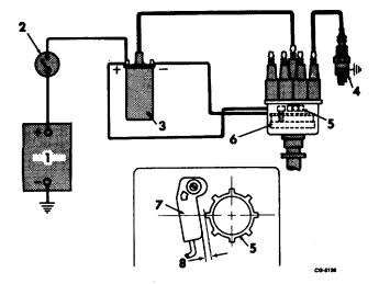
Fig. 1 Schematic View of Ignition System
