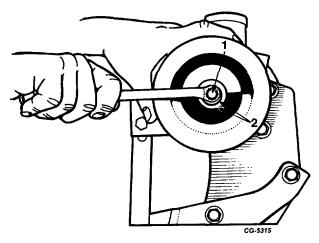
Fig. 22 Removing Power Steering Pump Pulley Bolt
