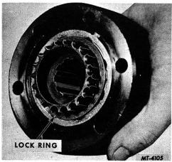
*Fig. 13. Hub Body* Remove the 10 rollers (7) from the roller cage (9). Take out centering spring (8). See Fig. 14.
