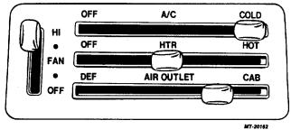
Fig. 23 Controls Set for Dehumidification of Cab
