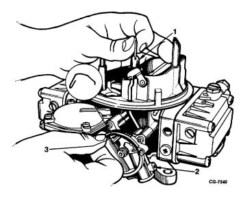
Figure 59. Checking Choke Qualifying Dimension
