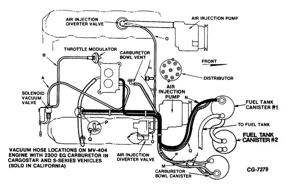
Fig. 85 Vacuum Hose Locations on MV-404 Engine With 2300 EG Carburetor in Cargostar and S-Series Vehicles With Three Vapor Storage Canisters (Sold in California)
