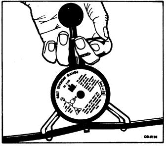
Fig. 64 Checking Belt Tension With SE-2312 Gauge
