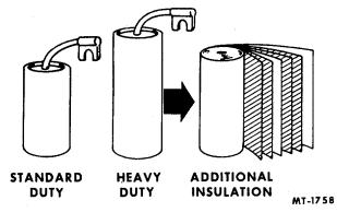
Fig. 9 Comparison Between Standard and Heavy-Duty Condenser
