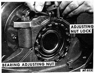
Fig. 9 Adjuster Lock Removal
