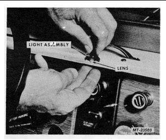
Fig. 17 Instrument Panel Control Light
