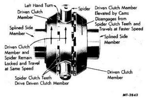
Fig. 40 Left-Hand Turn--Forward Direction
