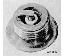
Fig. 4 Normal Spark Plug Appearance
