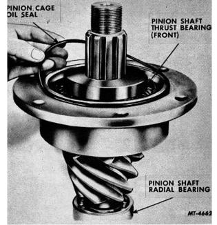
Fig. 7 Removing Pinion Cage Oil Seal
