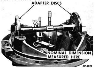
Fig. 28 Assembled Gauge in Position
