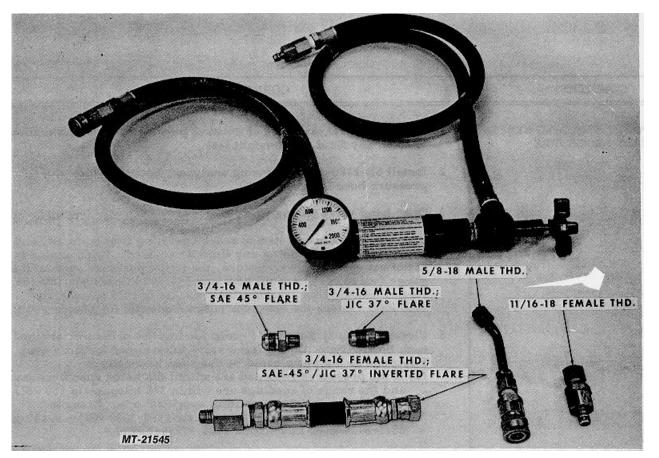
Fig. 7 SE-2780 Power Steering Analyzer
