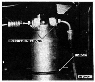
Fig. 50 Filter-Dehydrator Mounting
