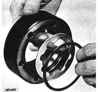
Fig. 18. Removing Spirolox Lock Ring and Thrust Washer
