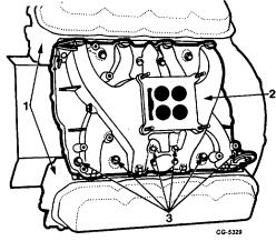
Fig. 36 Intake Manifold Removal
