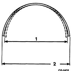
Fig. 125 Illustrating Bearing Spread
