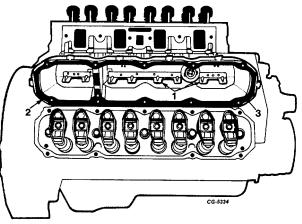
Fig. 41 Removing Cylinder Head Covers
