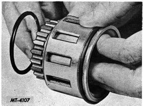
Fig. 14. Removing Centering Spring and Rollers
