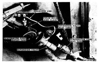
Fig. 49 Removing Expansion Valve
