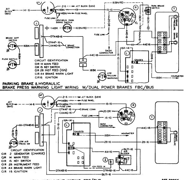
LOW AIR PRESS WARN LIGHT WIRING FBC/BUS
