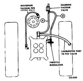
Fig. 95 Vacuum Hose Locations on V-537 Engine With 4150G Carburetor in Cargostar and S-Series Vehicles (Sold in Canada)
