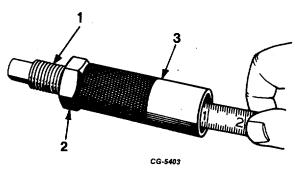
Fig. 109 Adjusting Valve Guide Installer SE-1943 for Proper Height
