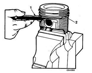
Fig. 100 Checking Ring-to-Groove Side Clearance with Feeler Gauge
