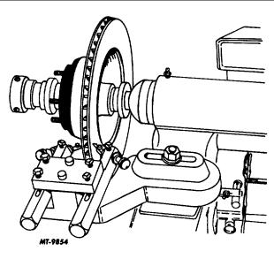
Fig. 19 Correct Method of Refacing Rotor
