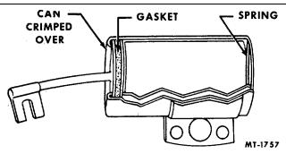
Fig. 8 Construction of Condenser
