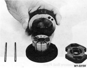
Fig. 15 Removing Pump Ring
