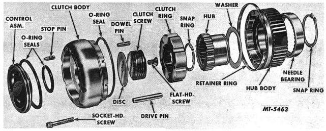
Fig. 9. Manual Type Locking Hub with Socket Head Mounting Screw (Exploded View)
