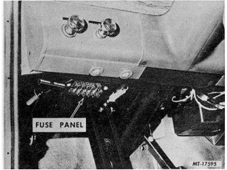
Figure 4 Figure 4 Fuse Panel Location Scout II Vehicles
