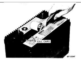
Fig. 11 Removing Section of Top Plaque to Gain Access to Cell Caps (Top Terminal Maintenance Free Battery)
