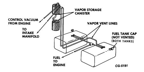
Fig. 29 CO-1610B and COF-1910B Cargostar Vehicles With 50 Gallon Dual Fuel Tanks
