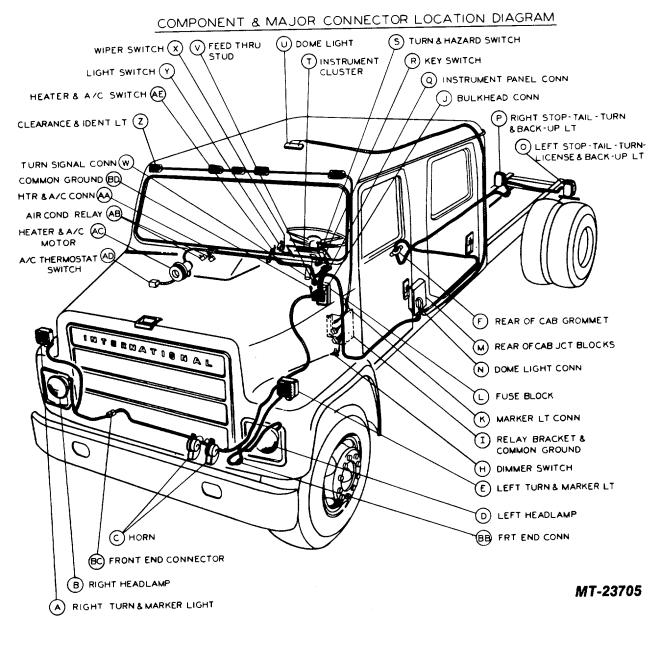
Component And Major Connector Location (On Chassis) 1700 thru 1900 Models
