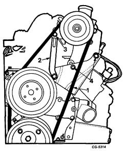
Fig. 21 Removing Power Steering V-Belt
