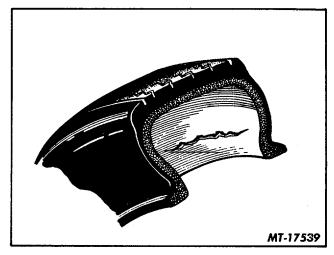
Fig. 19 Broken Cords Caused by Severe Blow
