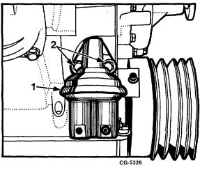
Fig. 33 Fuel Pump Removal
