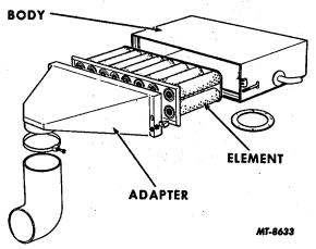
Fig. 4 Typical Dry Type Air Cleaner (Box Type)
