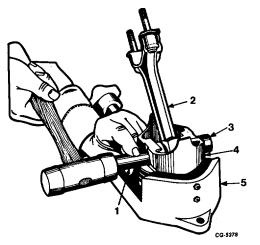
Fig. 85 Removing Piston Pin
