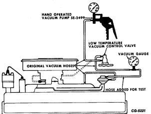
Fig. 52 Low Temperature Vacuum Control Valve and Connecting Hose Test
