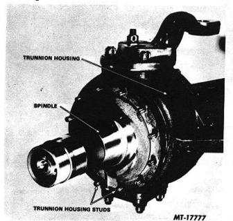
Fig. 1 Removing Spindle
