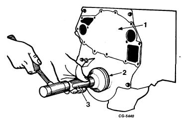
Fig. 148 Installing Engine Front Cover Oil Seal with Cover Assembled to Cylinder Block Using SE-1949 Installer
