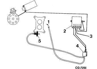
Figure 18 Deceleration Throttle Modulator System (Typical)
