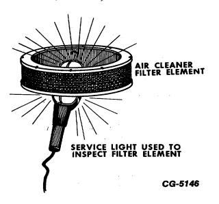
Fig. 7 Dry Type Air Cleaner Filter
