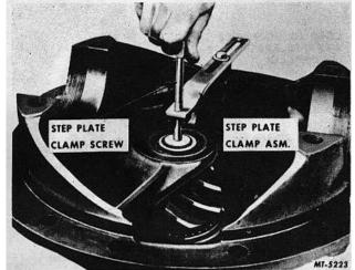
Fig. 13 Locating Step Plate Clamp
