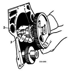
Fig. 62 Camshaft Removal
