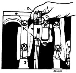
Fig. 59 Connecting Rod Cap Removal
