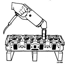
Fig. 115 Grinding Seats Using SE-1631 Grinder
