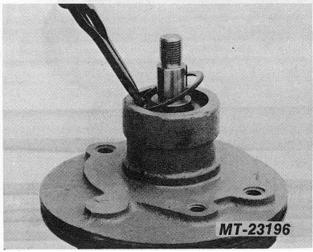
Fig. 17 Remove Retaining Ring
