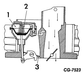
Figure 19 Secondary Throttle Operation (Low Speed or Light
