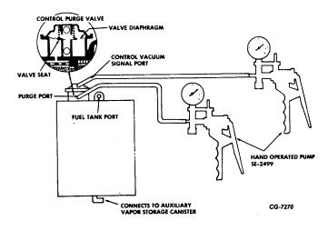
Fig. 17 Canister Purge Control Valve Diaphragm and Valve Seat Test
