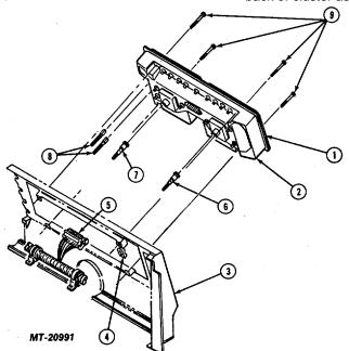
Fig. 2 Removing Instrument Cluster
