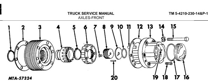
Fig. 6. Locking Hub (Manual Type with Hex Head Mounting Bolts) (Exploded View)
