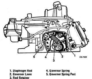
Figure 42 Interior View of Governor Housing
