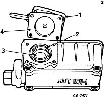
Figure 15 Acceleration Pump Assembly (shown with plastic pump inlet valve used on later model carburetors).
