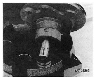
Fig. 23. Remove Needle Bearing and Seal
