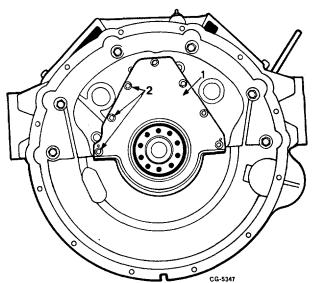
Fig. 54 Rear Oil Seal Retainer Plate Removal
