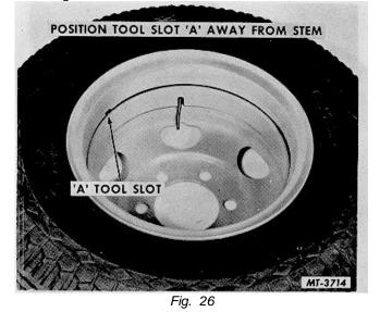
Step on the ring to force tire down, until cut-away "AA" on ring slip over the edge and hook on rim. Then insert tool into tool slot and push outward (Fig. 26). Hold onto tool and hammer the ring between slot and nearest cut away. This action will hook ring and rim together.
