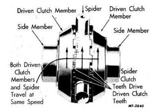
Fig. 38. Right-Hand Turn--Forward Direction
