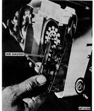
Fig. 24 Removing Air Pressure Gauges
