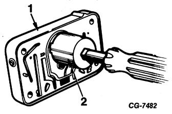
1. Metering Block 2. Power Valve Socket Figure 30 Using Socket Wrench SE-1772-1 to Remove Power Valve
