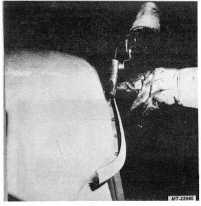
Fig. 51. Fastening Roof Panel To New Side Panel
