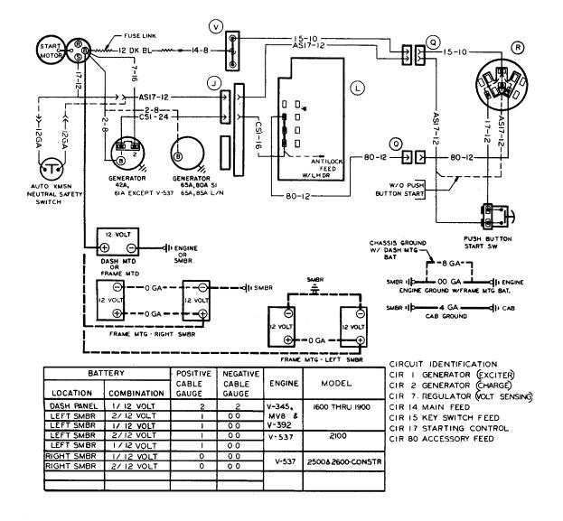
V-392, V-345, MV8 & V-537 STARTING, CHARGING & MAJOR FEED & GROUND WIRING MT-21960
