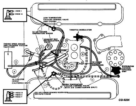
Fig. 89 Vacuum Hose Locations on V-304;345 Engines With 2210C Carburetor in Scout Vehicles (Sold in Canada)
