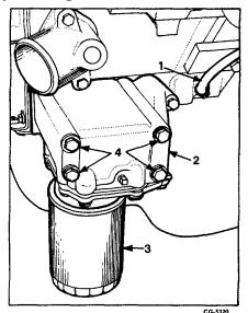
Fig. 27 Oil Cooler and Filter Removal
