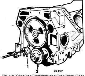
Fig. 145 Checking Camshaft and Crankshaft Gear Backlash
