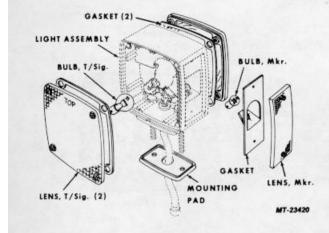
Fig. 9 Front Turn Signal/Marker Light
