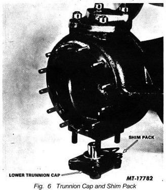
The lower trunnion bearing will lay loose on bottom of trunnion housing when lower trunnion cap is removed. Remove lower trunnion bearing by pulling trunnion housing away from axle housing to provide access to bearing as shown in Figure 7.
