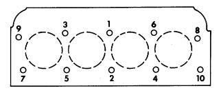
CG-5443 Fig. 151 Cylinder Head Mounting Bolt Tightening Sequence
