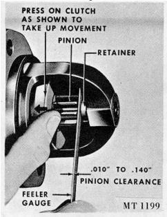
Fig. 13 Checking Pinion Clearance
