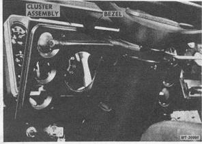
Fig. 6 Removing Instrument Cluster Bezel
