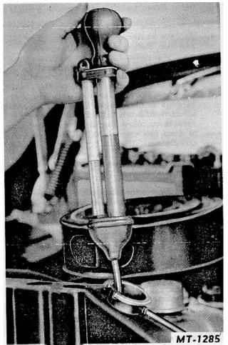
Fig. 8 Using Hydrometer to Test Antifreeze Solution
