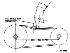
Conventional "V " belts are used on the engine to drive the fan and various accessories. Belt tensions are as follows:
