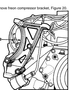
Fig. 20 Freon Compressor Bracket Removal
