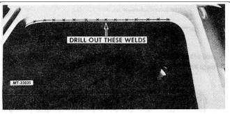
Fig. 46. Side Panel to Roof Inner Panel Spot Welds
