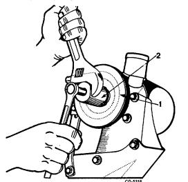
Fig. 23 Using SE-2420 Puller to Remove Power Steering Pump Pulley
