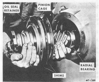
Fig. 5 Removing Pinion and Cage Assembly
