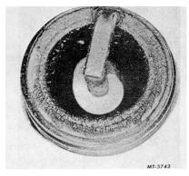
Fig. 13 Chipped Insulator
