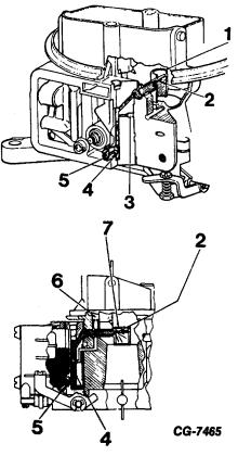
Figure 9 Main Metering Fuel Air Flow 1. Booster Venturi
