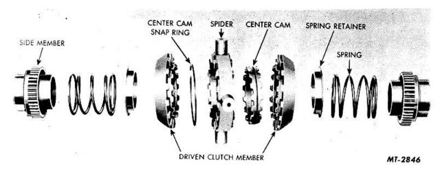
Fig. 34 Internal Spring Design differential Locking Unit (Exploded View)
