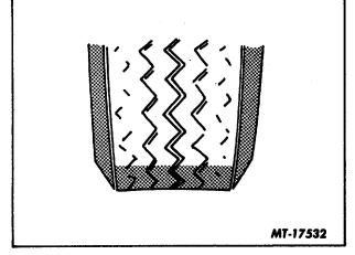
Fig. 12 Underinflation Causes Excessive Side Tread Wear
