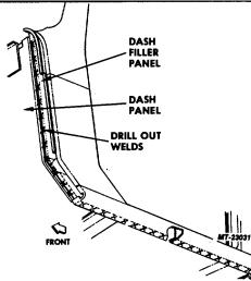
Fig. 42. Filler Panel to Dash Panel Spot Welds
