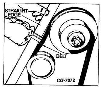
Fig. 65 Measuring Belt Tension
