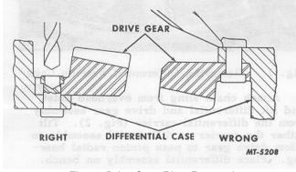
Fig. 3 Drive Gear Rivet Removal
