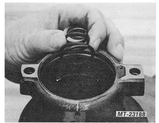
Fig. 9 Remove Spring
