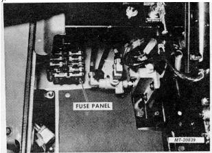
Fig. 13 Fuse Panel Location S-Series Vehicles
