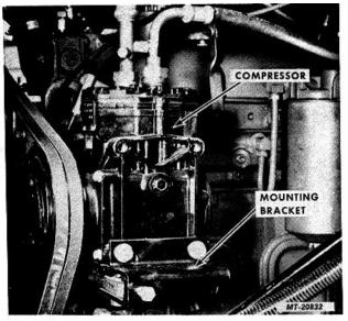
Fig. 41 Compressor Mounting (Typical)
