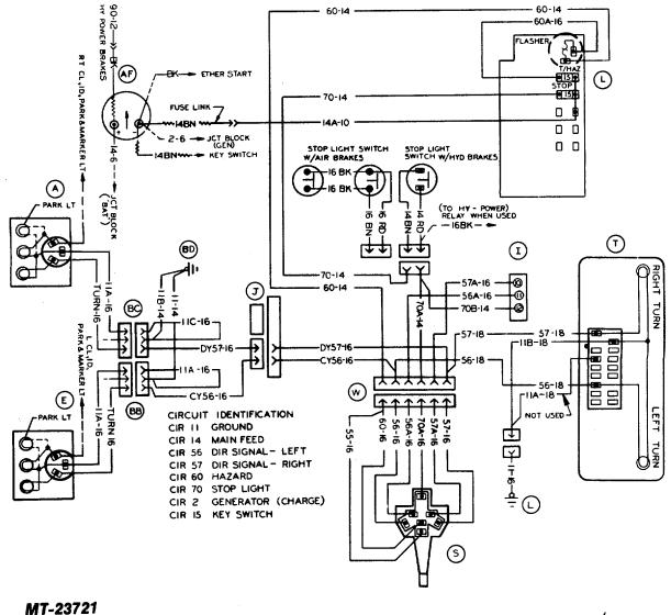
TURN HAZARD & STOP LIGHT WIRING - FBC/BUS
