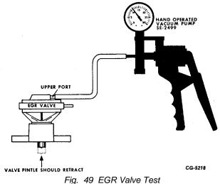
b. Apply 10-12" vacuum to EGR valve vacuum port (upper port of dual diaphragm valve). As vacuum is applied, valve pintle should move off seat and retract into valve housing (Fig. 49). If valve does not operate when vacuum is applied, valve is faulty and
