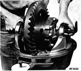
Fig. 11 Lifting out Differential and Gear Assembly
