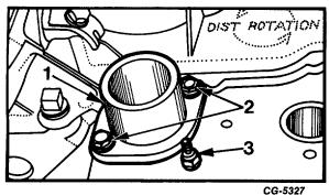
Fig. 34 Thermostat and Sender Unit Removal
