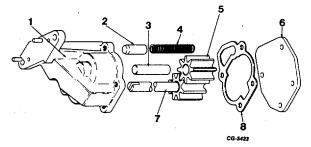
Fig. 130 Exploded View of Oil Pump
