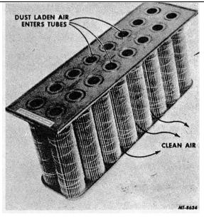
Fig. 5 Box Type Dry Air Cleaner Element
