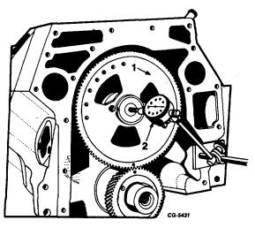
Fig. 139 Checking Camshaft End Play
