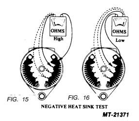
If a shorted or open diode is detected in the preceding tests, the entire heat sink assembly should be replaced.
