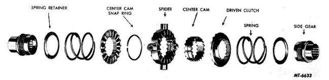
Fig. 35. External Spring Design Differential Locking Unit (Exploded View)
