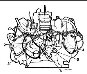
Fig. 28 Distributor and Wiring Removal
