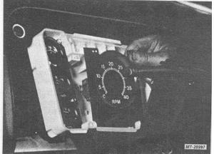
Fig. 8 Removing Tachometer
