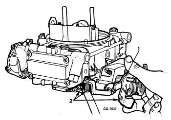
Figure 55. Accelerating Pump Lever Adjustment 1. Location of Pump Cam
