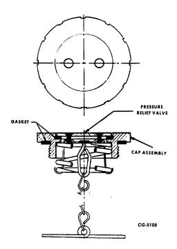
Fig. 20 Fuel Tank Cap (Nonvented Type)
