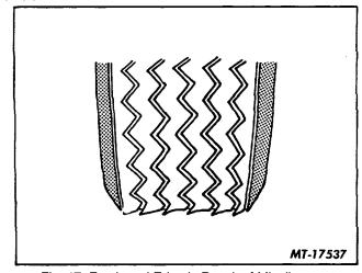
Fig. 17 Feathered Edge is Result of Misalignment
