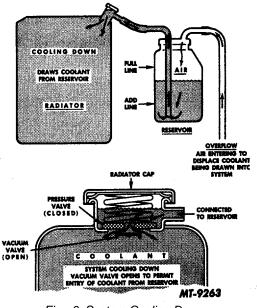
Fig. 6 System Cooling Down
