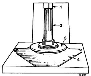
Fig. 142 Pressing Rear Oil Seal into Retaining Plate Using SE-1905 Installer with 5-1/4" O.D. Adapter
