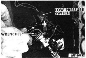
Fig. 55 Removing Low Pressure Switch
