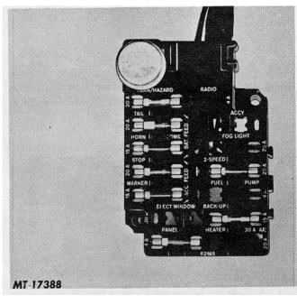
Figure 1 Fuse Panel (Typical)
