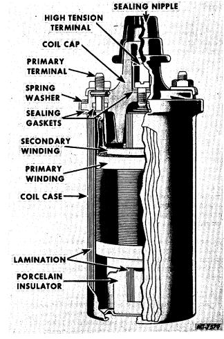
Fig. 1 Steel Encased Coil (Cutaway View)
