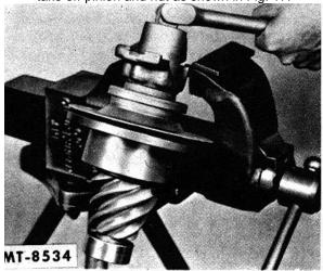
Fig. 17 Pinion and Cage Disassembly2. Tap or drive the pinion assembly from flange and out of cage using a soft hammer.
