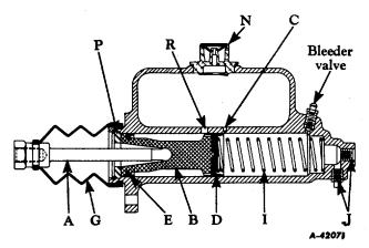
Fig. 2. Typical Master Cylinder with Bleeder Valve
