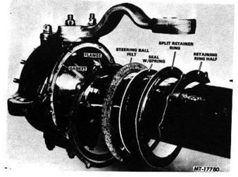
Fig. 4 Trunnion Housing Seals and Retainers
