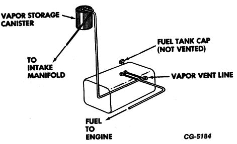
Fig. 22 CO-1610B and COF-1810B Cargostar Vehicles With 30 Gallon Right Fuel Tank
