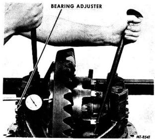
Fig. 31 Adjusting Differential Bearing Preload
