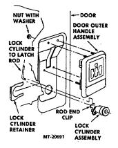
Fig. 23 Door Outer Handle and Lock Cylinder
