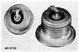
Fig. 8 Effects of Turbulence Burning
