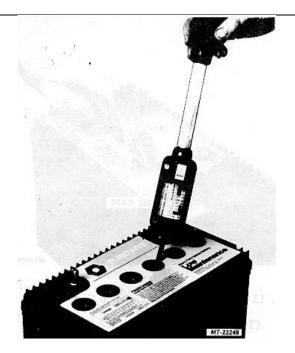
Fig. 12 Testing Specific Gravity
