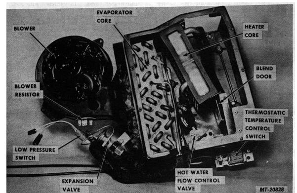
Fig. 3 Components of Combination Unit
