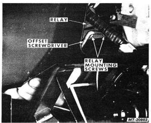
Fig. 52 Removing Relay
