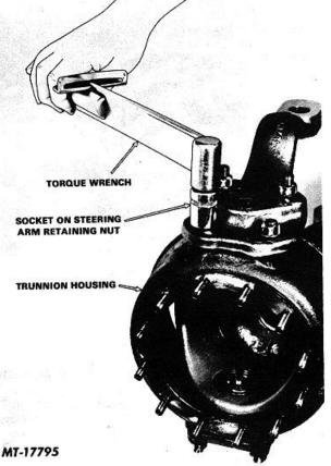
Fig. 20 Checking Bearing Adjustment
