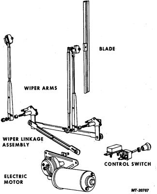
Fig. 1 Air Windshield Wiper Components
