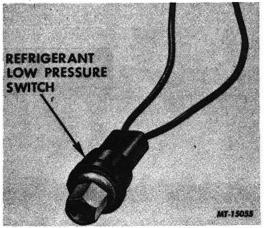
Fig. 13 Low Pressure Switch
