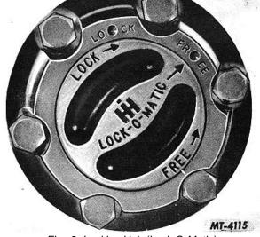
Fig. 2 Locking Hub (Lock-O-Matic)
