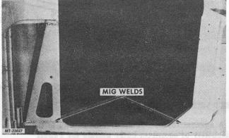
Fig. 38. Location of MIG Weld Seams
