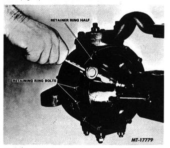
Fig. 3 Removing Retaining Ring Half (Halves) Mounting Bolts
