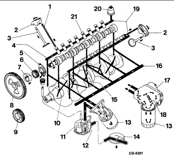
Fig. 5 Diagrammatic View of Lubricating System
