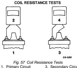
1. Primary Circuit3. Secondary Circuit2. Ohms X14. Ohms X1000
