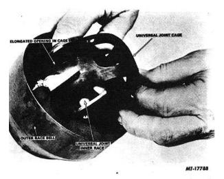
Fig. 12 Removing Cage and Inner Race
