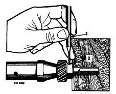
Fig. 18 Removing Distributor Driven Gear Pin
