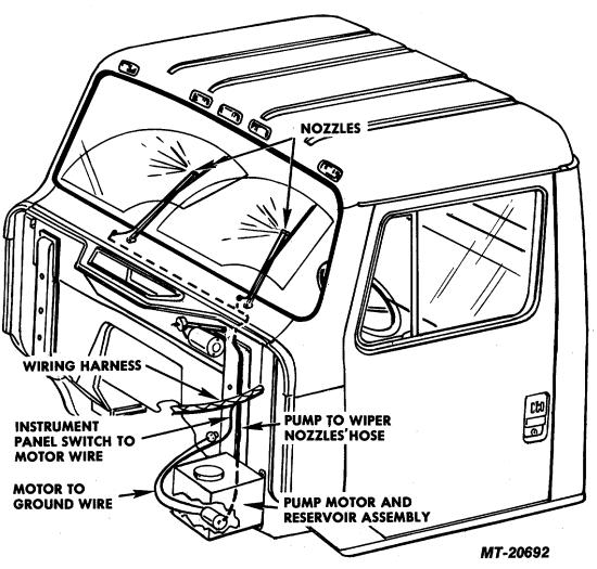
Fig. 1 Windshield Washer Installation (80" Wide Cab Shown)
