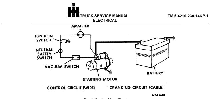
Fig. 3 Starting Motor Circuit
