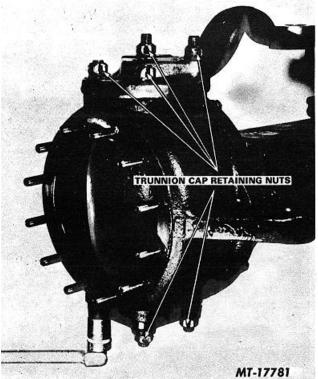
Fig. 5 Trunnion Cap Retaining Nuts
