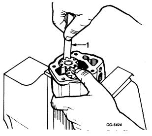
Fig. 131 Measure Pump Gear-to-Body Clearance
