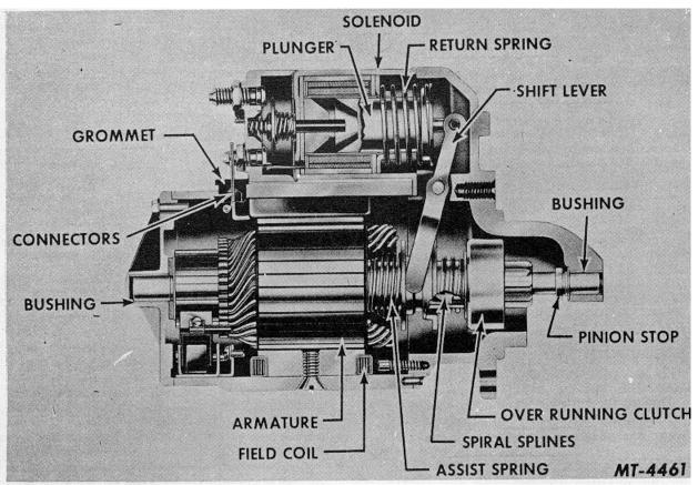
Fig. 1 Sectional View of Enclosed Shift Lever Type Starting Motor
