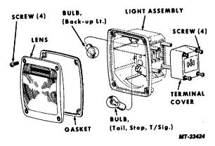
Fig. 16 Tail, Stop, Rear Turn Signal, Back-up Light
