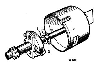
Fig. 21 Upper Thrust Washers (Distributors Without Tachometer Drive)
