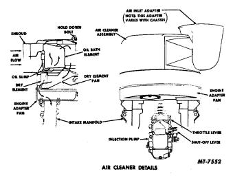
Fig. 8 Typical Combination Oil Bath And Dry Type Air Cleaner
