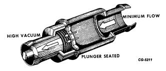
Fig. 46 Plunger Position During Idle or Low Engine Speed
