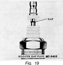
Prior to IH approval, the Booster Gap design was thoroughly tested and evaluated, at which time their antifouling characteristics were firmly established.
