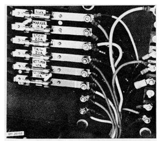
Fig. 14 Trailer Wiring Fuse Panel - S-Series Vehicles
