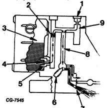
Figure 8 Idle System Fuel Air Flow Secondarv Side
