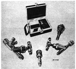
Fig. 25 High Vacuum Meter Kit (SE-2447)
