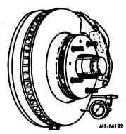
Fig. 15 Dial Indicator Installation
