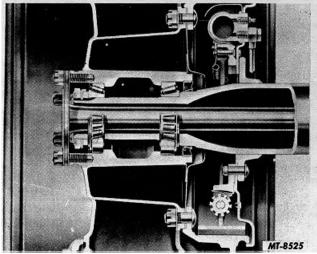
Fig. 4 Cross Section of Full-Floating Rear Axle
