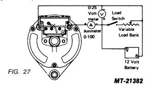
Before beginning the test and after the battery has been connected, momentarily flash the field by connecting a jumper between the diode trio terminal and the alternator positive output terminal (see Fig. 28). This will restore the residual magnetism which may have been weakened by handling or repair procedures.
