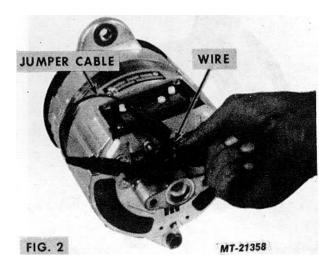
If the voltage fails to rise when performing this test, remove the regulator and carefully inspect it for a printed circuit track which has burned open. If this condition is found, replace the regulator. Check the brush spring caps and their contact screws for dirt or corrosion and clean if necessary. If the alternator does not operate after performing either or both of these operations, the alternator should be removed for repair or replacement.
