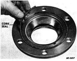
Fig. 19 Removing Pinion Cage Seal
