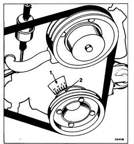
Fig. 45. Timing Marks (V-304, V-345, V392 Engines Shown) 1. Timing quadrant
