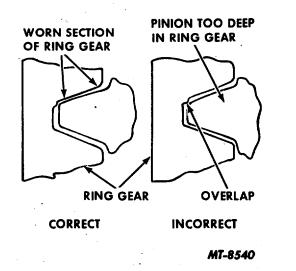
Fig. 30 Right and Wrong Adjustment of Ring Gear and Pinion When Worn Gears Are Reinstalled
