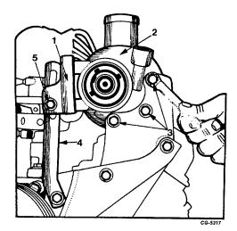
Fig. 24 Removing Power Steering Pump
