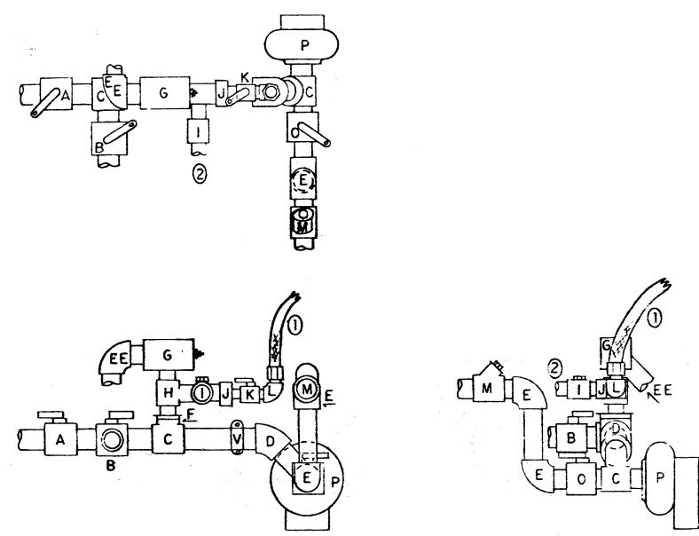
FIGURE 5 SUCTION SIDE OF PUMP INCLUDING RELIEF VALVE AN FOAM EDUCTOR
