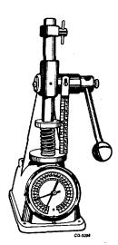
Fig. 104 Checking Spring Tension Using SE-2241 Tester
