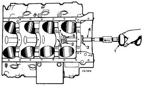
Fig. 81 Installing Second Bearing
