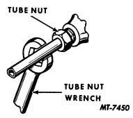
Fig. 2. Use of Tube Nut Wrench
