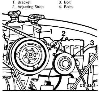
Fig. 15 Removing Freon Compressor V-Belt
