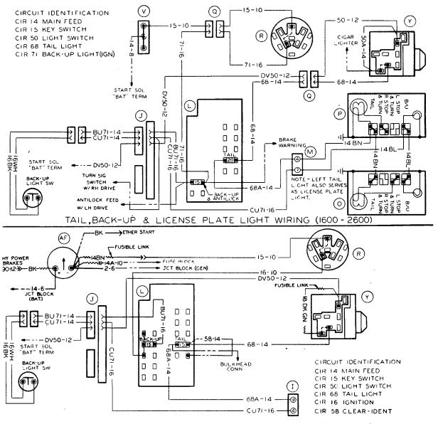
TAIL, BACK-UP & LICENSE PLATE LIGHT WIRING (FBC/BUS) MT-23293
