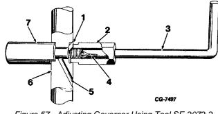
Figure 57. Adjusting Governor Using Tool SE-2072-2
