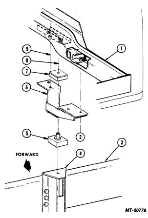
Fig. 55. Cab Rear Mounting (230 cm 90 inch Wide Cab)
