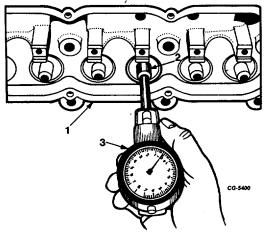
Fig. 106 Checking Guide Bore Using Gauge SE-2506
