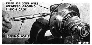
Fig. 22 Measuring Pinion Bearing Preload
