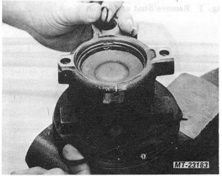
Fig. 4 Remove Housing and Union "O" Rings
