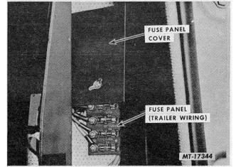
Figure 8 Trailer Wiring Fuse Panel 1900 Thru 2100 Fleetstar Vehicles
