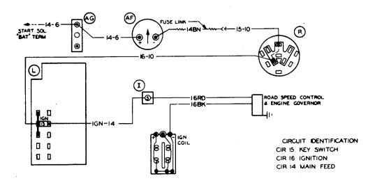
ROAD SPEED CONTROL 8 ENGINE GOVERNOR W/V-345, V-392 & MV8 ENGINES W/FBC/BUS
