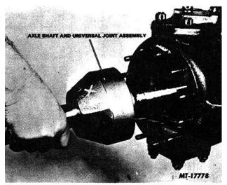
Fig. 22 Axle Shaft and Universal Joint Assembly
