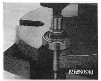
Fig. 21 Press Shaft Into Bearing
