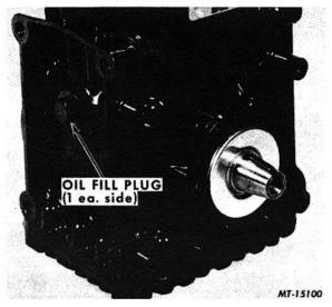
Fig. 36 Compressor Oil Fill Plug
