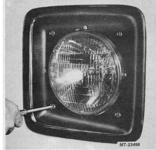
Fig. 3 Removing Headlight Bezel
