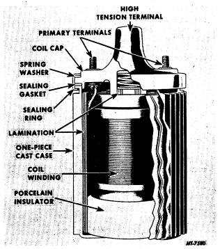
Fig. 2 Diecast Encased Heavy-Duty Coil (Cutaway View)
