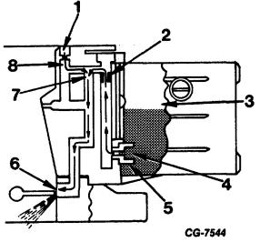
Figure 7 Idle System Fuel Air Flow Primary Side
