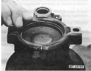
Fig. 6 Rotate Retaining Ring
