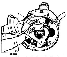
Fig. 12 Removing Diaphragm Rod Retainer
