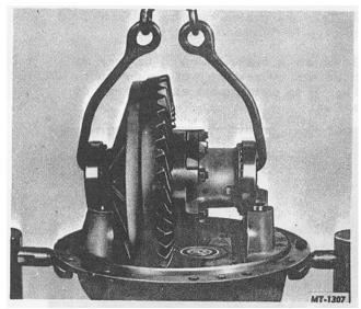
Fig. 2 Lifting Differential from Carrier
