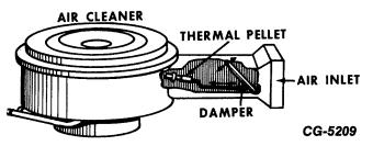
Fig. 44 Pellet Type Controlled Air Cleaner
