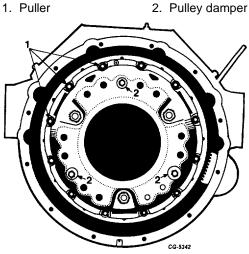
Fig. 49 Clutch Removal
