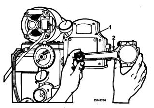
Fig. 93 Checking Connecting Rod Bushing Bore Using Precision Gauge Furnished with Honing Machine
