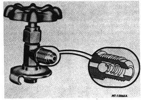
Fig. 31 Refrigerant Can Adapter (SE-2450)
