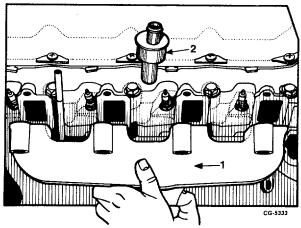
Fig. 40 Removing Right Exhaust Manifold
