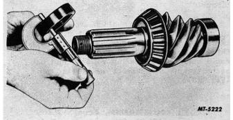
Fig. 12 Measuring Spacer Thickness
