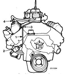
Fig. 31 Fuel Line Removal
