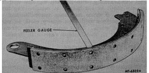
Fig. 13 Checking Tightness of Lining
