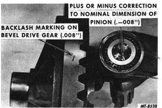
*Fig. 25 Location of Pinion Setting Markings* The procedure for establishing the correct nominal dimension by means of the pinion setting gauge is as follows:
