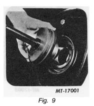
4. Hold tool handle firmly and strike until sound of impact changes when seal is seated (Fig. 10).
