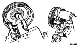
Fig. 7 Reconditioning Drum on Brake Drum Lathe
