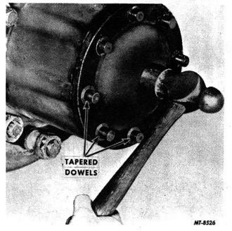
Fig. 6 Loosening Dowels in Axle Shaft
