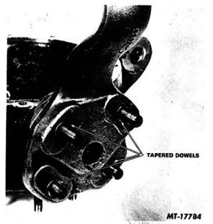
Fig. 8 Tapered Dowels
