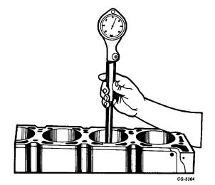
Fig. 71 Checking Cylinder Bore Using Dial bore Gauge SE-2331
