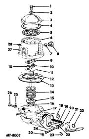
Fig. 4 Exploded View Screen Filter Type Fuel Pump
