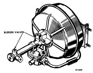
Fig. 4. Vacuum Power Cylinder RESIDUAL CHECK VALVE
