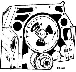
Fig. 61 Thrust Flange Bolt Removal
