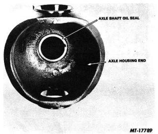
Fig. 13 Axle Shaft Oil Seal
