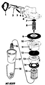
Fig. 5 Exploded View of Suspended Bowl Type Fuel Pump
