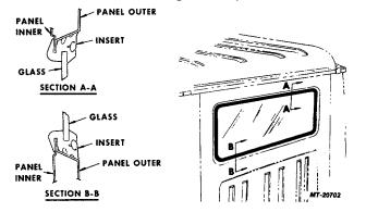
Fig. 34. Cab Rear Window Glass and Weatherseal
