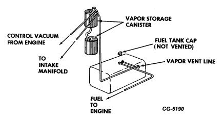
Fig. 28 CO-1610B and COF-1910OB Cargostar Vehicles With 50 Gallon Right Fuel Tank
