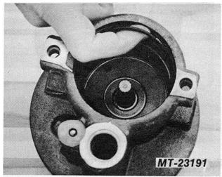
Fig. 12 Remove Pressure Plate "O" Ring
