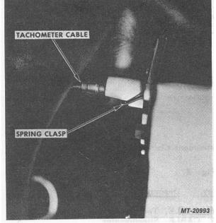
Fig. 4 Releasing Speedometer and Tachometer Cable
