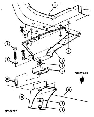
Fig. 53. Cab Front Mounting Bracket (Left Front View)
