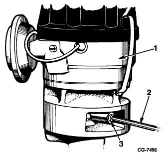
Fig. 56. Using Allen Wrench to Remove Governor Plug 1. Distributor 2. Allen Wrench 3. Governor Plug
