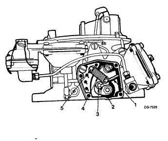
1. Diaphragm Rod4. Governor Spring2. Governor Lever5. Governor Spring Post3. Rod Retainer
