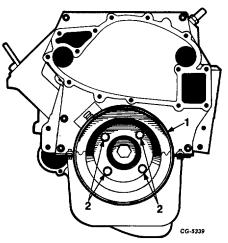
Fig. 46 Crankshaft Pulley Removal
