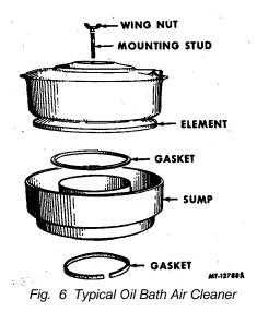
portion of the unit and then downward at high velocity. Just above the oil reservoir, in the bottom of the cleaner, the direction of air travel is suddenly reversed. This reversal of air flow causes the larger particles of dirt to fall into the oil. The partially cleaned air then travels upward through an oil moistened filtering element where any remaining dirt and dust particles are removed. The cleaned air then enters the carburetor.
