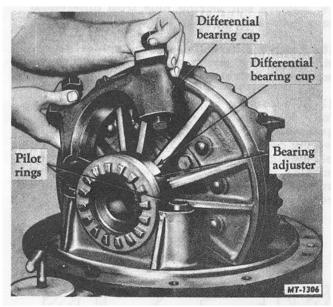
Fig. 1 Removing Differential Bearing Caps
