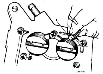
Figure 51 Checking Throttle Plate Clearance 1. Specified Drill or Gauge Size
