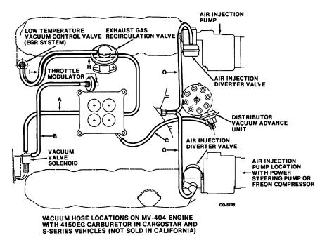
Fig. 79 Vacuum Hose Location on MV-404 Engine With 4150 EG Carburetor in Cargostar and S-Series Vehicles. (Sold in USA Except California)
