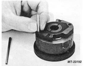
Fig. 13 Remove Dowel Pins
