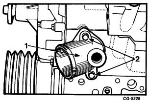
Fig. 35. Water Inlet Housing Removal
