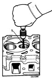
Fig. 105 Valve Guide Cleaning Tool **1. Cleaning tool**
