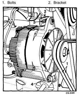
Fig. 13 Removing Alternator V-Belts
