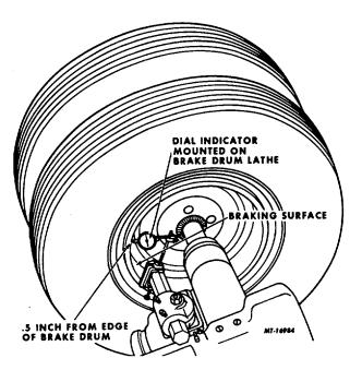
Fig 5 Checking Drum Runout on Brake Drum Lathe
