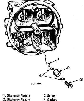
Figure 43 Installing Pump Discharge Needle
