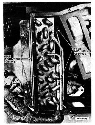
Fig. 47 Evaporator Core Mounting Screws
