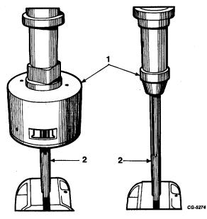
Fig. 33 Burnishing Upper and Lower Bushings Using Burnisher Tool.1. Housing 2. Burnisher
