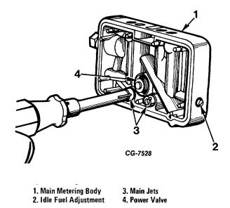
Figure 31 Using Jet Wrench SE-1772-6 to Remove Main Jets
