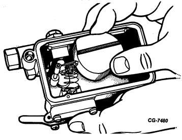
Figure 33 Removing Float and Hinge Assembly
