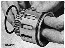
Fig. 15. Removing Spirolox Lock Ring
