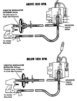
THROTTLE MODULATOR OPERATION cg-5214 Fig. 60 Throttle Modulator Operation
