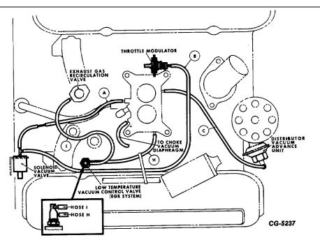
Fig. 90 Vacuum Hose Locations on V-345 Engine With 2210C Carburetor in Cargostar and S-Series Vehicles (Sold in Canada)
