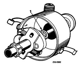
Fig. 22 Upper Thrust Washer (Distributors With Tachometer Drive)
