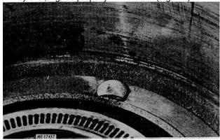
Fig. 22 Drum Bolt Alignment
