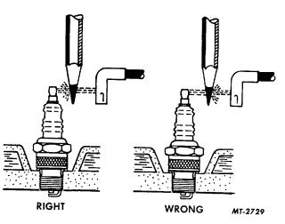
Fig. 6 Method of Checking for Reversed Polarity
