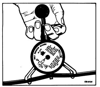
Fig. 156 Testing Alternator Belts Using SE-2312 Gauge
