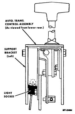
Fig. 20 Automatic Transmission Control Light
