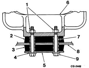
Fig. 6 Engine Front Mounting with Two-Piece Insulator
