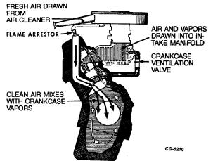
Fig. 45 Typical Air and Vapor Flow Through the System
