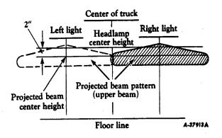
Fig. 1 Headlight Aiming Pattern
