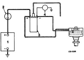
Fig. 51 Testing Voltage at Coil Negative (-) Terminal
