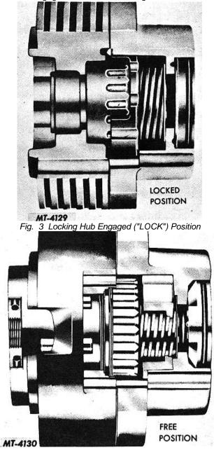
Fig. 4 Locking Hub Disengaged ("FREE") Position
