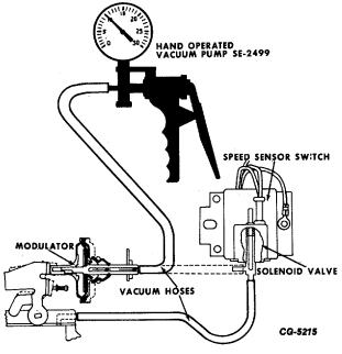
Fig. 61 Modulator Test
