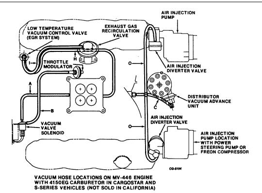
Fig. 80 Vacuum Hose Locations on MV-446 Engine With 4150 EG Carburetor in Cargostar and S-Series Vehicles (Sold in USA Except California)
