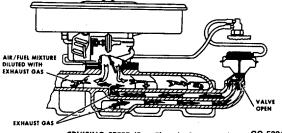
CRUISING SPEED (Part Throttle Operation) CG-5224 Fig. 56 Exhaust Gas Recirculation System
