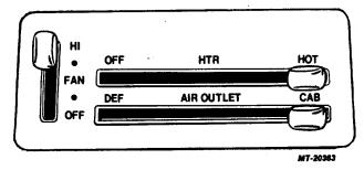
Fig. 19 Heater Controls Set for Maximum Heat
