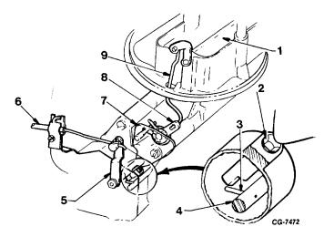
Figure 16 Manual Choke System
