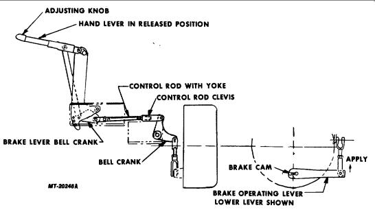
Fig. 2 Parking Brake Adjustment in the Orscheln Hand Lever
