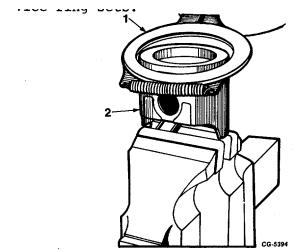
Fig. 101 Installing Piston Ring Using Suitable Piston Ring Expander Tool
