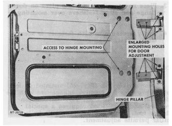
Fig. 27. Location for Door Adjustments at Hinge Pillar
