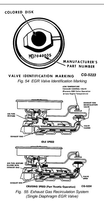
The EGR valve regulates the amount of exhaust gas entering the intake manifold. The EGR valve is controlled by ported vacuum, which is determined by position of the carburetor throttle plate(s). Operation of the exhaust gas circulation system is illustrated in Figures 55 and 56.
