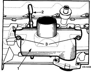
Fig. 39 Head Shroud Removal
