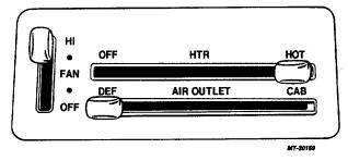
Fig. 20 Heater Controls Set for Defrosting
