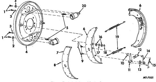
Fig. 3 Exploded view of Brake Group
