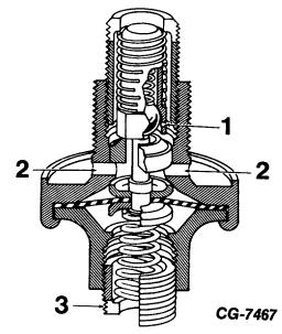
Figure 11 Two-Stage Power Valve
