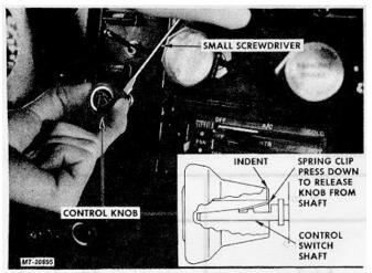
Fig. 6 Removing Control Knob from Switch
