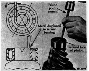
Fig. 9 Staking Pinion Straddle Bearing
