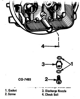
Figure 44 Installing Pump Discharge Check Ball
