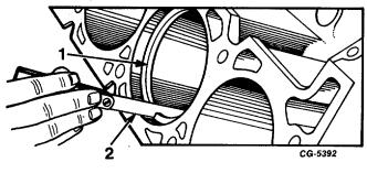
Fig. 99 Checking Ring Gap
