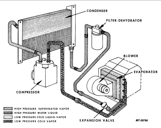
Fig. 18 Refrigerant Flow Through Air Conditioning System
