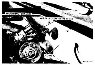
Fig. 5 Removing Windshield Wiper Motor
