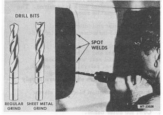
Fig. 37. Removing Cab Inner Corner Panel
