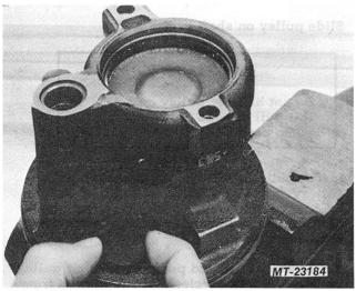
Fig. 5 Remove Magnet
