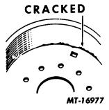
Fig 6 Cracked Drum
