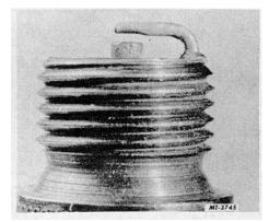
Fig. 15 Reversed Coil Polarity
