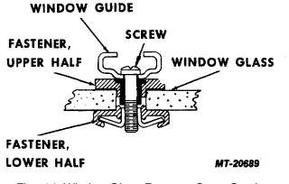
Fig. 14 Window Glass Fastener Cross Section
