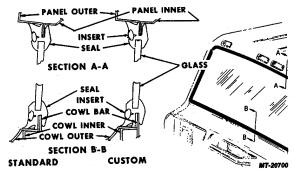
Fig. 32. Windshield Weatherseal (Retainer)
