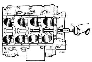
Fig. 82 Removing Front Bearing
