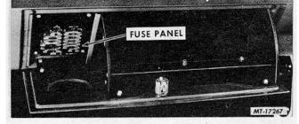
Figure 5 Fuse Panel Location 100, 150, 200, 500 and 1600 Thru 1850 Loadstar Vehicles
