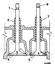
Fig. 114 Sectional View of Valves
