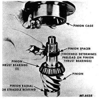
Fig. 18 Removing Pinion Bearing Spacer
