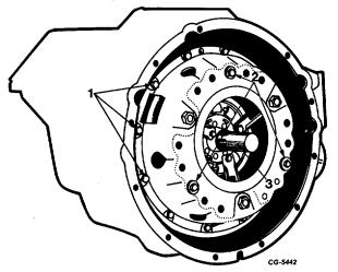
Fig. 150 Clutch Installation to Flywheel
