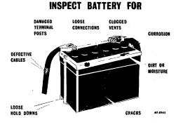
Fig. 8 Battery Maintenance Inspection
