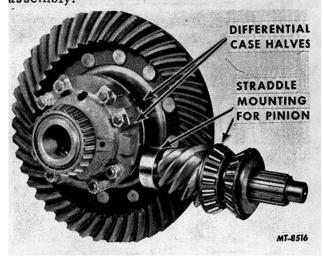
Fig. 1 Differential Assembly
