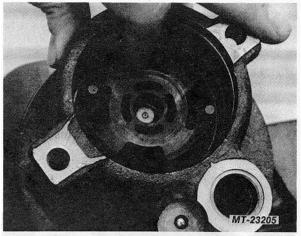
Fig. 26 Install Thrust Plate
