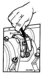
Fig. 129 Checking Connecting Rod End Clearance
