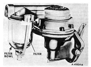
Fig. 1 Mechanical Fuel Pump (Side Mounted Bowl Type)
