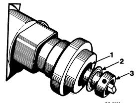
**cg-5261** Fig. 20 Lower Thrust Washer (Distributor for V-537 Engine)
