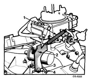
Fig. 29 Removing Return Spring and Bracket
