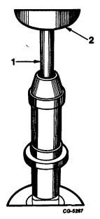
Fig. 26 Pressing Out Upper Bushing Using Knock-Out Bar
