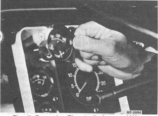
Fig. 7 Removing Electrically Actuated Water Temperature Gauge
