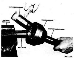
Fig. 10 Axle Shaft and Universal Joint Disassembly
