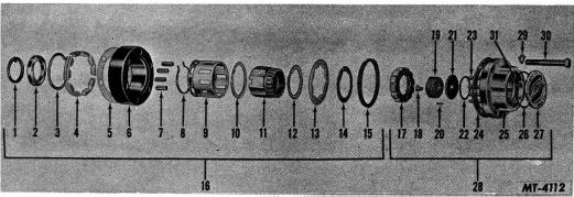
Fig. 12. Locking Hub (Lock-O-Matic) (Exploded View)
