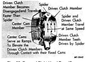
Fig. 39. Forward Right-Hand Turn (Cross Sectional View)
