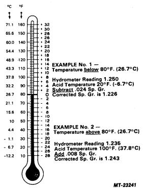
Fig. 7 Specific Gravity Temperature Correction Values
