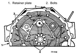
Fig. 55 Flywheel Housing Removal
