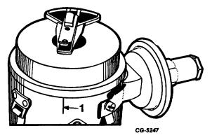
Fig. 6 Rotor Position Reference Mark
