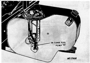
Fig. 3 Cutaway View of a Fuel Tank with an Electric In-Tank Mounted Fuel Pump
