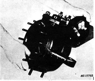
Fig. 7 Removing Trunnion Housing
