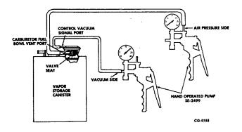
Fig. 16 Canister Fuel Bowl Vent Control Valve Seat Test
