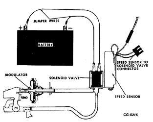
Fig. 62 Jumper Wires from Battery to Solenoid Valve Terminals
