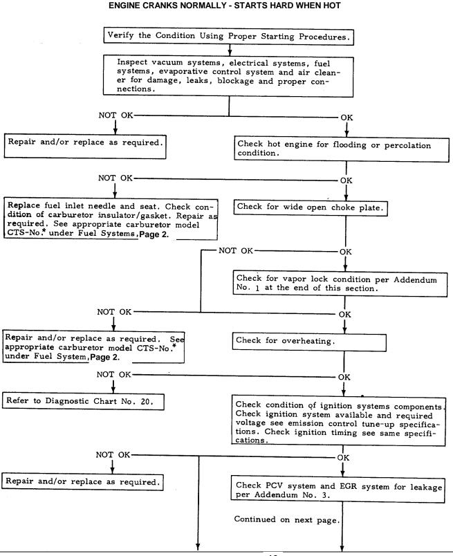
CHART NO. 05 ENGINE CRANKS NORMALLY - STARTS HARD WHEN HOT
