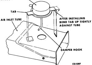
Fig. 42 Vacuum Chamber Details
