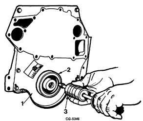
Fig. 53 Front Cover Oil Seal Removal with Cover Installed. Using SE-2091 Puller
