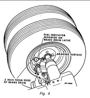
emery or steel wool particles from drum after this operation. More heavily damaged or out-of-round drums should be ground or turned on brake drum lathe.
