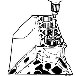
Fig. 76 Honing cylinder bore Using SE-784 Cylinder Grinder
