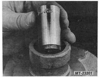
Fig. 22 Install New Pump Seal
