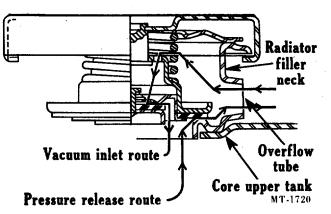
Fig. 1 Radiator Cap (Pressure Type)
