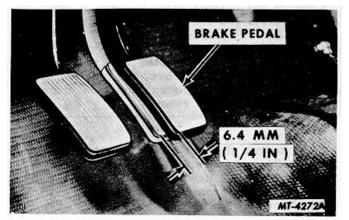
Fig. 1. Brake Pedal Free Travel
