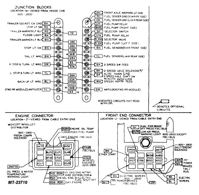
Component And Major Connectors Junction Blocks - Engine Connector - Front End Connector
