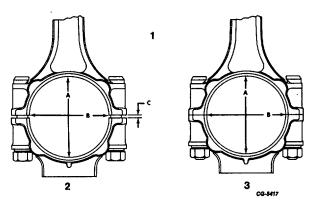
Fig. 124 Illustrating Bearing Crush
