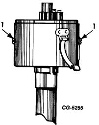
Fig. 14 Distributor Plate Mounting Screw
