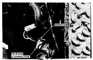
Fig. 39 Blower Resistor Removal
