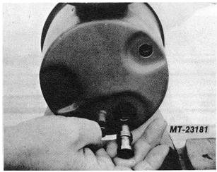
Fig. 2 Remove Flow Control Valve and Spring
