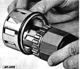
Fig. 16. Separating Axle Shaft Hub from Roller Cage
