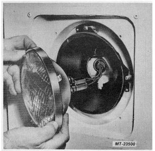
Fig. 5 Removing Sealed Beam Unit
