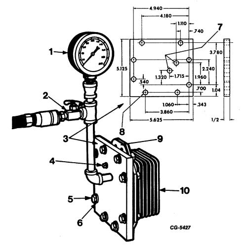
Fig. 134 Pressure Testing Engine Oil Cooler Core Assembly
