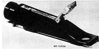
Fig. 10 SE-2395 Antifreeze and Battery Tester **TROUBLE SHOOTING**
