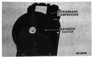
Fig. 7 Magnetic Clutch
