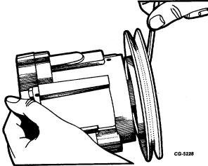
Fig. 67 Installing Centrifugal Air Filter Fan
