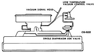
Fig. 53 Single Diaphragm EGR Valve System
