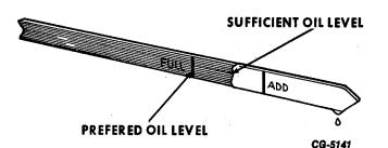
Fig. 2 Proper Oil Level
