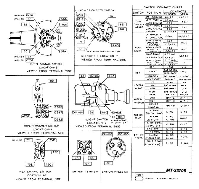
Component And Major Connectors (Not Schoolbus) Turn Signal Switch - Key Switch - Windshield Wiper/Washer Switch Light Switch - Heater/Air Conditioner Switch - Shut Down Temperature Switch Shutdown Pressure Switch
