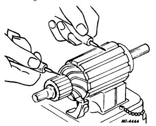
Fig. 9 Testing Armature for Grounds
