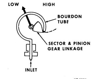
MT-8890 Fig. 23 Air Pressure Gauge Details
