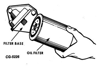
Fig. 1 Typical Spin-On Type Oil Filter
