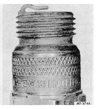
Fig. 16 Damage to Spark Plug from Pressure (Plier) Type Gap Tools
