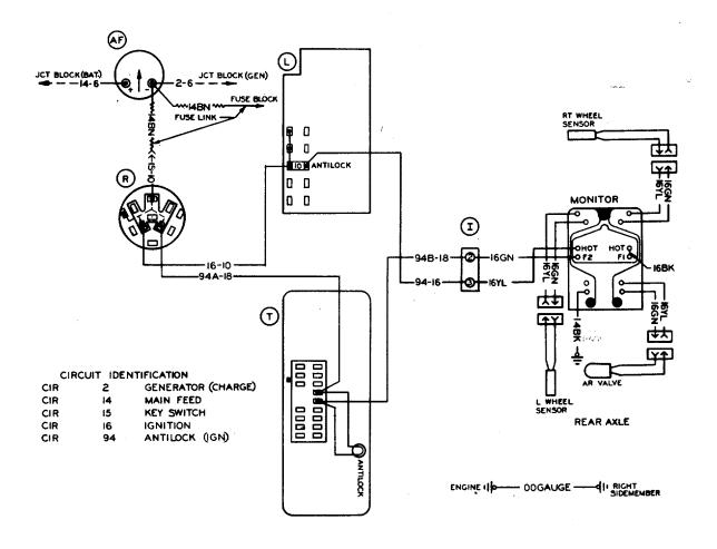
AIR BRAKES ANTILOCK WIRING FBC/BUS
