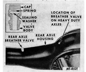
Fig. 2 Location of Breather Valve in Axle Housing
