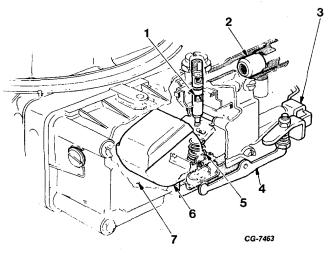
Figure 6 Typical Fuel Inlet System
