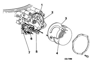
Figure 58. Automatic Choke Assembly
