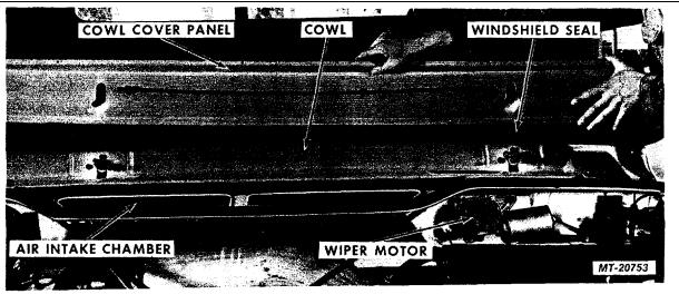
Fig. 3 Removing Cowl Cover Panel
