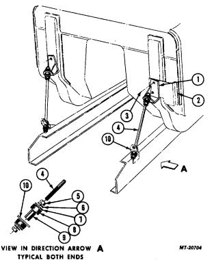
Fig. 56. Stay Rod Details for 200 x 280 cm (80 x 112 inch) Cab
