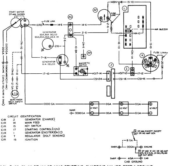
D 9.0L, D-150, 170, 190, DT-466 OR 3208 STARTING, CHARGING, MAJOR FEED & GROUND WIRING FBC/BUS
