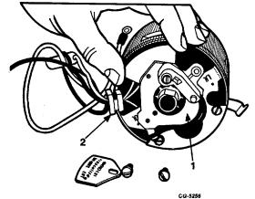
Fig. 15 Removing Electronic Control Unit
