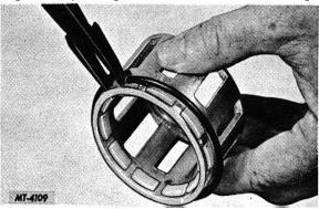
Fig. 17. Removing Friction Shoes and Spring
