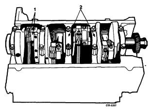
Fig. 58 Positioning Connecting Rods for Removal
