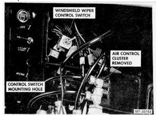
Fig. 7 Removing Wiper Switch from Instrument Panel
