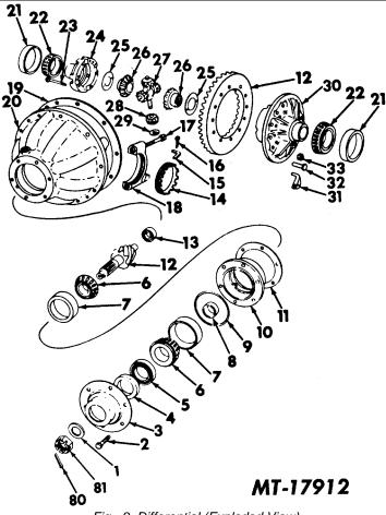
Fig. 8 Differential (Exploded View)
