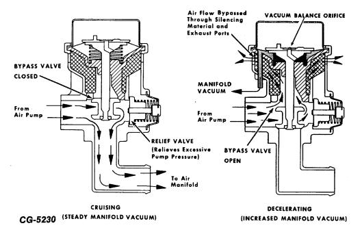
Fig. 69 Typical Diverter Valve Operation
