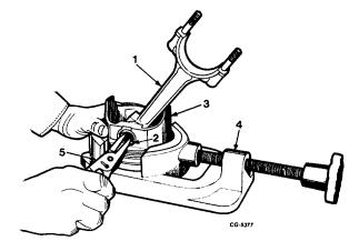
Fig. 84 Removing Piston Pin Retainers
