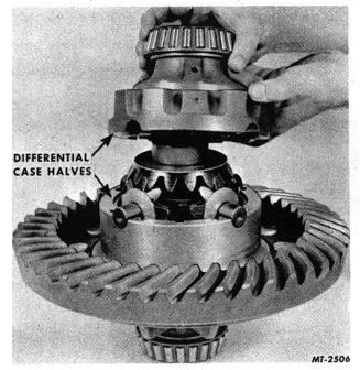
Fig. 13 Separating Differential Case Halves
