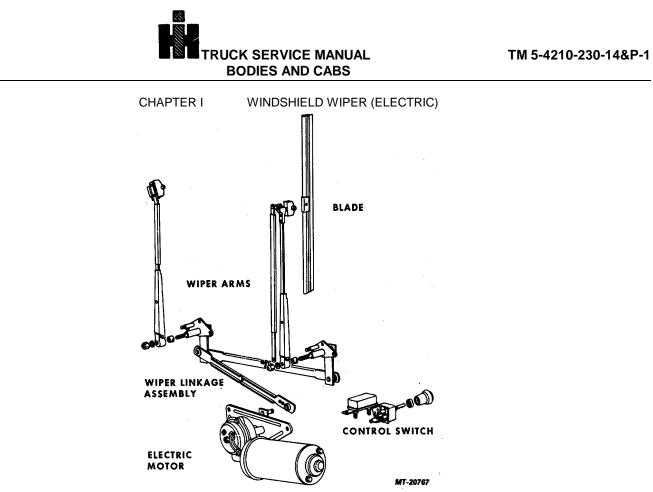
Fig. 1 Electric Windshield Wiper components
