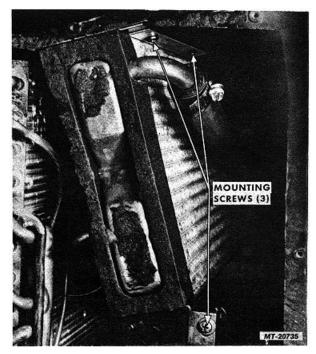
Fig. 51 Heater Core Mounting Screws
