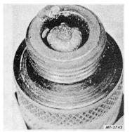
Fig. 12 Sustained Preignition Damage
