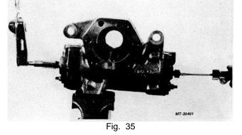
With rack piston (31) near center of steering gear travel, screw adjusting screw (39) into solid height.
