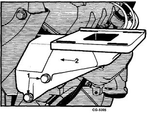
Fig. 12 Removing Air Compressor Bracket
