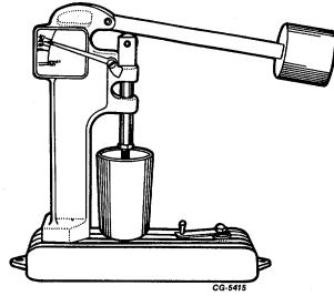
Fig. 122 SE-1893 Tester Used for Checking Leakdown Rate of Tappet
