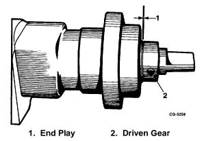
Fig. 17 Checking Distributor Shaft End Play (Thrust Washerto-Thrust Collar Clearance) (Typical)
