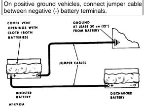
Fig. 9 Proper Jumper Cable Connections (Negative Ground Vehicles Shown
