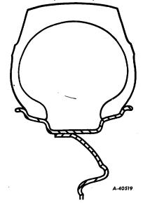
Fig. 4. Dual Cast Wheel and One Piece Rim (Tubeless)
