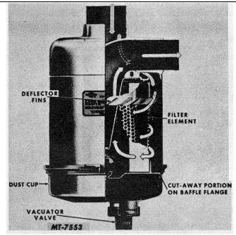
Fig. 3 Typical Dry Type Air Cleaner
