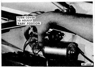
Fig. 8 Adjusting Wiper Blade Park Position
