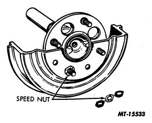
Fig. 20 Threaded Fastener Type Drum Mounting
