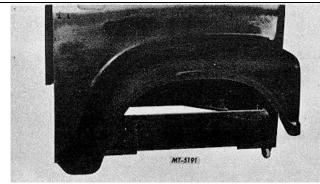
Fig. 13 Repaired Hood and Fender Assembly.
