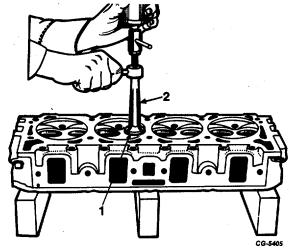
Fig. 111 Pulling Exhaust Valve Insert with SE-1951 Remover
