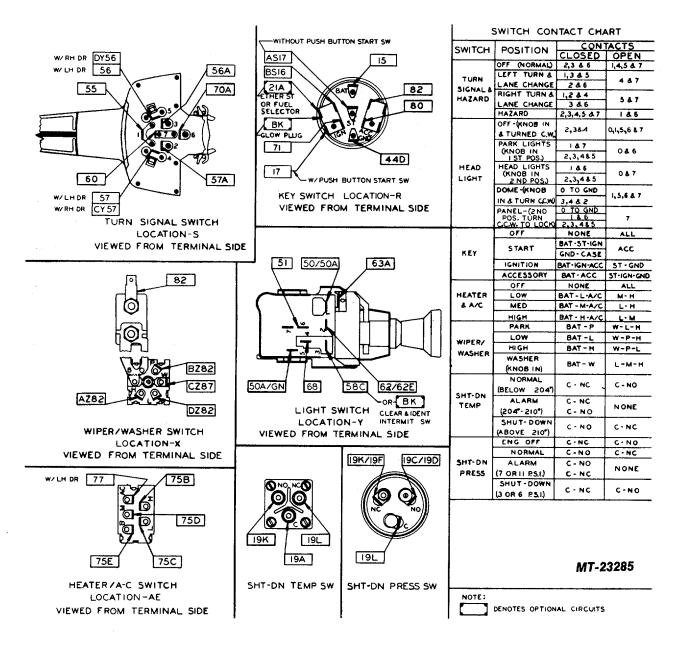
Turn Signal Switch - Key Switch - Windshield Wiper/Washer Switch
