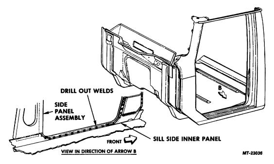
Fig. 47. Side Panel To Sill Side Inner Panel Spot Welds
