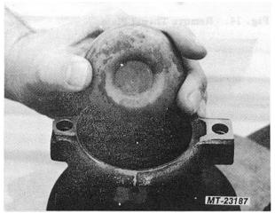
Fig. 8 Remove End Plate
