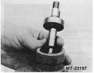
Fig. 18 Remove Shaft Assembly
