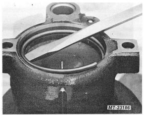
Fig. 7 Remove Retaining Ring
