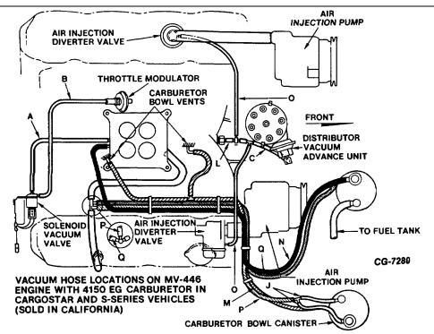
Fig. 86 Vacuum Hose Location on MV-446 Engine With 4150 EG Carburetor in Cargostar and S-Series
