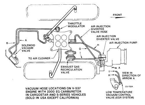
Fig. 81 Vacuum Hose Locations on V-537 Engine With 2300 EG Carburetor in Cargostar and S-Series Vehicles (Sold in USA Except California)
