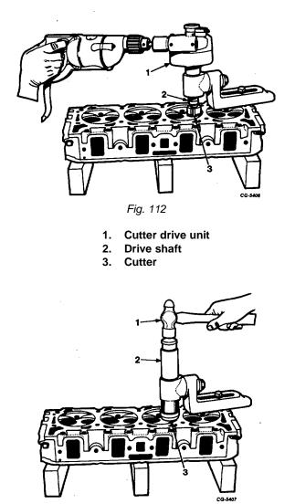
Fig. 113 Using Insert Installer from Counterbore Tool Set SE-1797 for Installing Inserts in Cylinder Head
