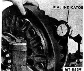
Fig. 29 Using Dial Indicator to Set Correct Backlash
