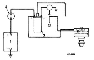
Fig. 53 Testing With Brown Wire Removed1. Battery3. Ignition Coil2. Ignition Switch4. Voltmeter
