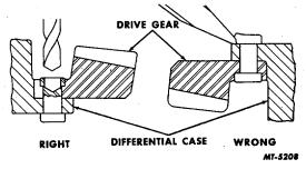
Fig. 15 Drive Gear Rivet Removal
