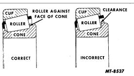
Fig. 21 Roller Bearing When Correct Adjustment is Obtained. (The rollers of the bearing must bear against the face of the cone as shown. Rotation of the bearing during adjustment is necessary to obtain this condition.)
