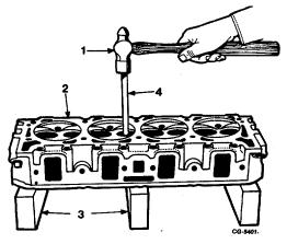
Fig. 107 Removing Valve Guides with SE-1722
