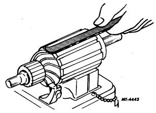
Fig. 8 Testing Armature for Short Circuits
