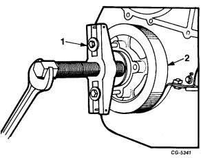
Fig. 48 Using SE-1368 Puller to Pull Crankshaft Damper
