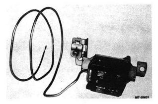
Fig. 12 Thermostatic Temperature Control Switch
