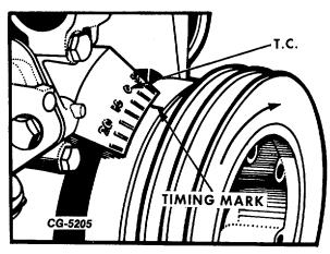
Fig. 40 Typical Location of Timing Marks
