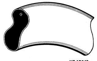
**MT-17542** Fig. 20 Damage Caused by Dirt In Tire
