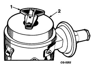
Fig. 11 Distributor Rotor and dielectric Shield (Dust Cover).
