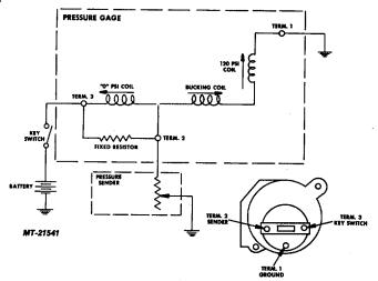
Fig. 21 Oil Pressure Gauge Circuit Diagram
