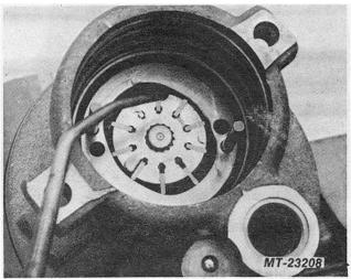
Fig. 29 Lubricate Rotating Group
