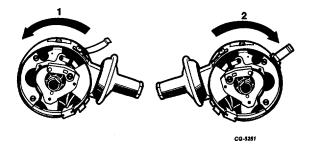
Fig. 10 Illustrating Vacuum Diaphragm Location and Distributor Rotation
