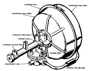
Fig. 3. Vacuum Power Cylinder
