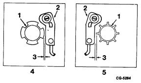
Fig. 49 Trigger Wheel-to-Sensor Air Gap 1. Trigger Wheel 4. 4 Cylinder Engine 2. Sensor
