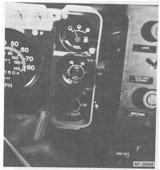
Fig. 9 Removing Air Gauges
