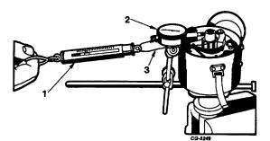
Fig. 8 Shaft and Bushing Wear Test (Checking Distributor Shaft Side Play)
