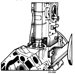
Fig. 75 Reboring Cylinder Using SE-1399 Boring Machine
