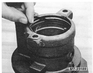
Fig. 10 Remove End Plate "O" Ring
