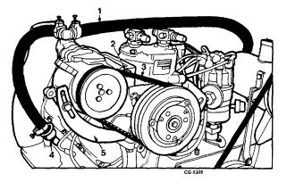
Fig. 16 Air Pump Removal
