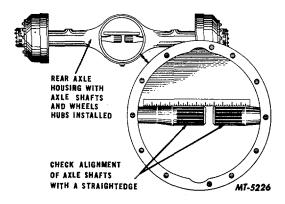
Fig. 5 Method of Checking For Bent Axle Housing
