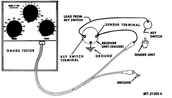
Fig. 19 Checking Fuel Level Gauge System with Gauge Tester
