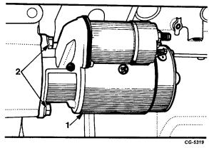
Fig. 26 Starting Motor Removal
