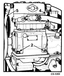
Fig. 11 Air Compressor Removal
