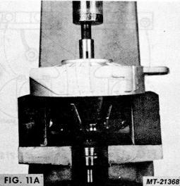
Remove four screws and bearing retainer and press 17 bearing out of drive end housing (see Fig. 12).
