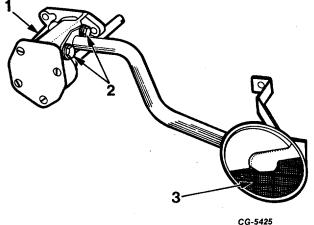
Fig. 132 Oil Pump and Screen Assembly 1. Oil pump 2. Bolts 3. Screen assembly
