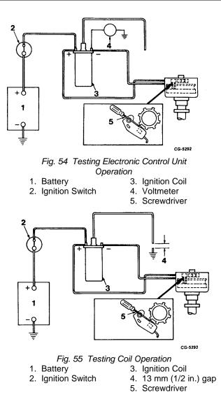
With ignition switch "on" observe for spark across gap each time screwdriver blade is placed against face of sensor.
