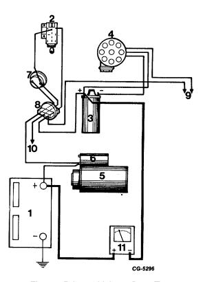
Fig. 58 Primary Voltage Drop Test 7. Ammeter
