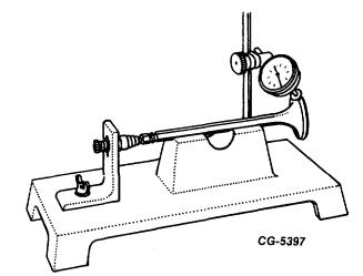
Fig. 103 Checking Valve Stem Straightness and Face Run-Out
