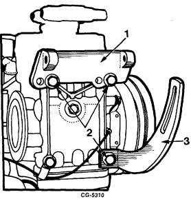
Fig. 17 Removing Air Pump Brackets
