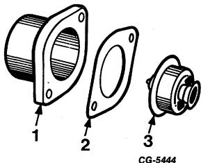
Fig. 152 Exploded View of Thermostat, Gasket and Engine Water Outlet
