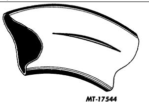
Fig. 22 Crease or Fold Result of Innertube Being Too Large for Tire Pinched Innertube:
