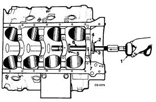
Fig. 83 Installing Front Bearing
