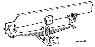
Fig. 1 Front Axle Application (Constant Rate)
