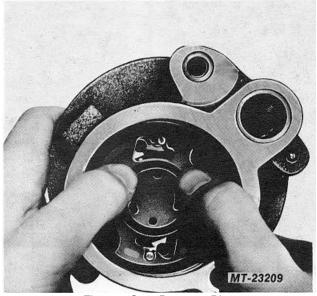
Fig. 30 Seat Pressure Plate
