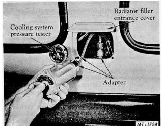
Fig. 7 Using SE-1870 Cooling System Pressure Tester with Adapter
