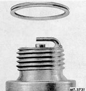
Fig. 1 Not Properly Tightened (Gasket Not Compressed)
