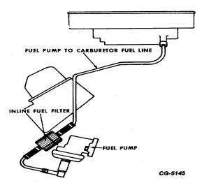
Fig. 6 Inline Fuel Filter Typical on Most Gasoline Engines
