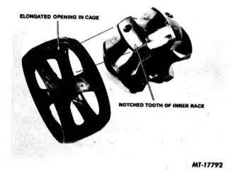
Fig. 16 Assembling Inner Race and Cage
