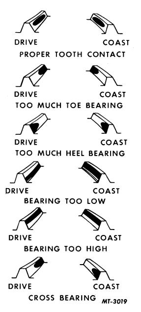
Fig. 33 Location, Size and Shape of Correct Tooth Contacts
