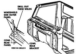
Fig. 44. Windshield Side Outer Panel to Cowl Rear Panel and Bracket Spot Welds
