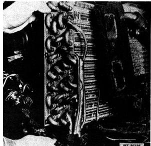
Fig. 48 Removing Evaporator Core
