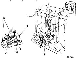
Figure 10 Power Enrichment Fuel Air Flow
