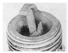
Fig. 14 Results of Mechanical Damage
