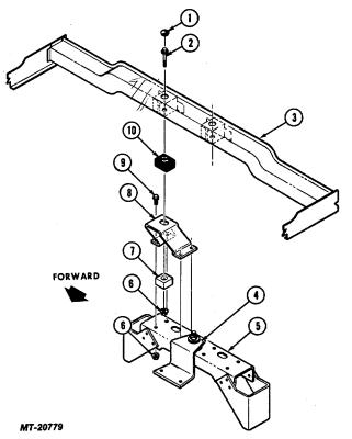
Fig. 54. Cab Rear Mounting (200 cm 80 Inch Wide Cab)
