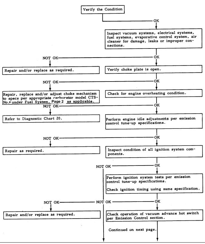
CHART NO. 11 ENGINE STALLS AT IDLE - ENGINE HOT
