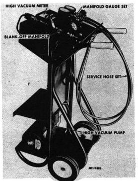
Fig. 32 Portable Air Conditioning Service Station (SE-2443)
