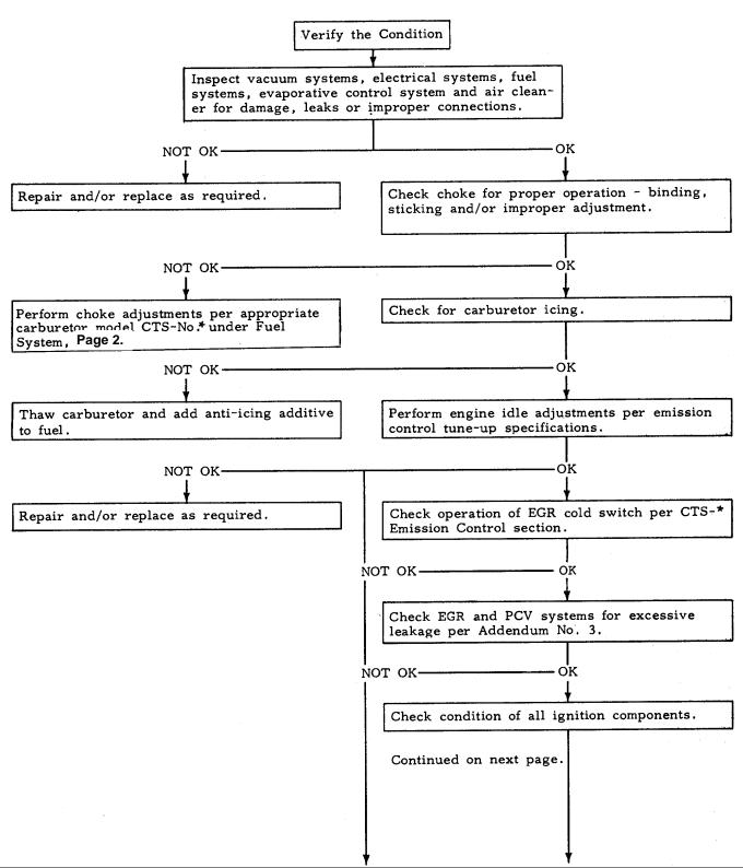
CHART NO. 10 ENGINE STALLS AT IDLE - ENGINE COLD
