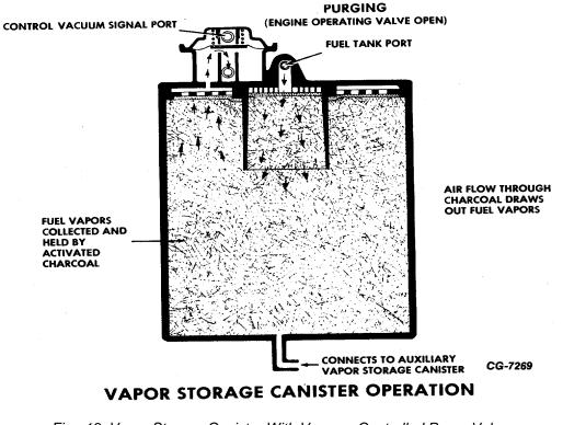
Fig. 13 Vapor Storage Canister With Vacuum Controlled Purge Valve
