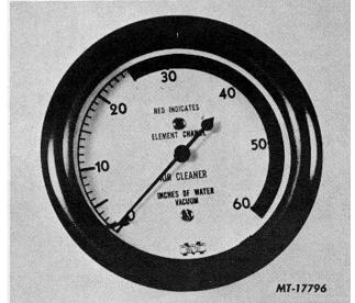
Fig. 10 Air Cleaner Restriction Gauge
