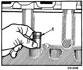
Fig. 43 Hydraulic Tappet Removal
