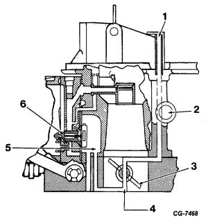
Figure 12 Modulator Valve in Open Position Power Valve Open
