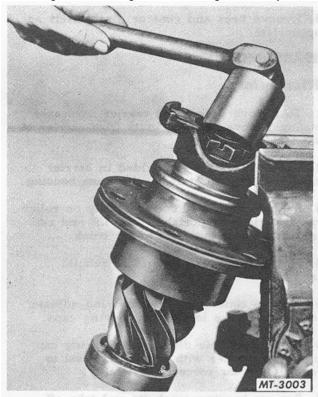
Fig. 6 Removing Pinion End Nut
