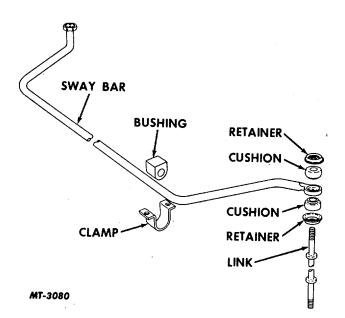
Fig. 7 Front Sway Bar
