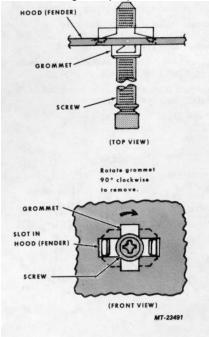
Fig. 8 Adjusting Screw Mounting Details
