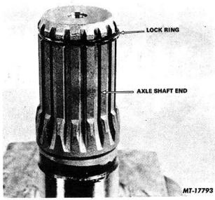
Fig. 18 Axle Shaft Lock Ring
