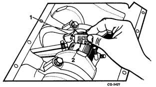
Fig. 128 Checking Connecting Rod Bearing Clearance
