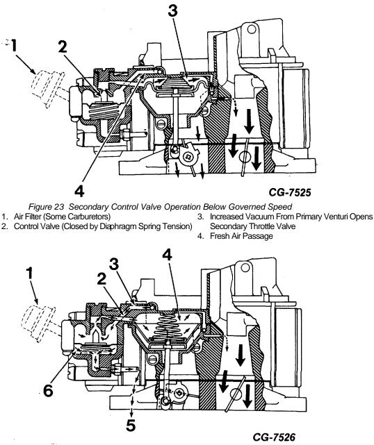
Figure 24 Secondary Control Valve Operation at Governed Speed
