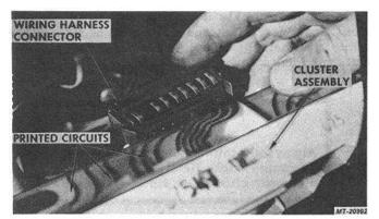
Fig. 3 Removing Wiring Harness Connector
