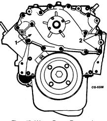
Fig. 45 Water Pump Removal
