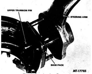
Fig. 9 Steering Arm Removal
