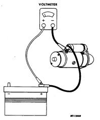
Fig. 4 Cranking Circuit Test
