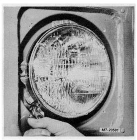
Fig. 6 Disconnecting Headlight Retainer Spring
