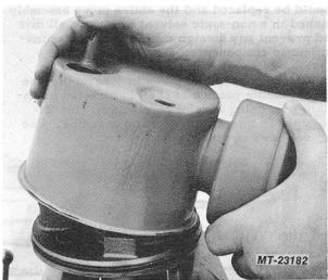
Fig. 3 Remove Reservoir
