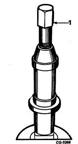
Fig. 27 Bushing Remover SE-1955-5 Installed in Lower Bushing 1. Remover
