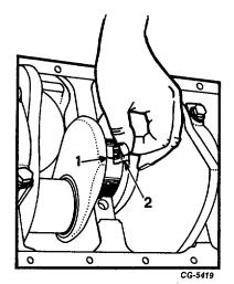
Fig. 126 Checking Main Bearing Clearance
