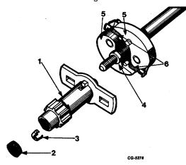
Fig. 37 Mechanical Advance System Components
