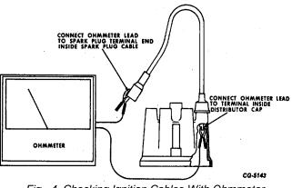
Fig. 4 Checking Ignition Cables With Ohmmeter
