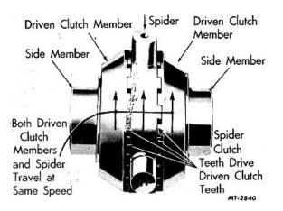
Fig. 37 Straight Forward Driving
