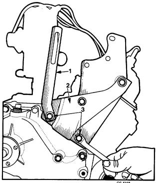
Fig. 25 Removing Power Steering Bracket and Strap
