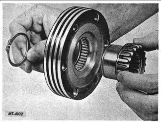
Fig. 7. Removing Axle Shaft Hub
