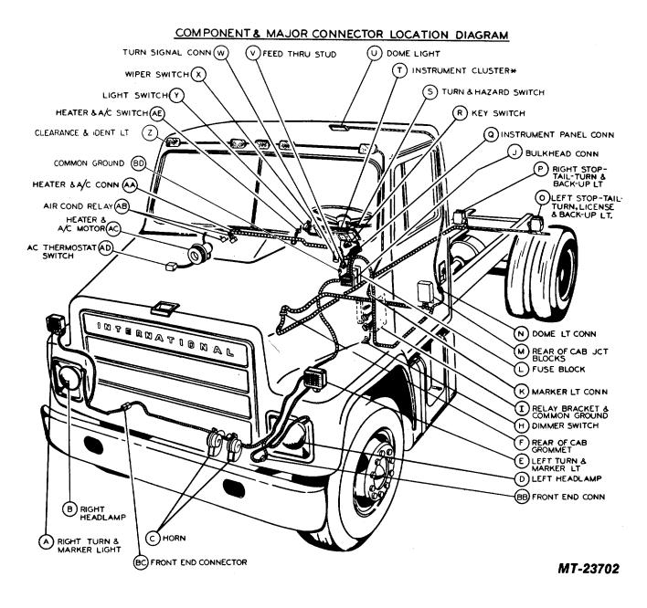
Component And Major Connector Location (On Chassis) 1600 thru 1900 Models
