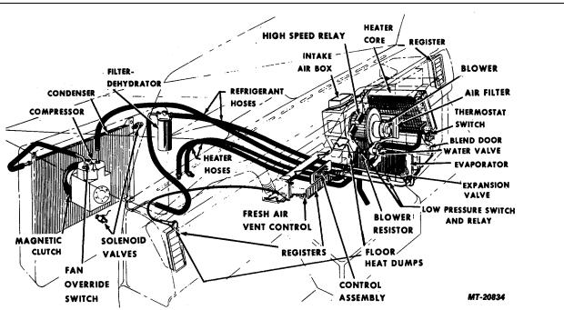
Fig. 1. Comfort Control Heating and Air Conditioning System
