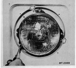
Fig. 4 Removing Sealed Beam Unit Retaining Ring
