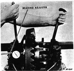
Fig. 18 Adjusting Bearing Preload
