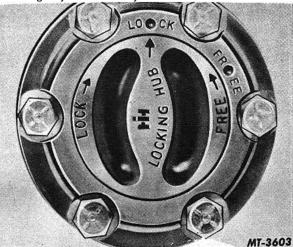
Fig. 1 Locking Hub (Manual Type)
