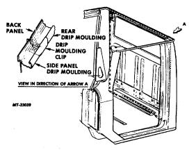
Fig. 50. Securing Drip Moulding Clip
