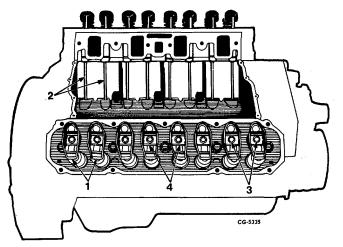
Fig. 42 Rocker Arm Removal
