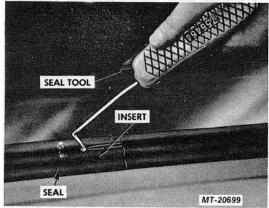
Fig. 31. Removing Windshield Weatherseal Insert
