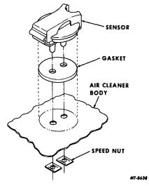
Fig. 12 Temperature Sensor Replacement
