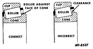
Fig. 10 Pinion Bearing Roller Position
