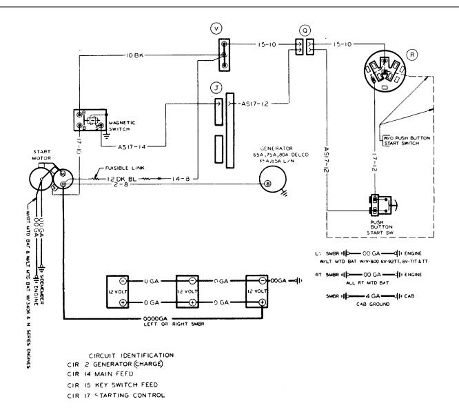
6V-92TT.8V-7IT&TT.800,3406&N-SERIES STARTING,CHARGING & MAJOR FEED & GROUND WIRING MT-23744
