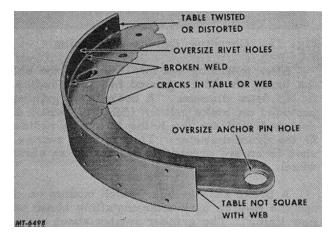
Figure 8 Defects to be looked for on Brake Shoe
