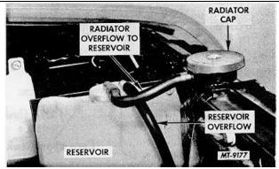
Fig. 2 Coolant System Reservoir Installation
