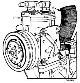
Fig. 18 Removing Freon Compressor Idler Pulley Bracket
