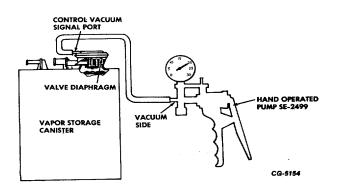
Fig. 15 Canister Fuel Bowl Vent Control Valve Diaphragm Test
