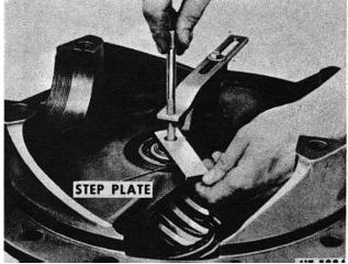
Fig. 14 Installing Step Plate
