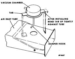
Fig. 11 Vacuum Chamber Replacement
