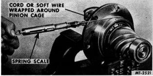
Fig. 11 Measuring Pinion Bearing Preload
