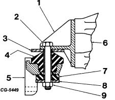
Fig. 7 Engine Rear Mounting with Two-Piece Insulator
