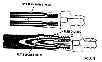
Fig. 1. Flexible Hose Damage
