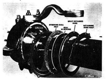
Fig. 21 Trunnion Housing Seals and Retainers
