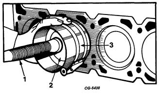
Fig. 146 Installation of Piston in Cylinder Block
