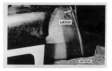
To remove the engine cover (in cab), pull outward on the cover latches.
