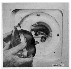
Fig. 7 Removing Headlight Assembly
