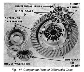
When reinstalling ring gear, it is suggested that Riveting Fixture SE-2222 be used. This special tool is designed for use with either hydraulic or mechanical press equipment. Rivet pressures for
