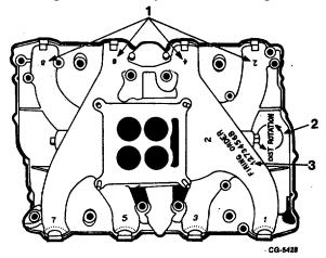
Fig. 135 Illustration of Information Contained on Intake Manifold
