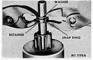
Fig. 11 Installation of Retainer And Thrust Collar
