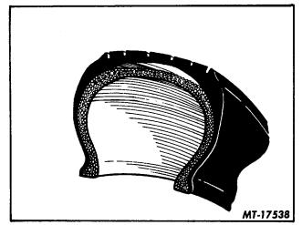
Fig. 18 Tread Separation Result of Underinflation, Overloading, or High Speed
