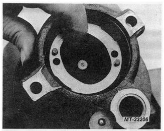
Fig. 27 Install Pump Ring
