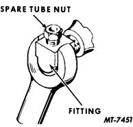
Fig. 3. Protecting Fitting Against Damage During Removal or Installation
