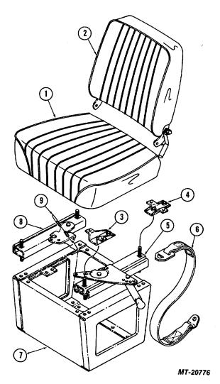
Fig. 29. Individual Drivers Seat Custom Trim Exploded View
