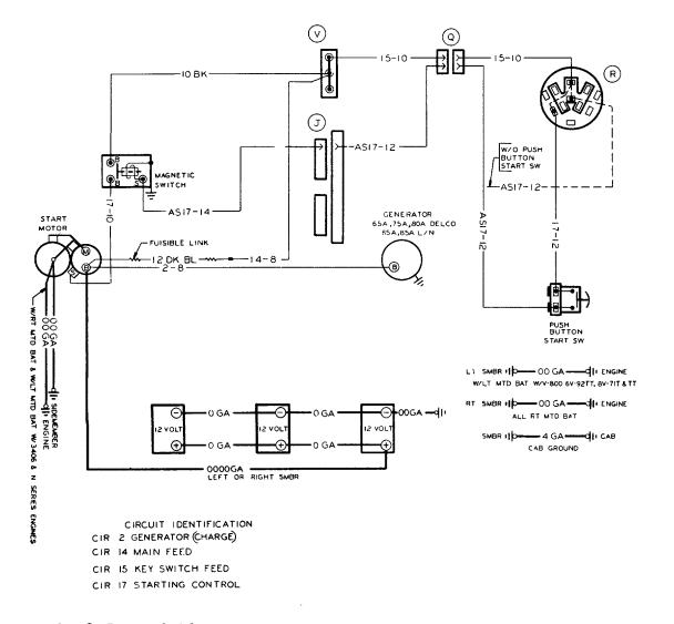
6V-92TT.8V-7IT&TT.800,3406&N-SERIES STARTING, CHARGING & MAJOR FEED & GROUND WIRING MT-21971
