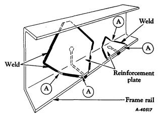
Fig. 5-Suggested Types of Reinforcing Plates and Method of Attaching to Frame Rail.
