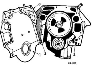
Fig. 51 Removal of Engine Front Cover
