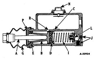
Fig. 1. Typical Master Cylinder
