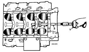
Fig. 80 Removing Second Bearing
