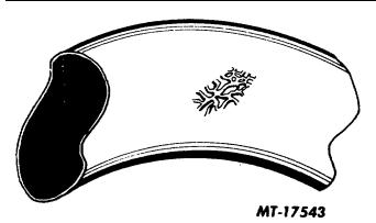
Fig. 21 Damage Caused by Not Removing Label
