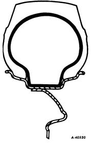
Fig. 1. Drop Center Type Disc Wheel (with Tube)
