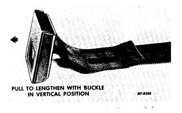
Always pull the belt completely out of the retractor before adjusting and fastening the other half of the belt unit.
