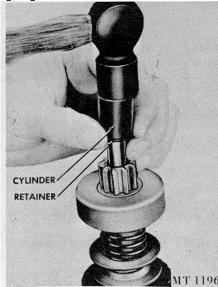
Fig. 7 Removing Retainer from Snap Ring
