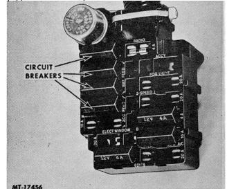
Figure 3 Fuse Panel with Fuse Replacement Type Circuit Breakers Installed
