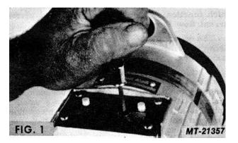
If the voltage is excessively high and cannot be lowered by means of the adjustment, the regulator is probably defective and should be replaced. If the output voltage cannot be raised, either the alternator, regulator or diode trio may be at fault. To determine if the fault is in the regulator or in the alternator, perform the following test.
