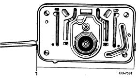
1. Idle Adjusting Screws Figure 50 Secondary Metering Block
