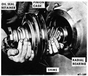
Fig. 16 Removing Pinion and Cage Assembly
