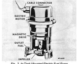
Fig. 2 In-Tank Mounted Electric Fuel Pump
