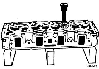
Figure 116 Using Gauge from SE-1631 Tool Grinder Set for Checking Seat Run-Out
