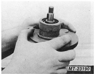
Fig. 11 Separate Rotating Group From Housing
