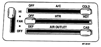
Fig. 22 Air Conditioning Controls Set for Maximum Cooling
