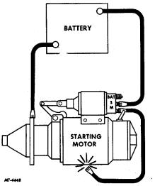
Fig. 12 Pinion Drive Clearance Check Hookup
