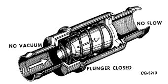
Fig. 48 Plunger Position During Backfire or When Engine is "OFF".
