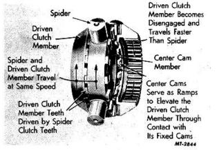
Fig. 41 Forward Left-Hand Turn (Cross Sectional View)
