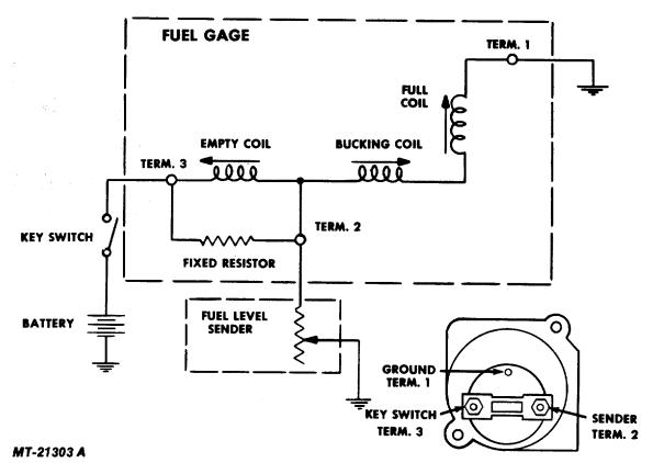
Fig. 17 Fuel Gauge Circuit Diagram
