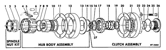
Fig. 1. Locking Hub (Automatic)
