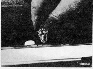
Fig. 13 Removing Bulb and Bulb Socket from Cluster
