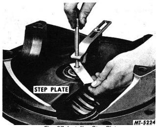
Fig. 27 Installing Step Plate
