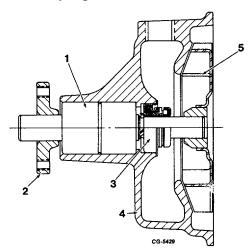
Fig. 137 Section View of Water Pump Assembly
