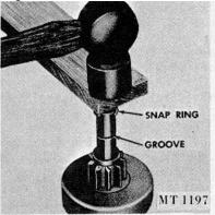
Fig. 10 Installing Snap Ring
