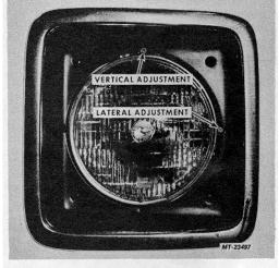
Fig. 2 Headlight Adjusting Screws
