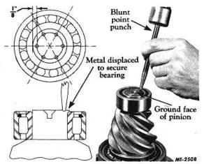
Fig. 24 Staking Pinion Straddle Bearing ESTABLISH NOMINAL DIMENSION
