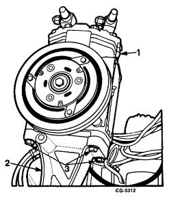
Fig. 19 Freon Compressor Removal
