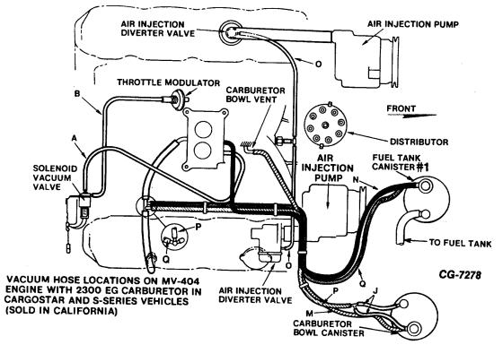
Fig. 84 Vacuum Hose Locations on MV-404 Engine With 2300 EG Carburetor in Cargostar and S-Series Vehicles With Two Vapor Storage Canisters (Sold in California)
