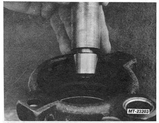
Fig. 24. Install New Needle Bearing,
