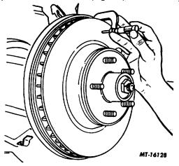
Fig. 18 Checking Rotor with Micrometer
