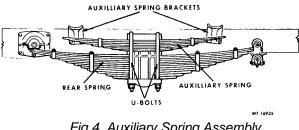
Fig.4 Auxiliary Spring Assembly
