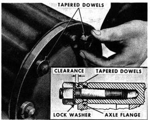
Fig. 7 Details of Taper Dowels
