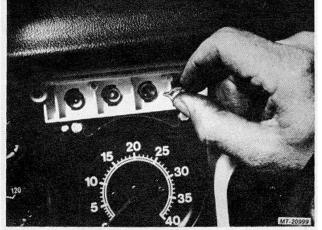
*Fig.* 12 *Removing Bulb from Face of Cluster* 3. Insert new bulb into socket.
