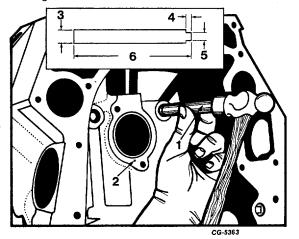
Fig. 70 Tappet Oil Gallery Plug Installation
