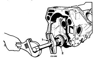
Fig. 67 Using SE-1368 Puller to Remove Crankshaft Gear
