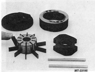
Fig. 16 Remove Vanes From Rotor
