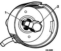
Fig. 25 Bushing Remover SE-1955-5 Installed in Upper Bushing 1. Upper Bushing 2. Remover
