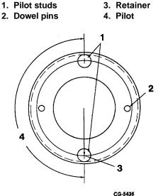
Fig. 144 Dimensions for Rework of SE-1942-2 Pilot
