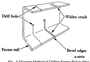
Fig. 4-Showing Method of Drilling Frame Rail to Stop Progress of Crack. Also shows Method of Preparing Crack for Welding.
