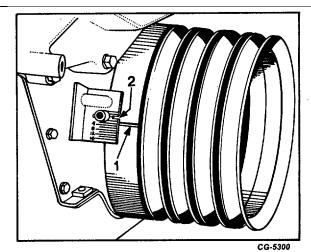
Fig. 4 Illustrating Timing Marks on Crankshaft Pulley Hub and Engine Front Cover
