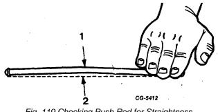
Fig. 119 Checking Push Rod for Straightness
