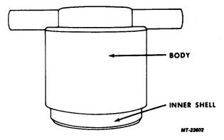
Fig. 4. Air Cleaner Assembly (Replaceable Element Type)
