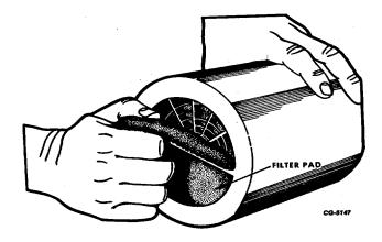
Fig. 8 Vapor Storage Canister Air Filter Location
