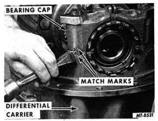
Fig. 10 Marking Bearing Cap for Identity
