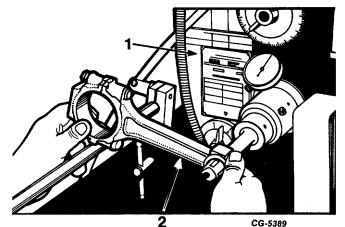
Fig. 96 Honing Connecting Rod Bushing Using SE-2218 Equipment
