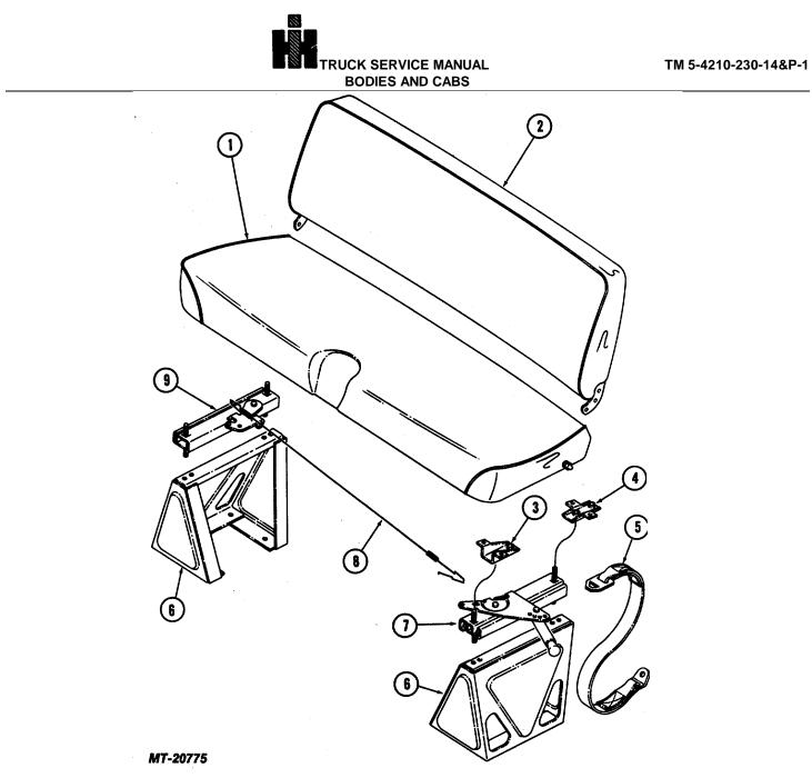
Fig. 28. Full Width Bench Seat - Standard Trim - Exploded View
