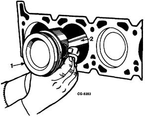
Fig. 60 Connecting Rod and Piston Removal
