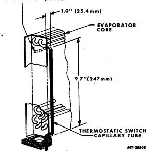
Fig. 59 Capillary Tube Location in Evaporator
