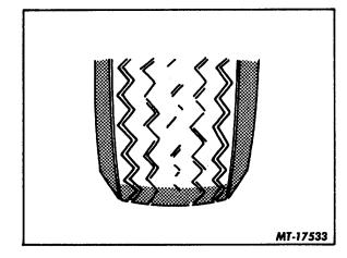
Fig. 13 Overinflation, Excessive Wear in Center of Tread
