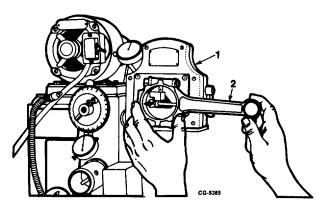
Fig. 92 Checking Connecting Rod Bore Using Precision Gauge Furnished with Honing Machine SE-2218
