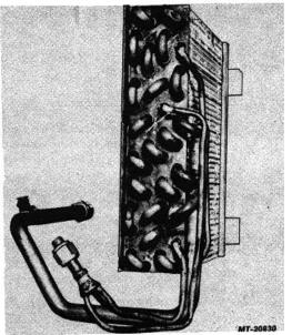
Fig. 11 Evaporator Core
