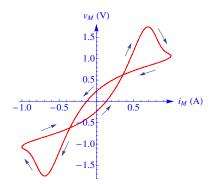
Fig. 7. Mathematica  $v_M - i_M$  for capacitor in parallel with memristor (discharge tube). A parasitic capacitance of 1 F was used, memristor parameters are the same as in Fig. 5.
