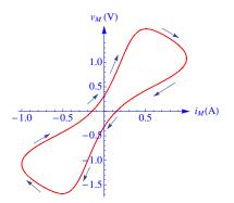
Fig. 6. Mathematica  $v_M - i_M$  for inductor in series with memristor (discharge tube). A parasitic inductance of 5 H was used, memristor parameters are the same as in Fig. 5.
