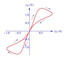
Fig. 5. Theoretical  $v_M - i_M$  memristor (discharge tube) Lissajous figure from Mathematica. Parameters used for simulation were  $\beta = 0.1, \alpha = 0.1, F = 1, \omega = 0.063$ .
