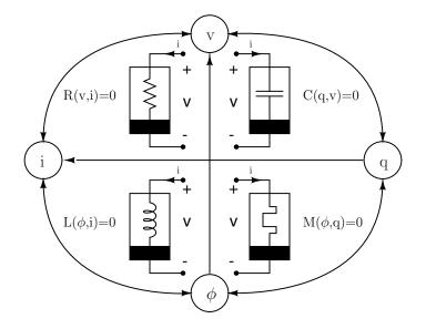
Fig. 1. The four fundamental 2-terminal circuit elements relate the fundamental circuit variables [5]. Note that current is defined as the rate of flow of charge  $(i = \dot{q})$ . Voltage is defined as the rate of change of flux-linkage  $(v = \frac{d\phi}{dt})$ . Flux-linkage is the number of magnetic field lines passing through a given cross-sectional area.
