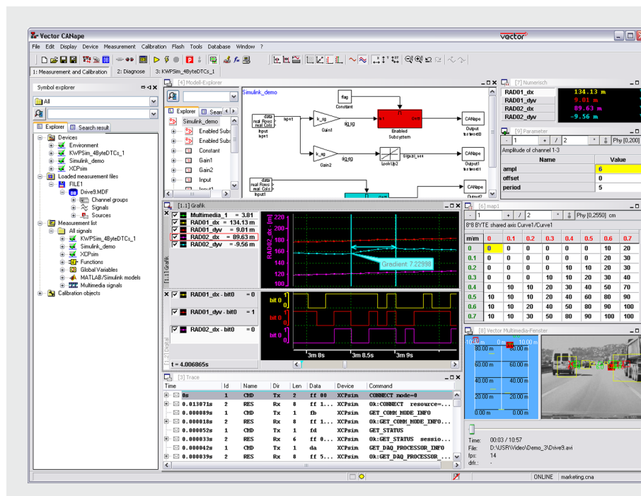
Figure 1: Time-synchronous real-time acquisition and visualization of internal ECU signals via CCP/XCP, and of signals from CAN, LIN and FlexRay buses and external measurement equipment via CANape.
