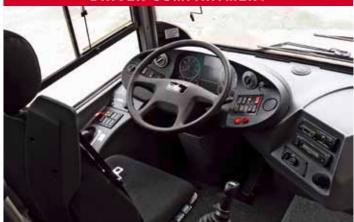
Multi adjustable driver's seat with pneumatic suspension, integrated headrest and 3-point safety belt with pretensioner
