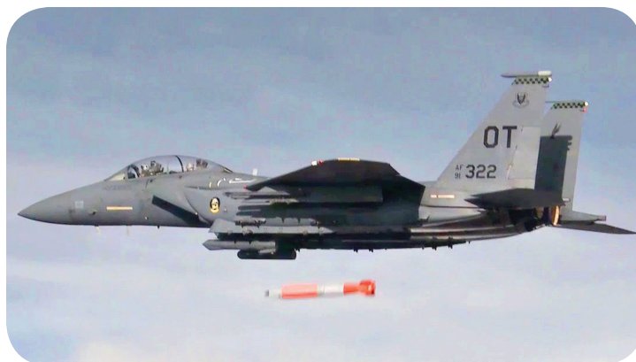
An F-15E drops a B61-12 test unit during a development flight test.
