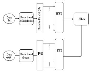
Fig.(2) Block diagram of OFDM system
