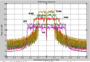
Fig.(3)OFDM Spectrum with different modulation
