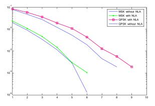
Figure (7-a) effect of NLA on MSK & QPSK As regarding to our previous results, it can be noticed that, the MSK modulation gives us the lowest PAR when used in OFDM besides its main advantage, that it ignores any fading introduced amplitude fluctuation present in the received signal,
