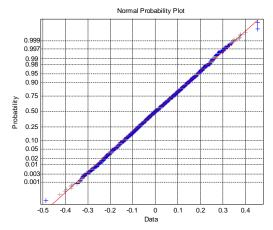
Fig.(1) Normal probability plot of OFDM signal
