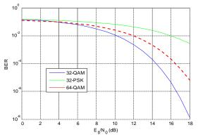
Fig.(5-b) BER of OFDM using 32,64 -PSK&QAM Regarding to the BER performance of the used modulation techniques, it is clear from figure (5-a) and (5-b) that, for M-PSK and M-QAM, the BER increases ad M increase while for the same M the BER of M-PSK is larger than that of M-QAM for the same  $E_b/N_{o}$ .
