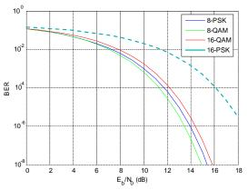
Fig.(5-a)BER of OFDM using 8,16 -PSK&QAM
