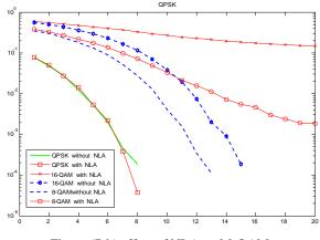
Figure (7-b) effect of NLA on M-QAM
