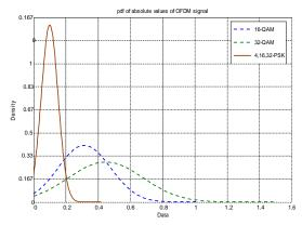
Fig.(4) PDF of OFDM with different modulation
