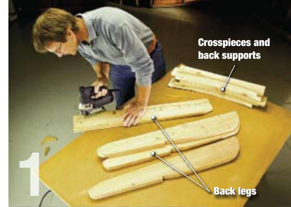
Cut the legs, crosspieces and back supports. Make one of each part based on the illustration; then use that piece as a pattern for the other parts.
