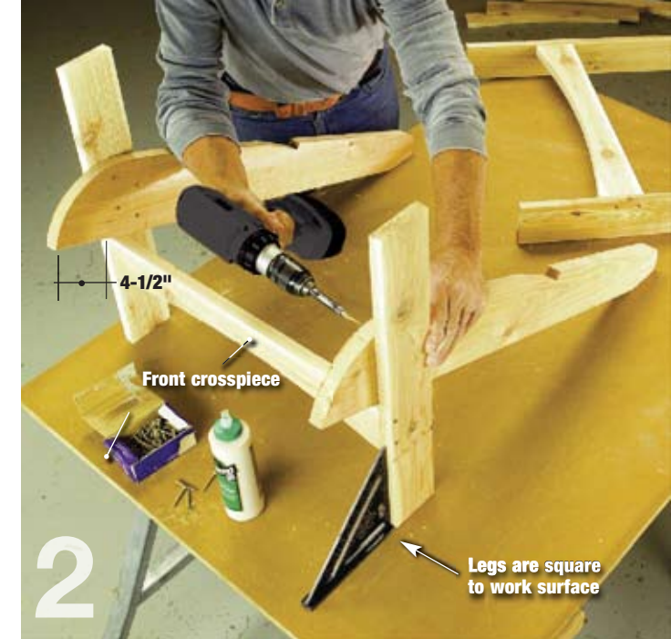
Assemble each base with exterior-rated glue and deck screws. Keep the front legs square to the ground or work surface.
