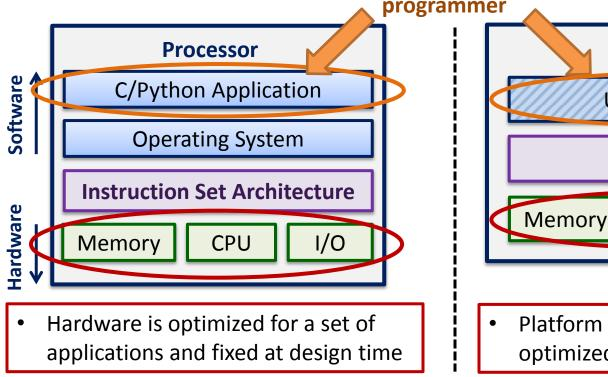
Platform hardware can be optimized for the target application
