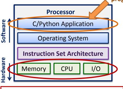
Hardware is optimized for a set of applications and fixed at design time
