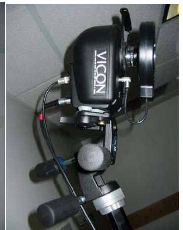
Vicon cameras with ring of infrared LEDs
