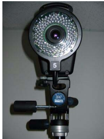
Vicon cameras with ring of infrared LEDs
