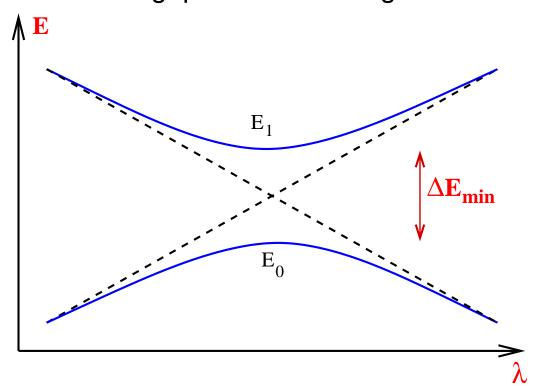
The dashed lines show a crossing that the ground state and first excited would have in the absence of any coupling between them. However, there is actually "level repulsion" so the two levels, shown by the solid lines, do not cross but have a minimum gap  $\Delta E_{min}$ .
