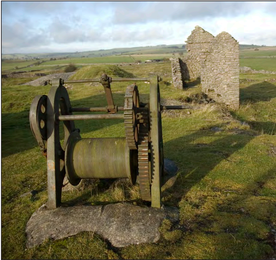
Plate 3: Site 129: One of the crab winches at Magpie Mine (Site 129), with the dressing engine house behind, both at the heart of the Scheduled Monument and cared for by the Peak District Mines Historical Society for several generations.
