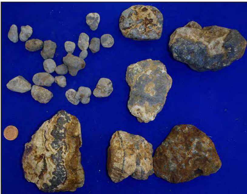
Plate 10: Lumps of detrital galena from Speedwell Cavern. The larger pieces are typical pieces of barite/galena ore. These are probably representative of lead ore found in some of the easily worked sedimentary deposits containing derived galena that have been worked in most parts of the Peak District and led to short term high outputs. 1p coin for scale.
