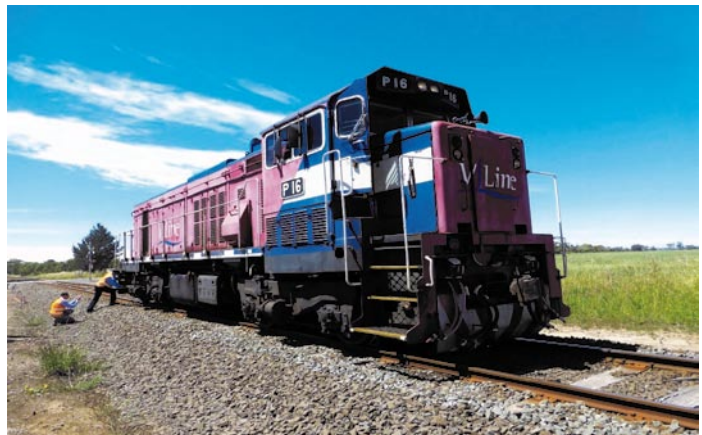
Figure 15 - Class “P” Bo-Bo Diesel/Electric Loco
