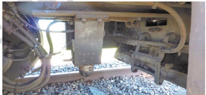
Figure16 - View of the TPWS aerial under the “P” Class loco
