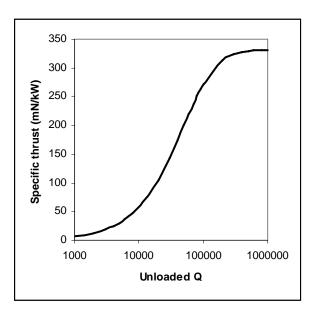
Fig 4.2 Specific thrust at 3km/s.
