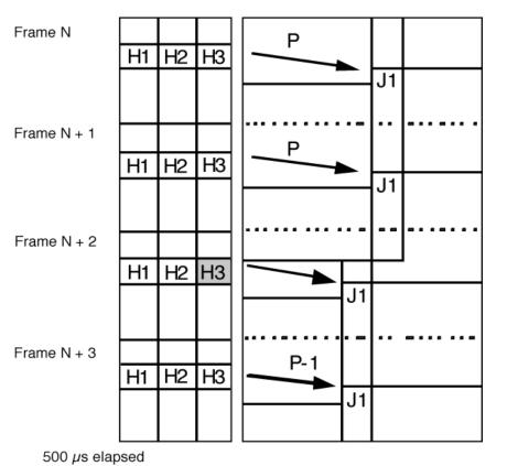
The SPE moves forward in time when a data byte has been stuffed into the H3 byte.
