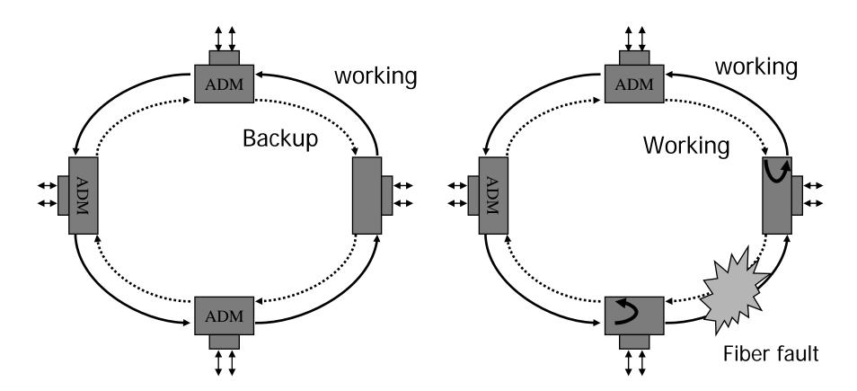
Only nodes close to the fault are involved in the protection
