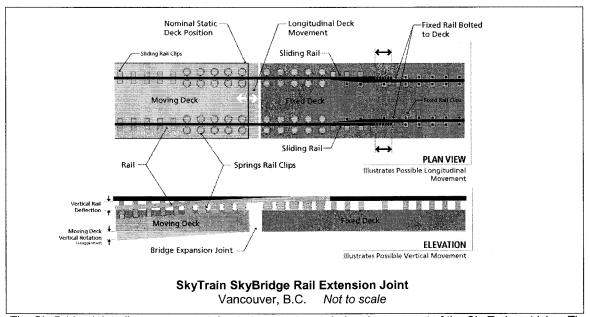
The SkyBridge joint allows movement due to temperature, wind and movement of the SkyTrain vehicles. The rail joint undergoes vertical and horizontal angular changes and longitudinal movement. The rail joint consists of two parts: a pair of sliding sections that allow for longitudal movement (top), and another section with spring devices that allow for vertical angular change (bottom).
