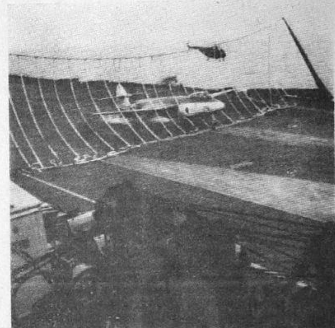
THESE TWO PICTURES show a modern crash barrier in action. This barrier is a nylon webbing. Note the helicopter, standing by.
