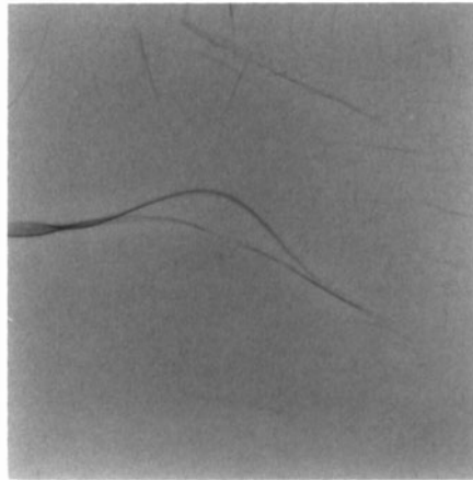
Fig. 6: Low-kV contact radiographic image of the 23 mm thick tile.
