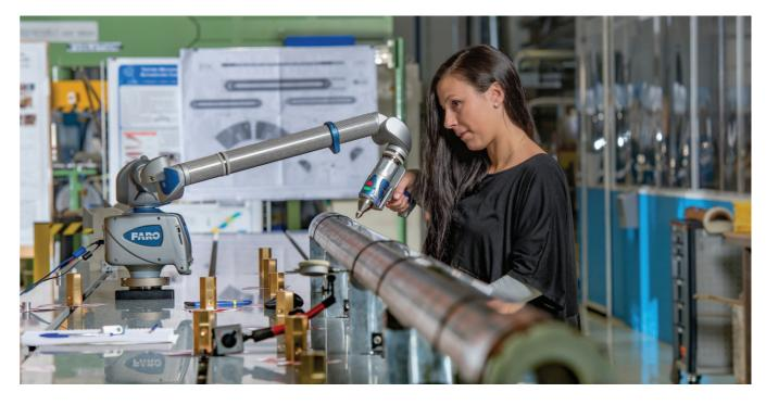
A scientist carefully checks the geometry of a dipole magnet coil for the High-Luminosity LHC. (OPEN-PHO-ACCEL-2017-010-1)
