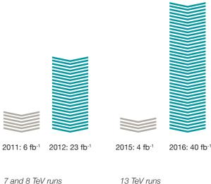
Above, the amount of data delivered by the LHC to the ATLAS and CMS experiments over the course of its proton runs. These quantities are expressed in terms of integrated luminosity, which refers to the number of potential collisions during a given period.
