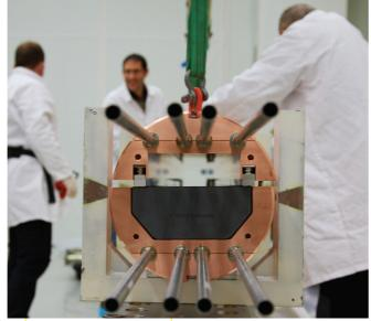
A new SPS beam dump was designed and built in just a few months for installation in the accelerator during the extended yearend technical stop. (CERN-PHO-201704-084-15)
