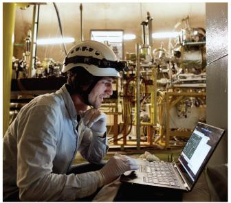
Member of the AWAKE collaboration performing tests in the experiment's underground tunnel. AWAKE explores the use of plasma to accelerate particles. (CERN-PHOTO-201612-314-9)
