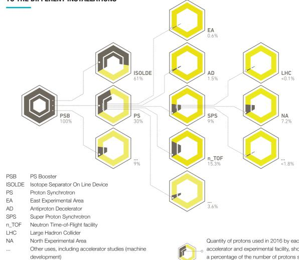
1.34 x 10<sup>20</sup> protons were accelerated in the accelerator complex in 2016. This might sound like a huge number, but in reality it corresponds to a minuscule quantity of matter, roughly equivalent to the number of protons in a grain of sand. In fact, protons are so small that this amount is enough to supply all the experiments. The LHC uses only a tiny portion of these protons, less than 0.1%, as shown in the diagram.
