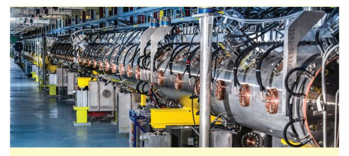
View of the new 86-metre-long Linac4 accelerator. In 2016, Linac4 was completed and reached its design energy of 160 MeV. It will become the first link of the LHC accelerator chain after 2020. (OPEN-PHO-ACCEL-2017-011-3)
