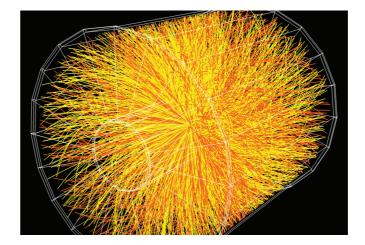
The outcome of a high-energy lead-lead collision recorded by the ALICE detector, in which a total of 3161 charged particles were detected. (ALICE-PHO-GEN-2016-001-3)
