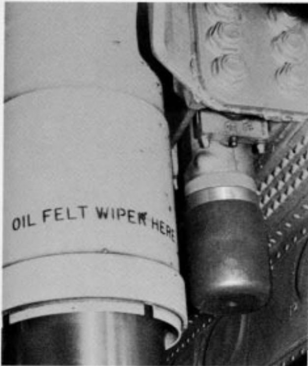
Figure 2. Main landing gear splash guard installed.
