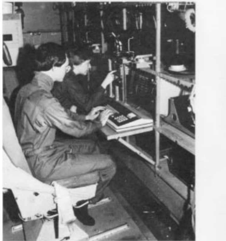
With the LADS, test data is available for study almost immediately after a data point is flown.
